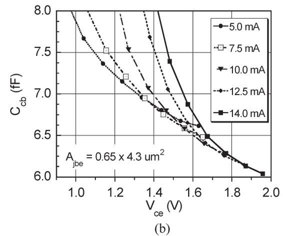
Fig. 4. Variation of  $C_{cb}$  with  $V_{cb}$  at  $I_c = 0 \text{ mA}$  for (a) a mesa HBT and the pedestal HBT (b) and variation of  $C_{cb}$  with  $V_{ce}$  at different  $I_c$  to show the effect of high-series collector resistance. Junction areas as well as the emitter, base, and drift collector layer structures of the two HBTs are identical.
