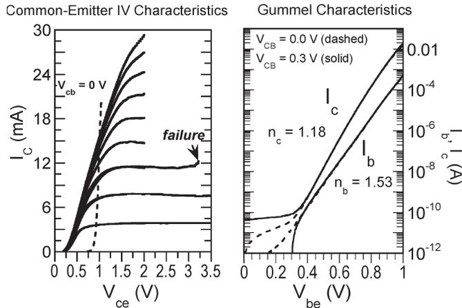
Fig. 2. Common-emitter  $I$ - $V$  characteristics ( $I_{b,step} = 100 \mu\text{A}$ ) and Gummel characteristics. Emitter junction dimension  $A_{je} = 0.6 \times 4.3 \mu\text{m}^2$ .
