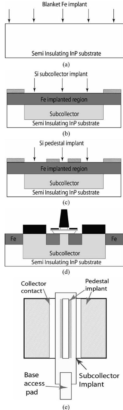
Fig. 1. Pedestal/subcollector process cross section—(a) blanket surface Fe implant to suppress interface states and form the extrinsic collector depletion regions, (b) deep Si implant to form the subcollector, (c) Si pedestal implant to electrically link the N $^-$  drift collector and collector contacts to the subcollector, (d) active HBT layers are then grown and device formation ensues, and (e) top view of the device showing the pedestal (hatched lines) and subcollector implants.
