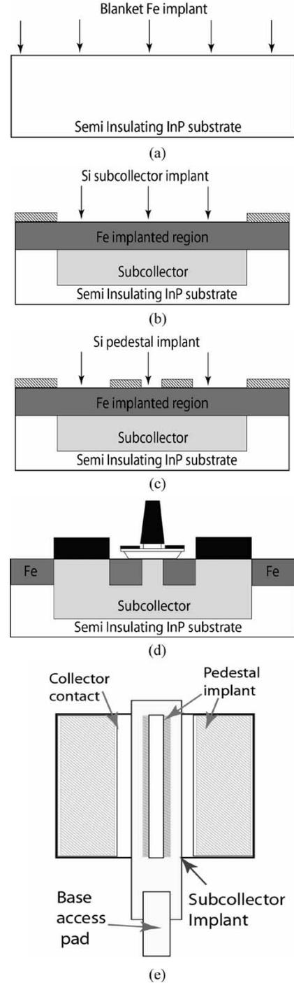
Fig. 1. Pedestal/subcollector process cross section—(a) blanket surface Fe implant to suppress interface states and form the extrinsic collector depletion regions, (b) deep Si implant to form the subcollector, (c) Si pedestal implant to electrically link the N<sup>-</sup> drift collector and collector contacts to the subcollector, (d) active HBT layers are then grown and device formation ensues, and (e) top view of the device showing the pedestal (hatched lines) and subcollector implants.
