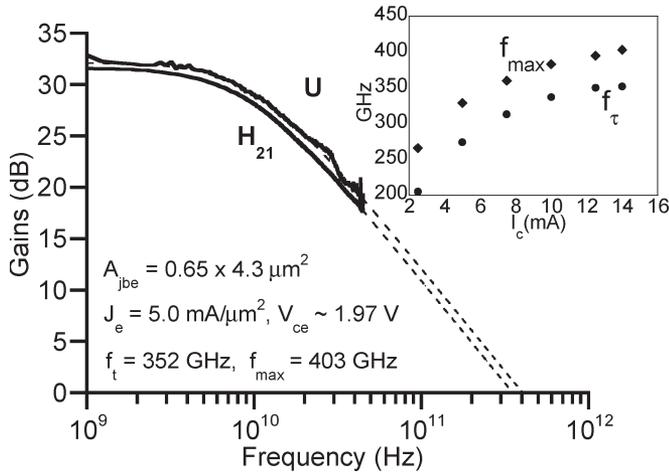
Fig. 3. Measured microwave gains  $H_{21}$  and Mason's unilateral power gain  $U$  at a bias associated with peak  $f_\tau$  and  $f_{max}$ . Figure inset  $-f_\tau$  and  $f_{max}$  versus  $I_c$ .
