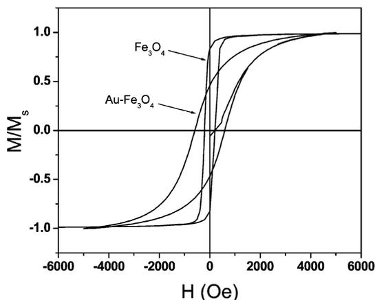
**Figure 7.** Magnetization hysteresis loops measured at 10 K, for assemblies of 10 nm Fe<sub>3</sub>O<sub>4</sub> nanoparticles and spherical Au–Fe<sub>3</sub>O<sub>4</sub> core–shell hybrid nanoparticles with 3 nm Au cores and 10 nm total diameter.
