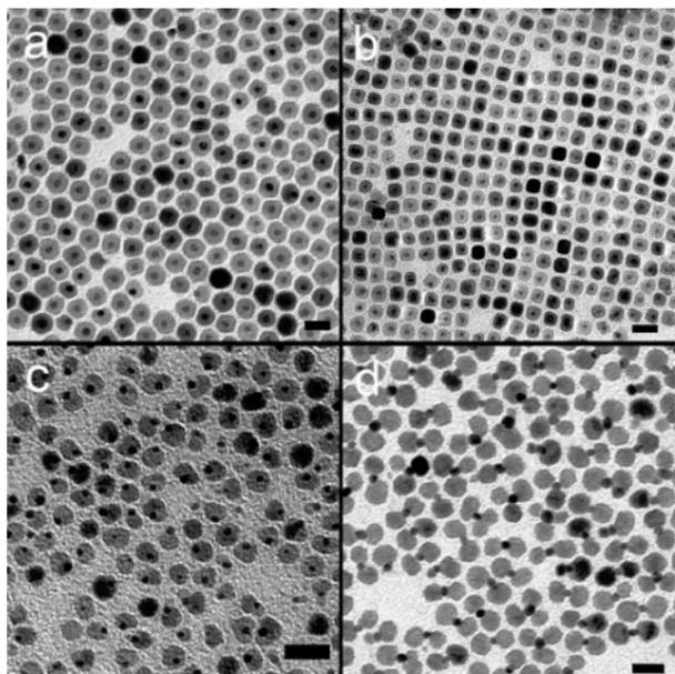
**Figure 1.** TEM images of spherical (a), cubic (b), peanutlike (c), and dumbbell-like (d) Au–Fe<sub>3</sub>O<sub>4</sub> hybrid nanoparticles. The scale bars are 20 nm.
