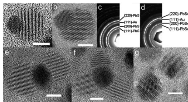
**Figure 4.** HRTEM images of 3 nm Au–6 nm PbS (a), 5 nm Au–8 nm PbS (b), Au–PbS dumbbell (e) Au–PbS tripod (f), and Au–PbSe core–shell (g) hybrid nanoparticles. Typical electron diffraction patterns from Au–PbS (c) and Au–PbSe (d) structures. The scale bars are 4 nm.
