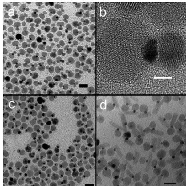
**Figure 5.** TEM images (a, c, and d) and HRTEM image (b) of Fe<sub>3</sub>O<sub>4</sub>–Au–PbSe (a and b) and Fe<sub>3</sub>O<sub>4</sub>–Au–PbS (c and d) ternary hybrid nanoparticles. The scale bars are 20 nm in a, c, and d and 4 nm in b.
