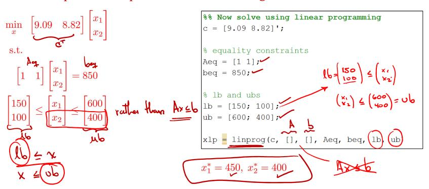
Let's consider two generation units with **linear costs** feeding a load of 850 MW
