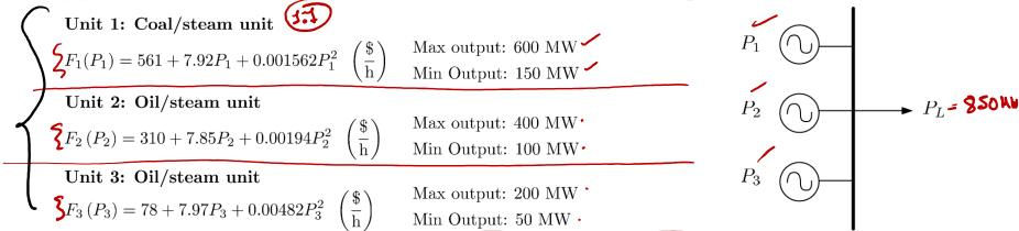
The three generators feed a load of  $P_L = 850 \text{ MW}$ . What is the power level of each generator to minimize the cost of operation?
