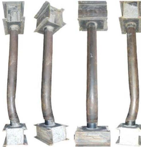
Figure 11: Plastic Deformation of CFST under Blast
