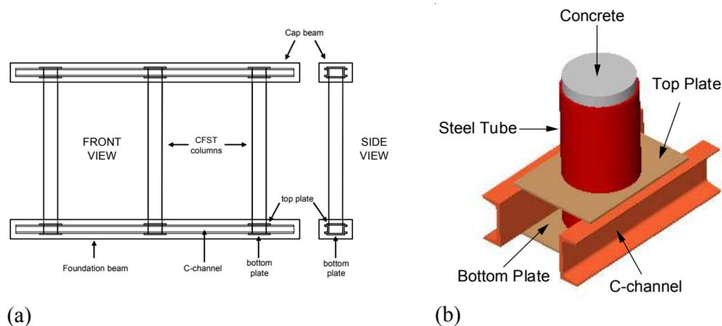
Figure 3: Multi-column pier-bent made up of CFST columns: (a) General description; (b) Details of column-to-foundation beam connection
