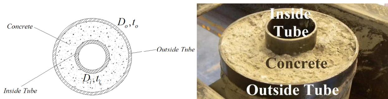
Figure 9: Concrete Filled Double Skin Tube
