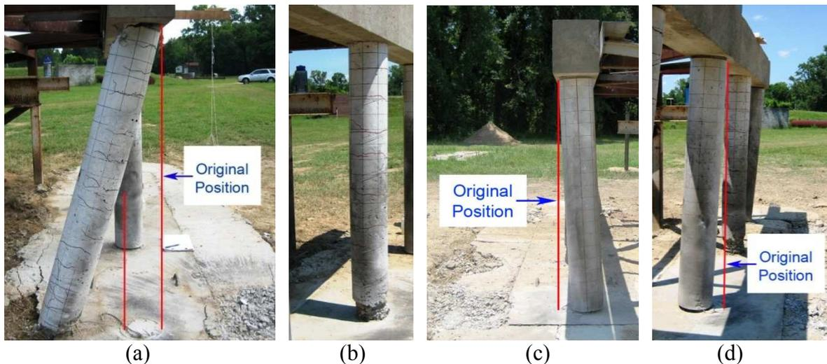
Figure 7: Columns after tests: (a) side view of Column RC1, Test 1 (b) front view of Column RC2, Test 2 (c) side view of Column SJ2, Test 3 (d) side view of Column SJ1, Test 4
