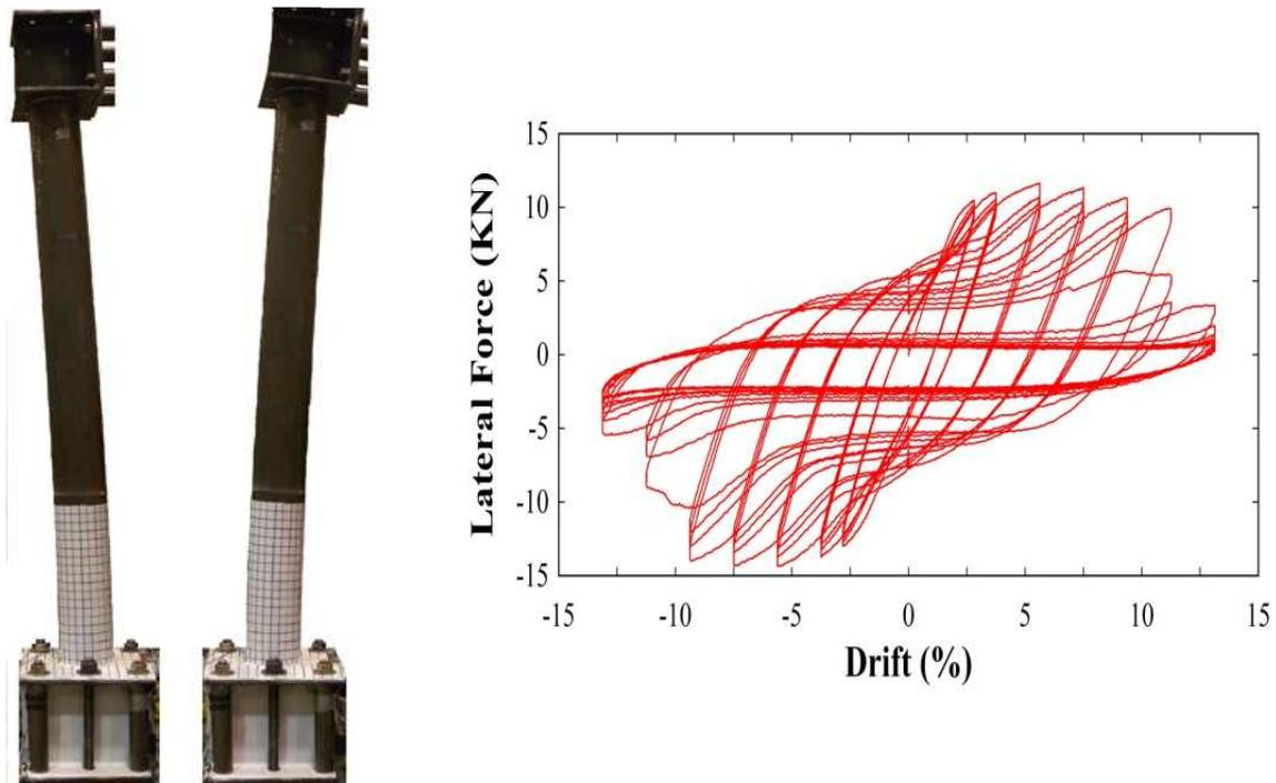
Figure 13: Specimen at Maximum Strength (Left) and Typical Hysteretic Loop (Right)
