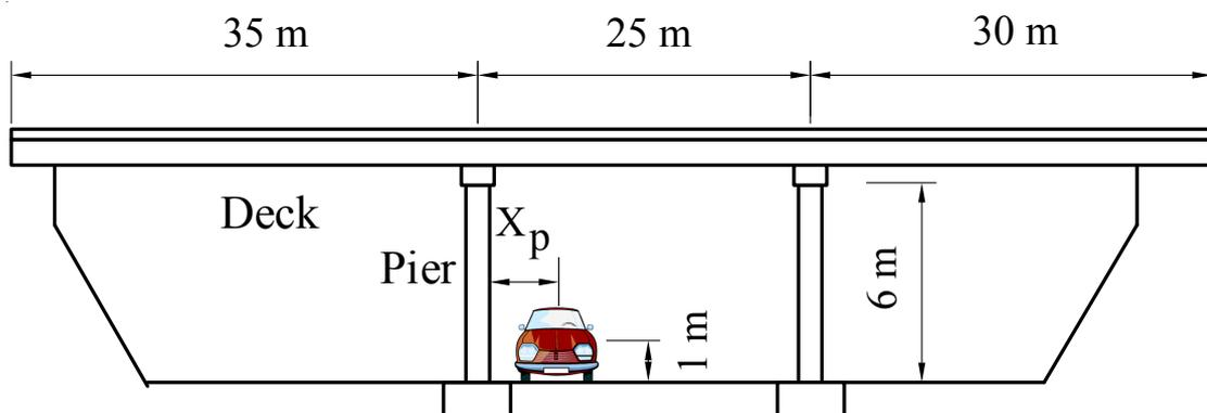
Figure 1: Schematics of prototype bridge and assumed blast scenario
