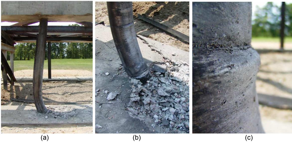
Figure 5: Specimen after extreme blast (charge at credible threat height): (a) column deformation (b) foundation (c) buckling.
