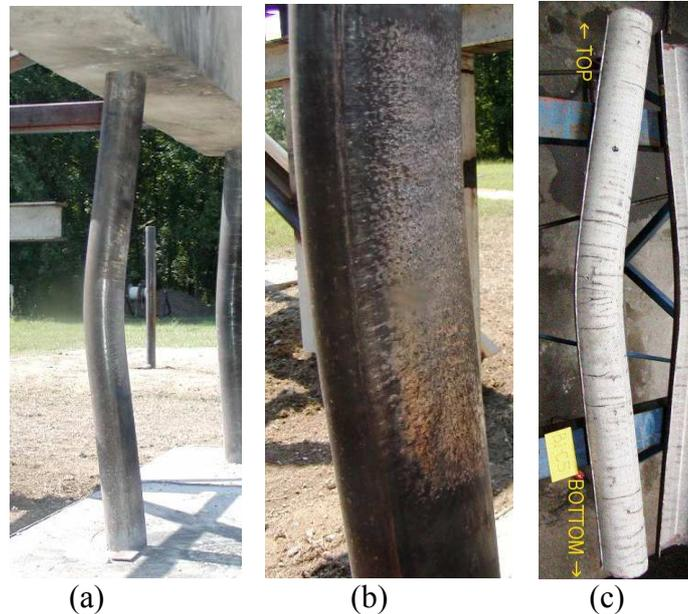
Figure 4: Column subjected to charge at mid-height: (a) column deformation; (b) column surface around mid-height; (c) core concrete
