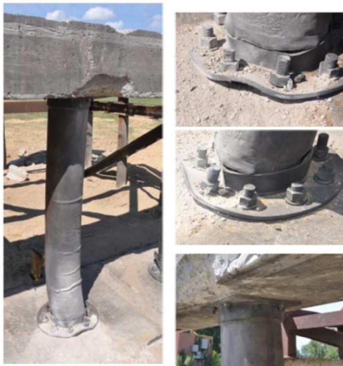
Figure 12: Global (Left) and Local Deformation (Right) of MSJC after Blast Test
