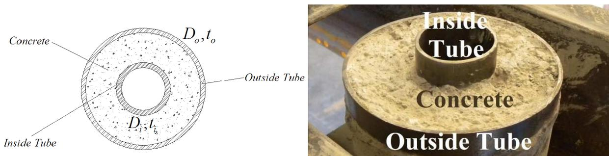
Figure 9: Concrete Filled Double Skin Tube
