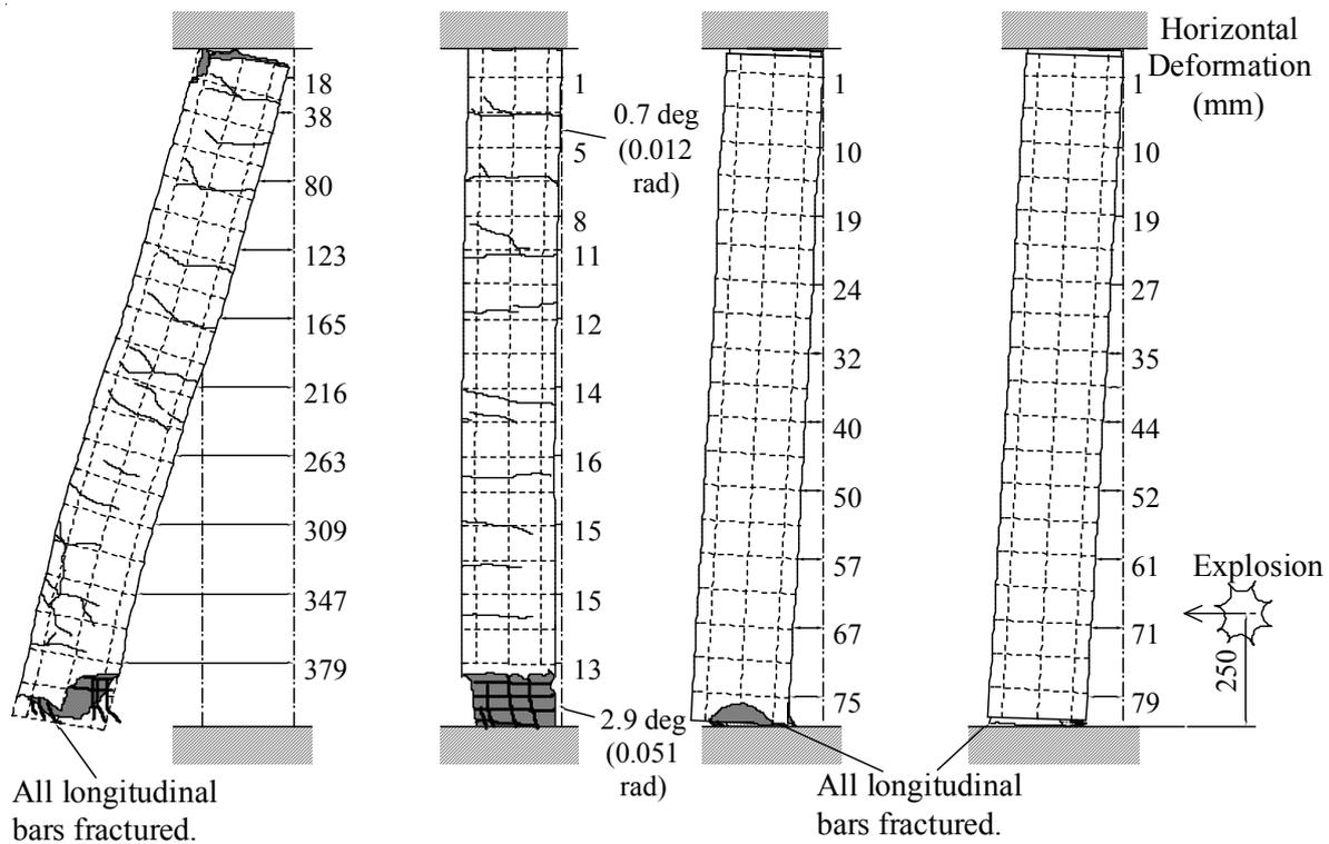
Figure 8: Sketches of columns after tests from side view: Left to right, (a) Column RC1, Test 1 (b) Column RC2, Test 2(c) Column SJ2, Test 3 (d) Column SJ1 Test 4
