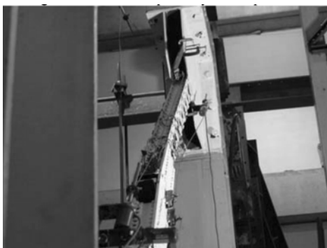
Fig. 15 Out-of-plane buckling of specimen Bx 8-60
