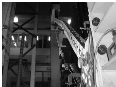
Fig. 16 In-plane buckling of specimen Bx 16-120
