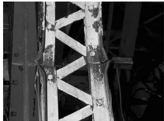
Fig. 10 Fractured shape of specimen Ay 8-120
