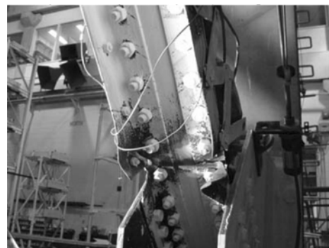
Fig. 14 Fractured shape of specimen By 16-60
