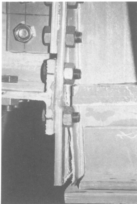
**FIG. 14. Separation of Column's Flange and Web**
