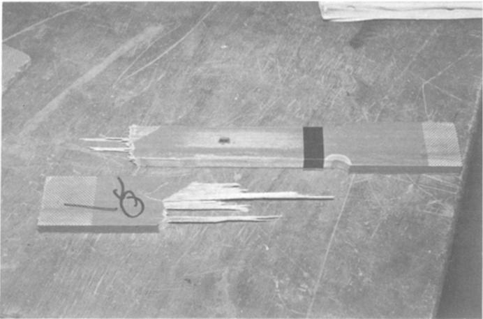
FIG. 1. Failed ASTM E-06 Tension Specimen
