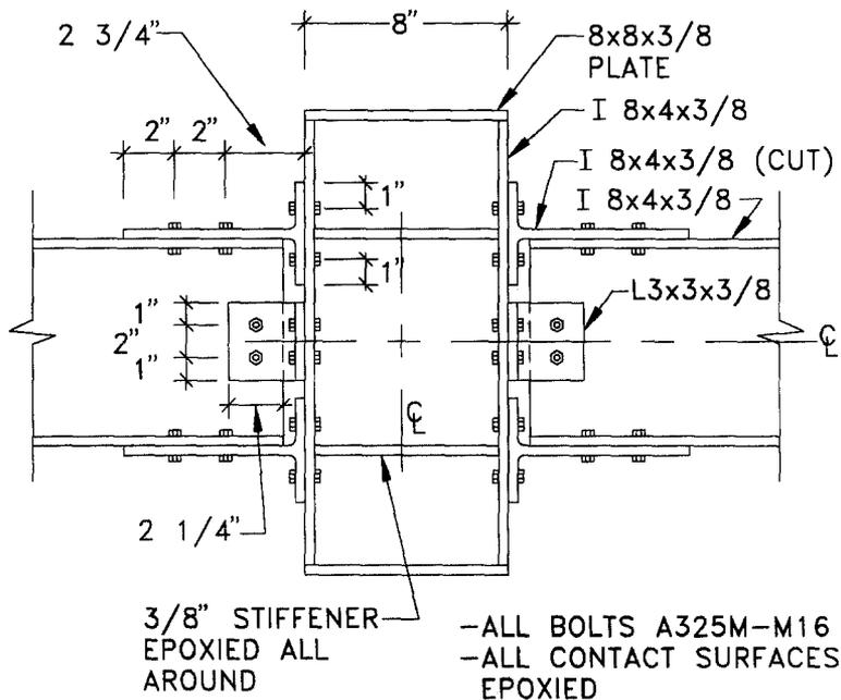
FIG. 8. Details of Tested Rigid Beam-Column Connection
