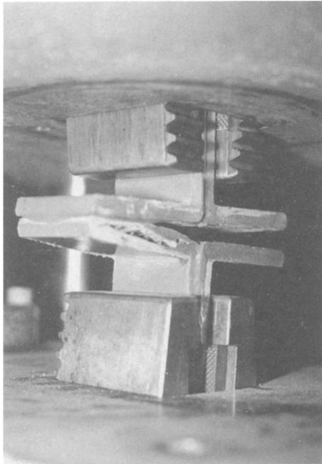
**FIG. 7. Delamination Failure of Epoxied Angles**
