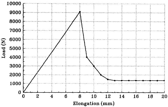
**FIG. 6. Load-Deformation of Epoxy Peel-Test Specimen**
