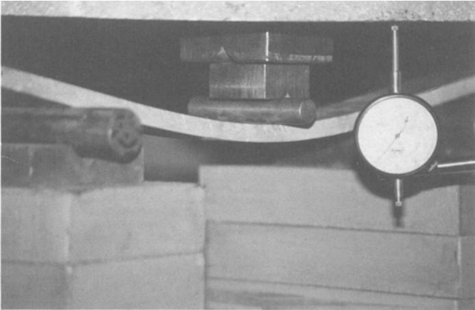
**FIG. 3. Plate's Flexural Deformations near Failure**
