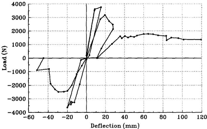
**FIG. 12. Load-Deflection History of Tested Rigid Beam-Column Connection**
