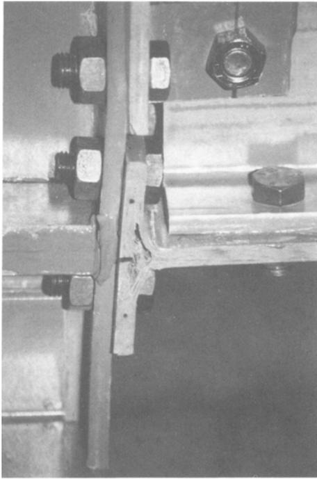
**FIG. 13. Delamination of T-Clip Angle at Flange-Web Core**
