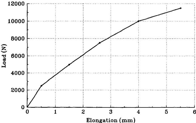
FIG. 4. Stress-Deformation of Epoxy Shear-Test Specimens
