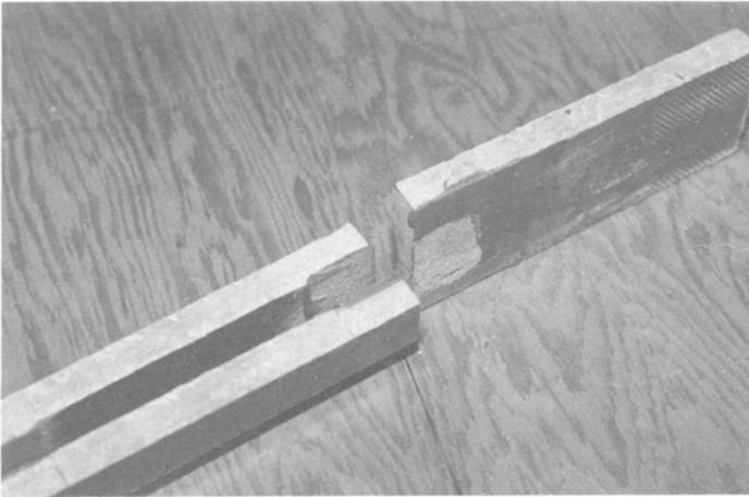
**FIG. 5. Failed Epoxy Shear-Test Specimen**
