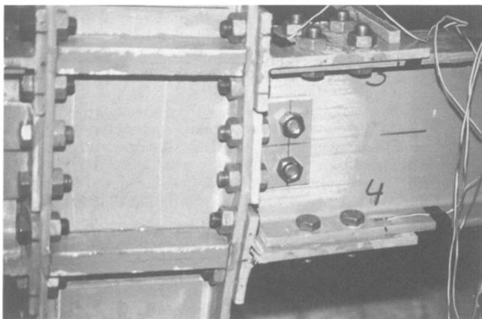
**FIG. 15. Deformations of Specimen near Failure**
