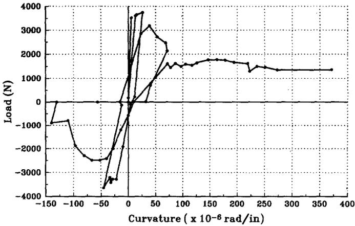
**FIG. 11. Load-Curvature Relationship of Tested Rigid Beam-Column Connection**
