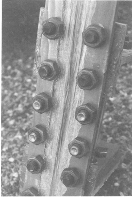
**FIG. 16. Texture of Failure Surface at Separated Web and Flange**
