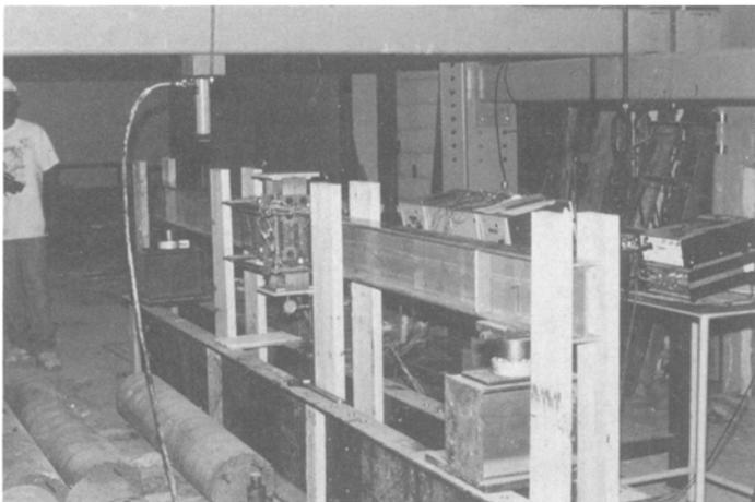
**FIG. 10. Rigid Beam-Column Connection Test Set-up**
