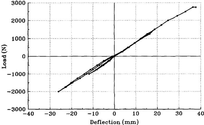
FIG. 2. Load-Deflection Results for Cyclic Plate-Bending Test
