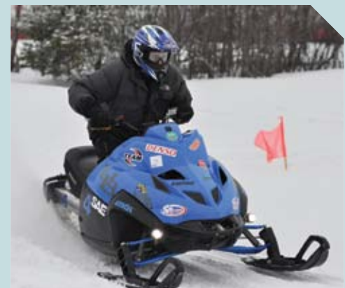
UB SAE's diesel-powered snowmobile performing in the SAE Clean Snowmobile Challenge acceleration and handling events
