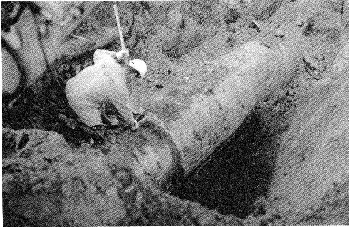
FIGURE 4-25 Compressive Failure of a Welded Slip Joint of the Granada Trunk Line on Balboa Boulevard
