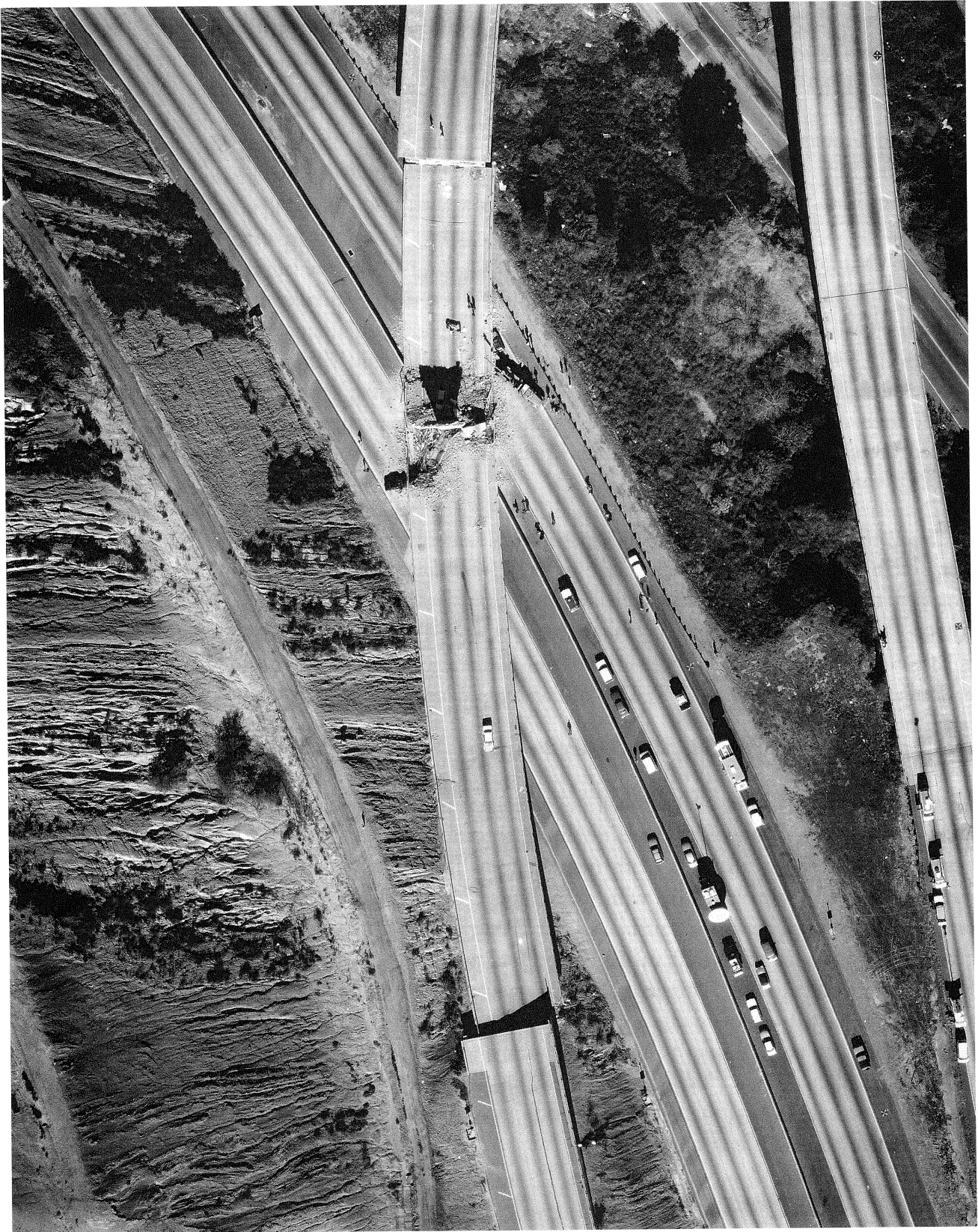
FIGURE 3-5 SR14/I-5 Separation and Overhead (Southbound) - Aerial View of Collapse
