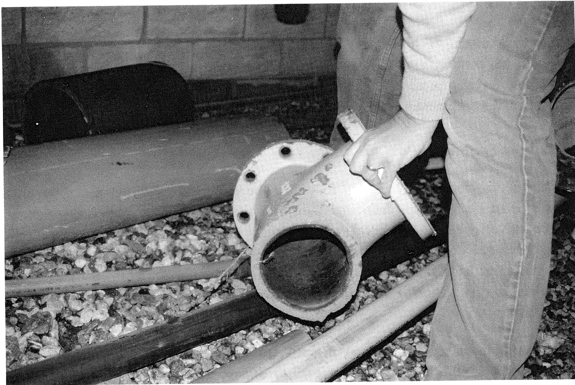
FIGURE 3-54 Process Tank Anchorage Failures Led to Excessive Piping Loads, Resulting in Failures in Flanged Piping
