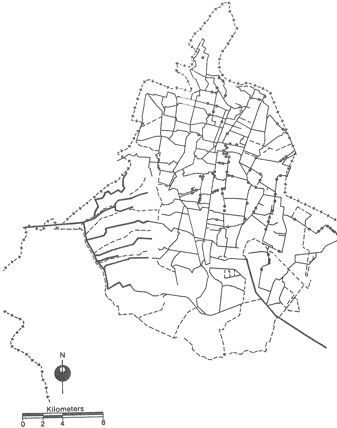
FIGURE 6-14 Well Documented Pipeline Damage In Primary Distribution System Of Federal District - 1985 Michoacan Earthquake
