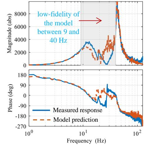
Figure 8.10. Results of acceleration-tracking experiments,  $K_e = 5$  V/in,  $K_p = 0.0002$  V/psi,  $f_c = 80$  Hz,  $\tau_s = 500$   $\mu$ s [2000 Hz]
