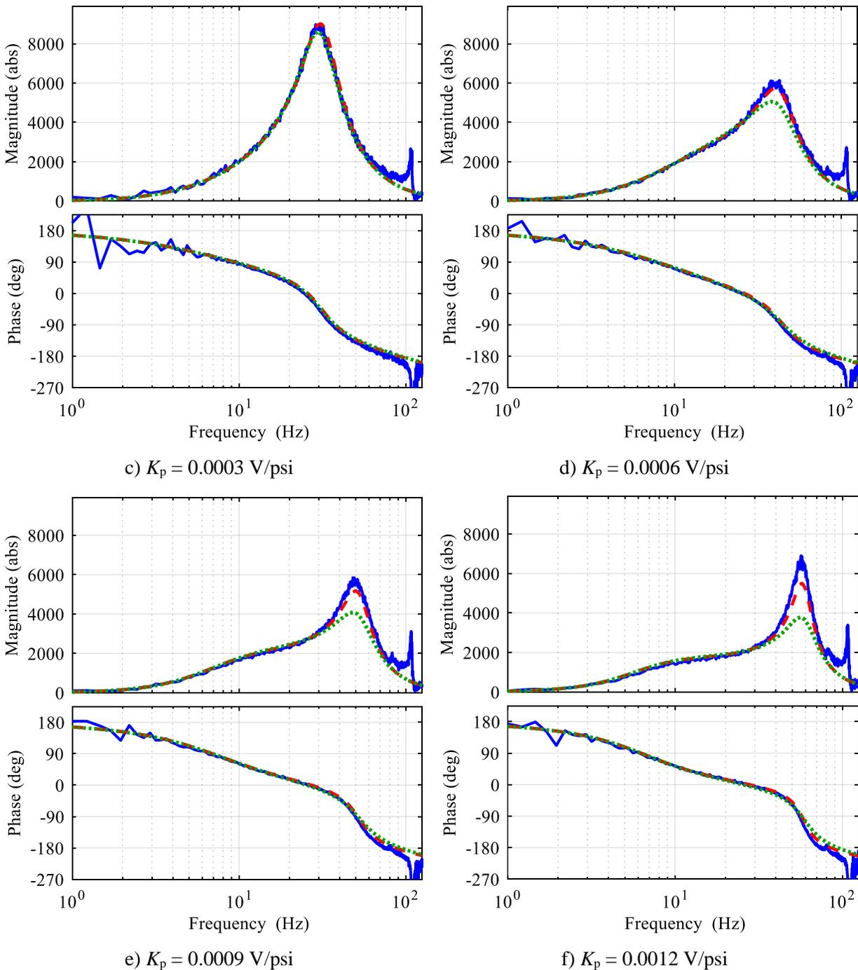
Figure 4-13. Experimental evaluation of the bare shake table for different values of  $K_p$ ;  $K_e = 5$  V/in and  $\tau_s = 500 \mu\text{s}$  [2000 Hz] (cont'd)
