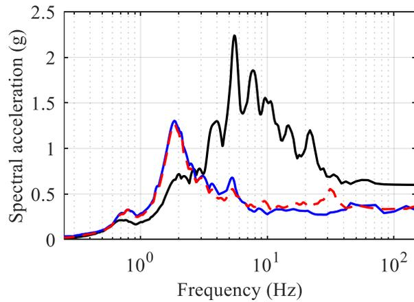
b) 5%-damped acceleration spectra
