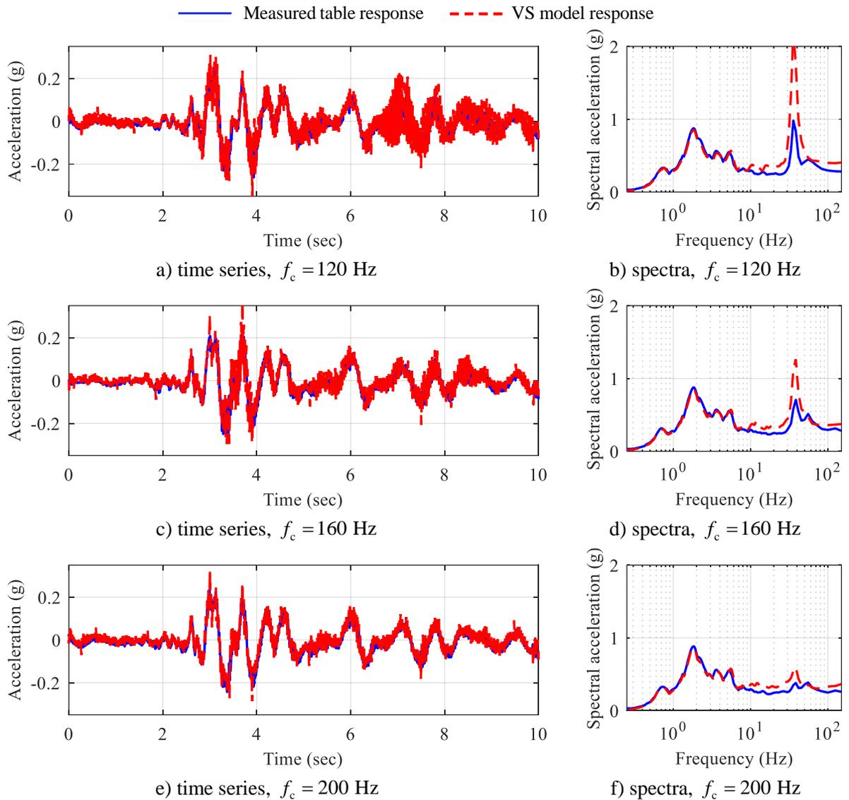
Figure 9.35. Effect of the filter cutoff frequency for imitating  $SD_2$  isolation system subjected to motion  $GM_2$ ,  $m_{vs} = 0.7m_{st}$ ,  $K_e = 5$  V/in,  $K_p = 0.001$  V/psi,  $\tau_s = 500$   $\mu$ s (2000 Hz)
