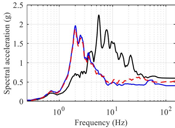
b) 5%-damped acceleration spectra
