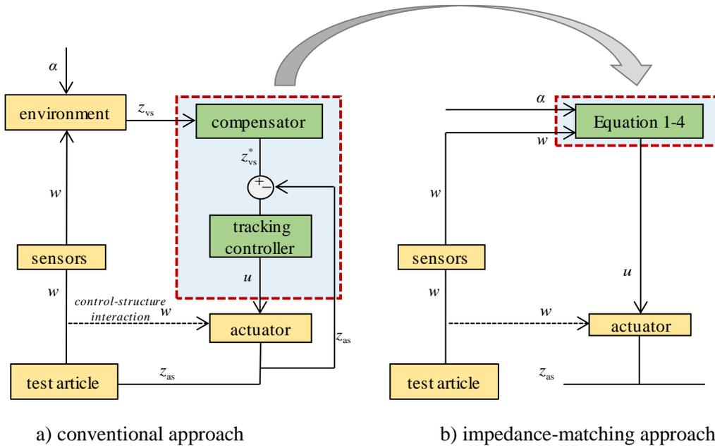
Figure 1.3. Contrasting conventional and the impedance-matching approach to MIL
