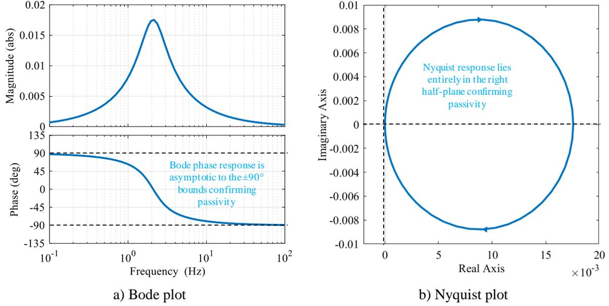
Figure 9.30. Bode and Nyquist plots of the force-velocity transfer function of the  $SD_2$  system
