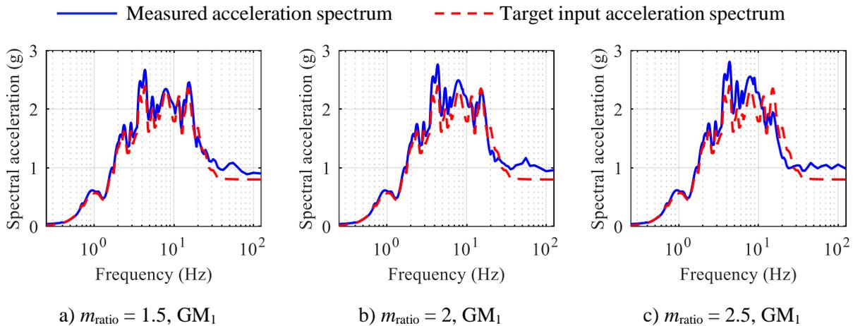
Figure 10.6. Results of acceleration-tracking experiments, different water depths,  $K_c = 5 \text{ V/in}$ ,  $K_p = 0.001 \text{ V/psi}$ ,  $f_c = 80 \text{ Hz}$ ,  $\tau_s = 500 \mu\text{s}$  [2000 Hz]
