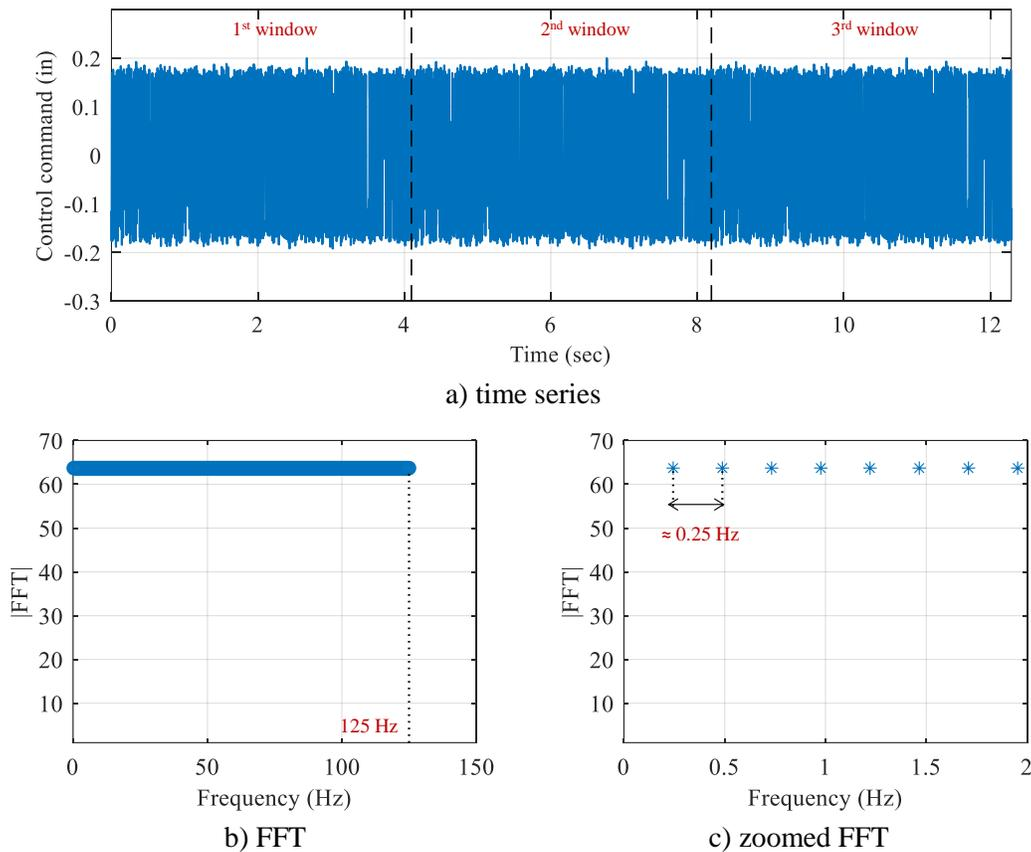
Figure 4.12. Multisine input for the frequency-response experiments
