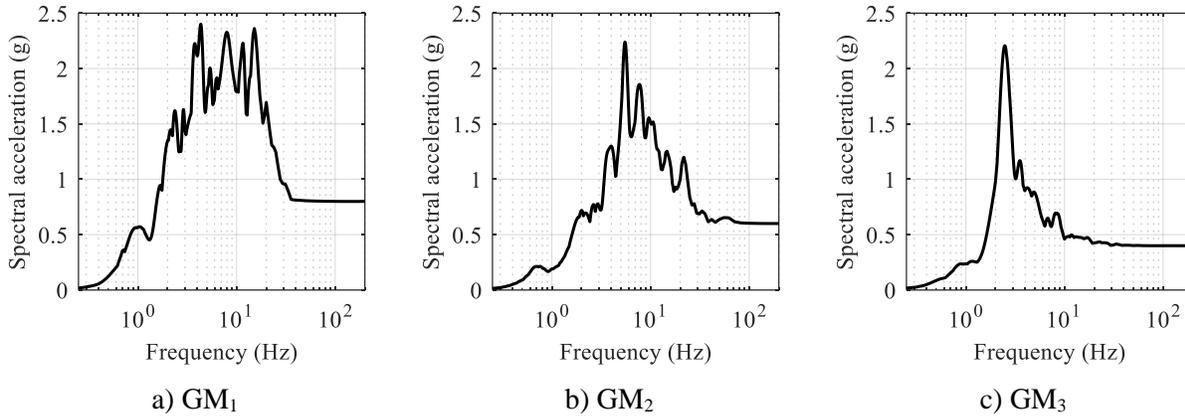
Figure 8.1. 5%-damped acceleration response spectra of the input ground motions
