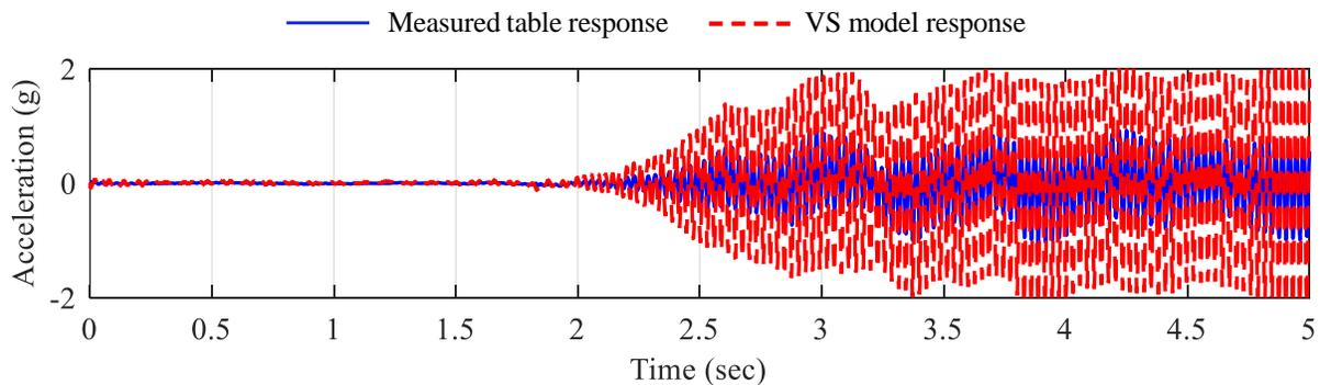
Figure 9.34. Unstable MIL simulation imitating SD<sub>2</sub> system subjected to motion GM<sub>2</sub>,  $m_{vs} = 0.7m_{st}$ ,  $f_c = 80$  Hz,  $K_e = 5$  V/in,  $K_p = 0.001$  V/psi,  $\tau_s = 500$   $\mu$ s [2000 Hz]
