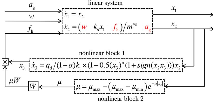
Figure 5.5. Modeling strategy for the FP system: linear system representation with nonlinear components viewed as external inputs in feedback
