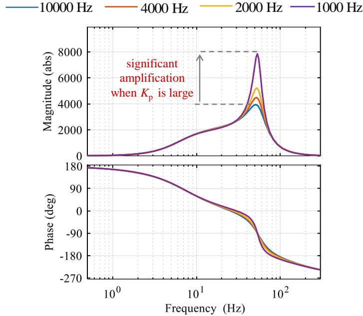
Figure 10.3. Effect of the controller loop frequency,  $K_e = 5 \text{ V/in}$ ,  $K_p = 0.001 \text{ V/psi}$
