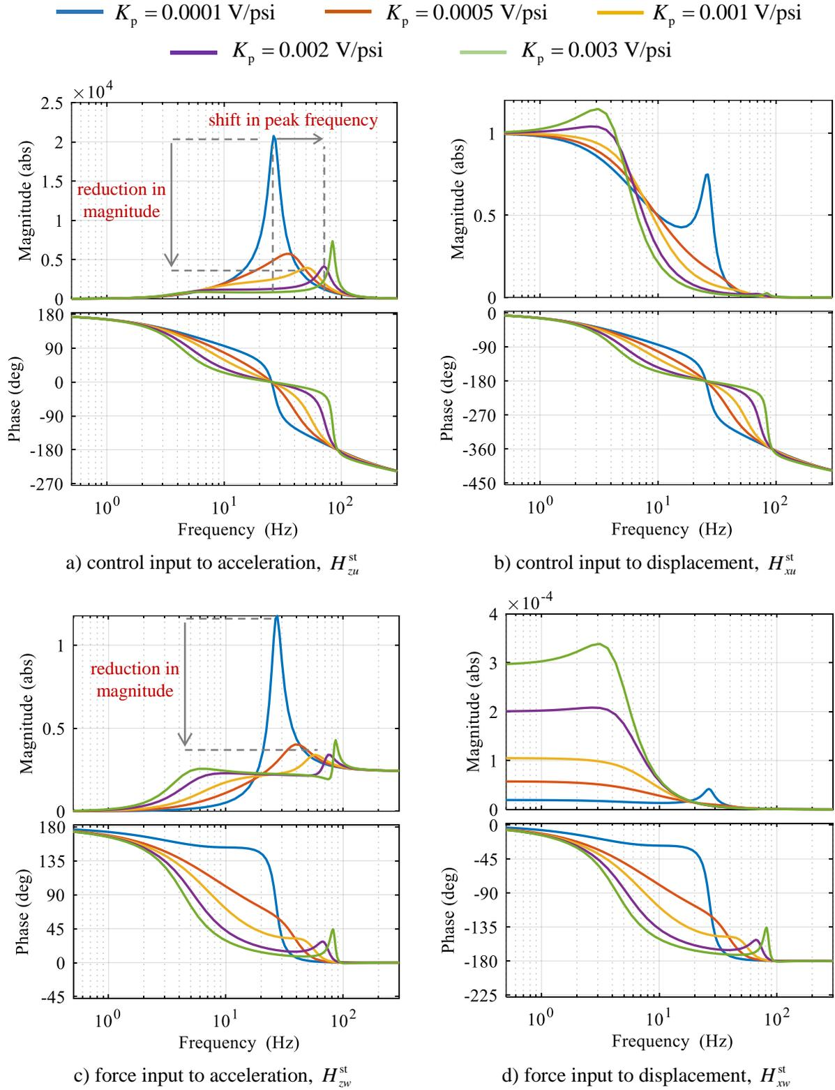
Figure 4.8. Sensitivity of the analytical transfer functions of the shake table to differential pressure gain;  $K_c = 5$  V/in,  $\tau_s = 0$   $\mu$ s
