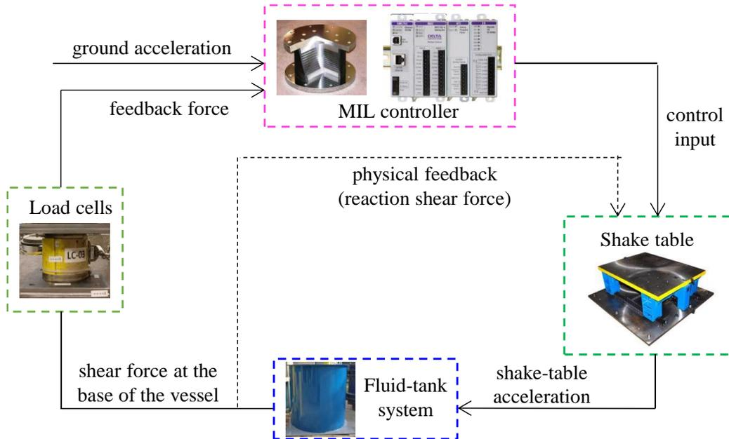
Figure 1.5. Feedback interaction in the MIL experiments
