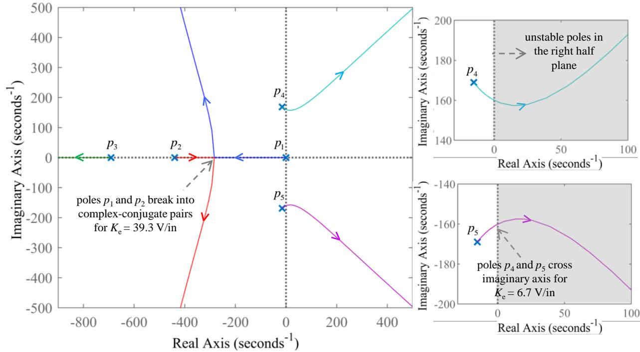
Figure 4.7. Root locus of the shake-table poles for increasing values of  $K_e$ ;  $K_p = 0$  V/psi and  $\tau_s = 0$   $\mu$ s
