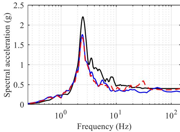
b) 5%-damped acceleration spectra
