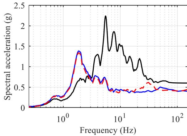
b) 5%-damped acceleration spectra
