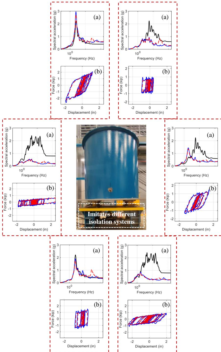
Figure 1.7. Sample test results; panels marked (a) present the acceleration response spectra at the base of the vessel, and panels marked (b) present the force-displacement response of the isolation system to the input motion; solid blue lines are the shake table responses, dashed red lines are the responses of the isolation system model, and the solid black lines are the acceleration spectra of the input ground motion.
