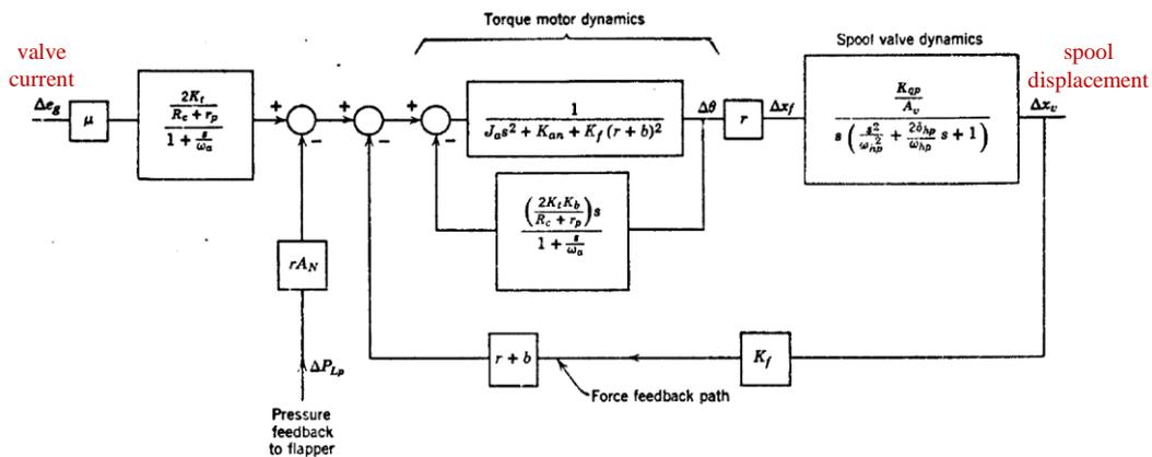
Figure 4.2. Block diagram for a two-stage servovalve model (Merritt, 1967)
