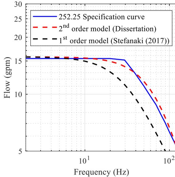
Figure 10.1. Modeling of servovalve dynamics using MTS specification curve (MTS, 2003)
