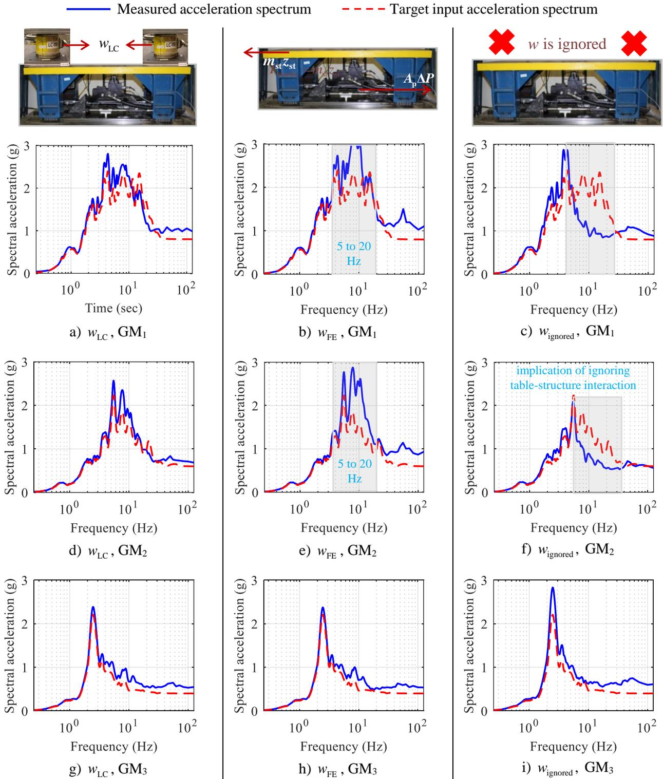
Figure 8.9. Results of acceleration-tracking experiments, different feedback measurements,  $d_w = 42$  inches,  $K_e = 5$  V/in,  $K_p = 0.001$  V/psi,  $f_c = 80$  Hz,  $\tau_s = 500 \mu\text{s}$  [2000 Hz]
