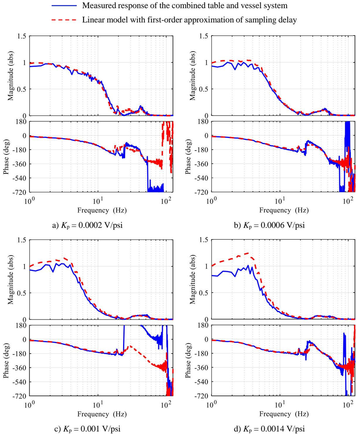
Figure 4.17. Experimental evaluation of the combined table and vessel system, displacement responses, different values of  $K_p$ , water depth of 36 inches,  $K_e = 5$  V/in, and  $\tau_s = 500 \mu s$
