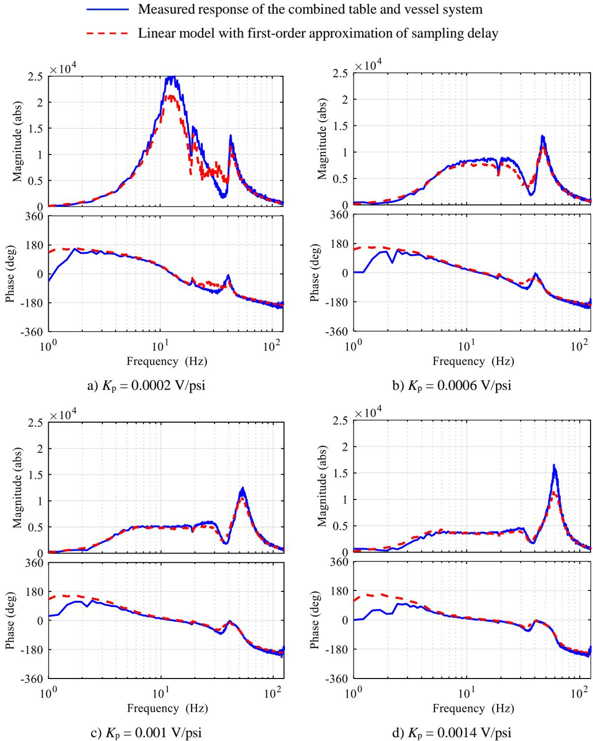
Figure 4.18. Experimental evaluation of the combined table and vessel system, differential pressure responses, different values of  $K_p$ , water depth of 36 inches,  $K_e = 5$  V/in, and  $\tau_s = 500 \mu s$
