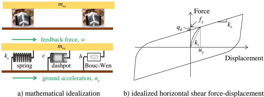
Figure 5.2. Nonlinear lead-rubber virtual system
