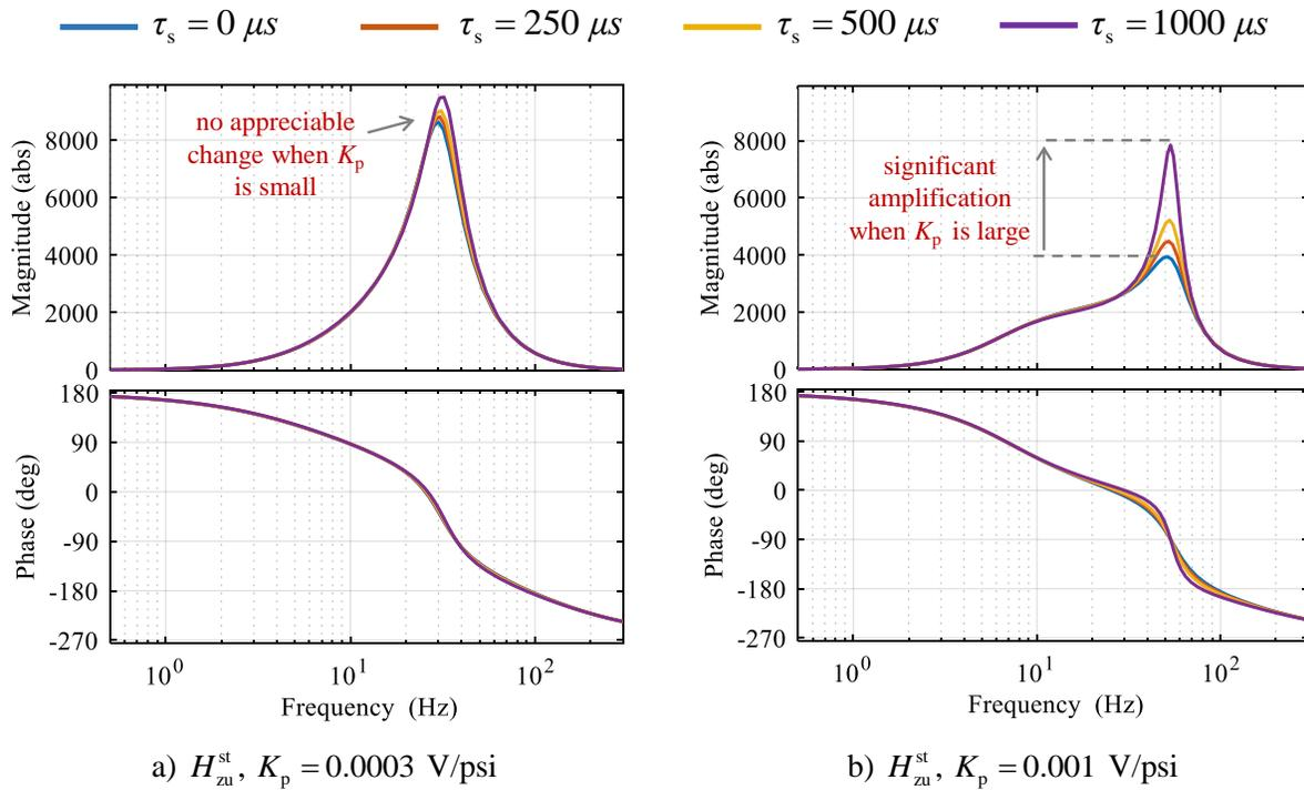
Figure 4.10. Sensitivity of the analytical transfer functions of the shake table to controller loop time;  $K_e = 5$  V/psi
