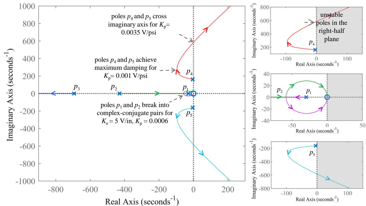
Figure 4.9. Root locus of shake-table poles for increasing values of  $K_p$ ;  $K_e = 5$  V/in and  $\tau_s = 0$   $\mu$ s
