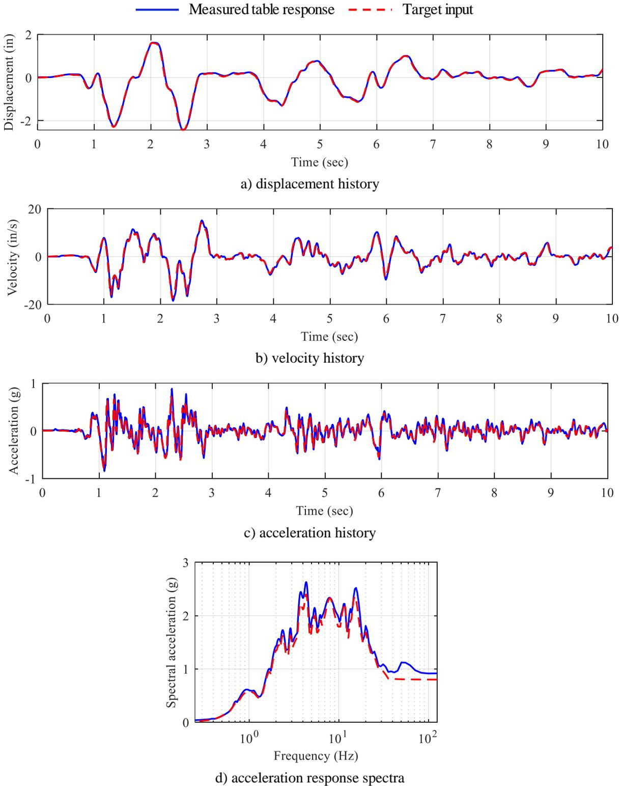
Figure 8.2. Results of acceleration-tracking experiments,  $GM_1$ , empty vessel ( $m_{ratio} = 0.75$ ),  $K_e = 5$  V/in,  $K_p = 0.001$  V/psi,  $f_c = 80$  Hz,  $\tau_s = 500$   $\mu$ s [2000 Hz]
