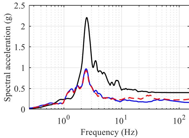
b) 5%-damped acceleration spectra
