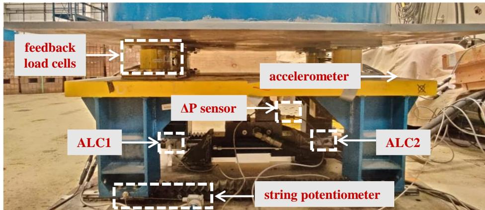
Figure 7.1. Instrumentation of the uniaxial shake table
