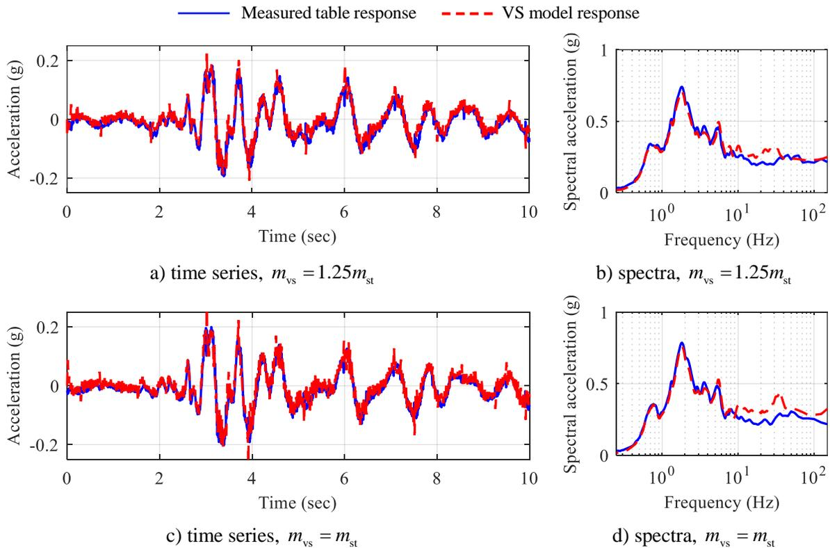
Figure 9.33. Effect of decreasing VS basemat mass ratio for imitating SD<sub>2</sub> system subjected to motion GM<sub>2</sub>,  $f_c = 80$  Hz,  $K_e = 5$  V/in,  $K_p = 0.001$  V/psi,  $\tau_s = 500 \mu s$  (2000 Hz)
