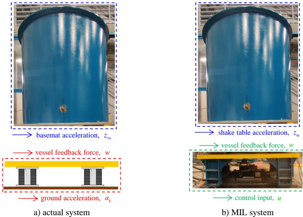
Figure 1.4. MIL conceptualization for 1D base-isolated equipment
