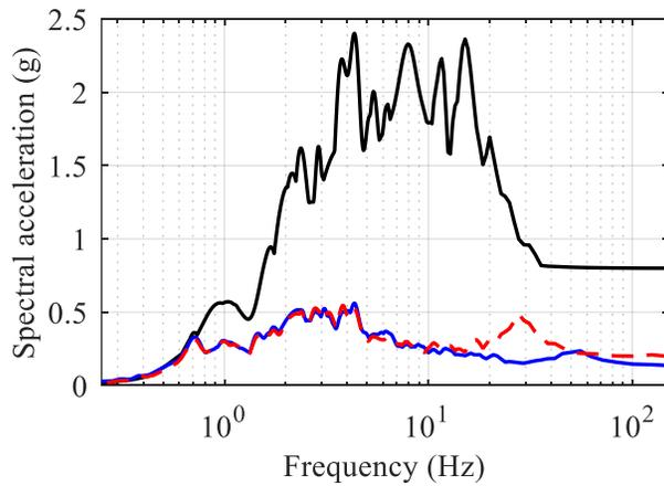
b) 5%-damped acceleration spectra
