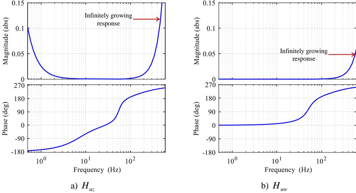
Figure 6.1. Bode plots of the controller transfer functions; properties per Table 4-1
