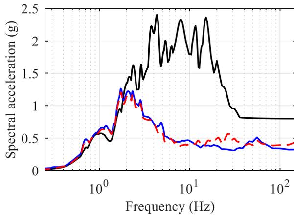
b) 5%-damped acceleration spectra
