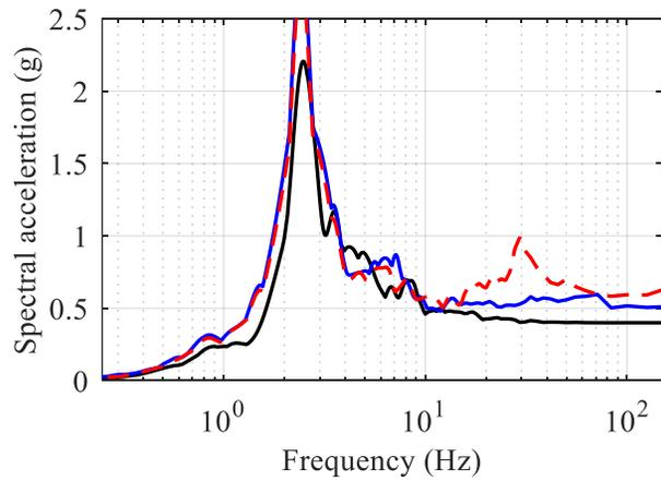
b) 5%-damped acceleration spectra
