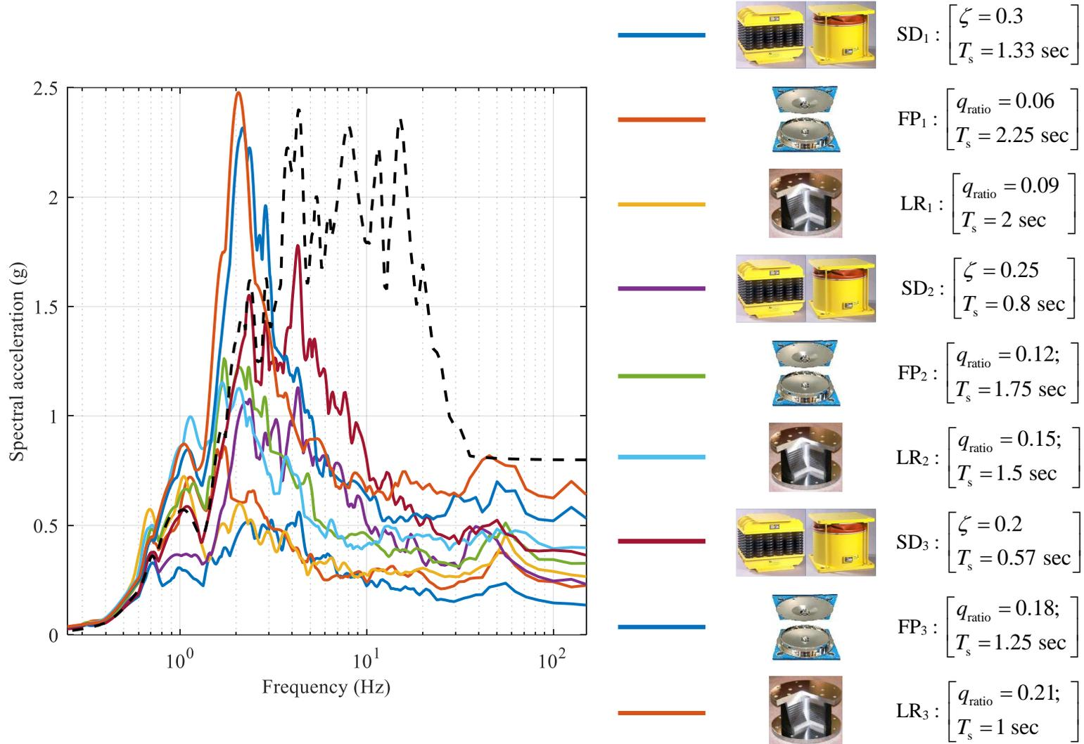
Figure 9.29. Response spectra (5% damped) of the measured shake-table acceleration imitating different seismic isolation systems; GM<sub>1</sub>
