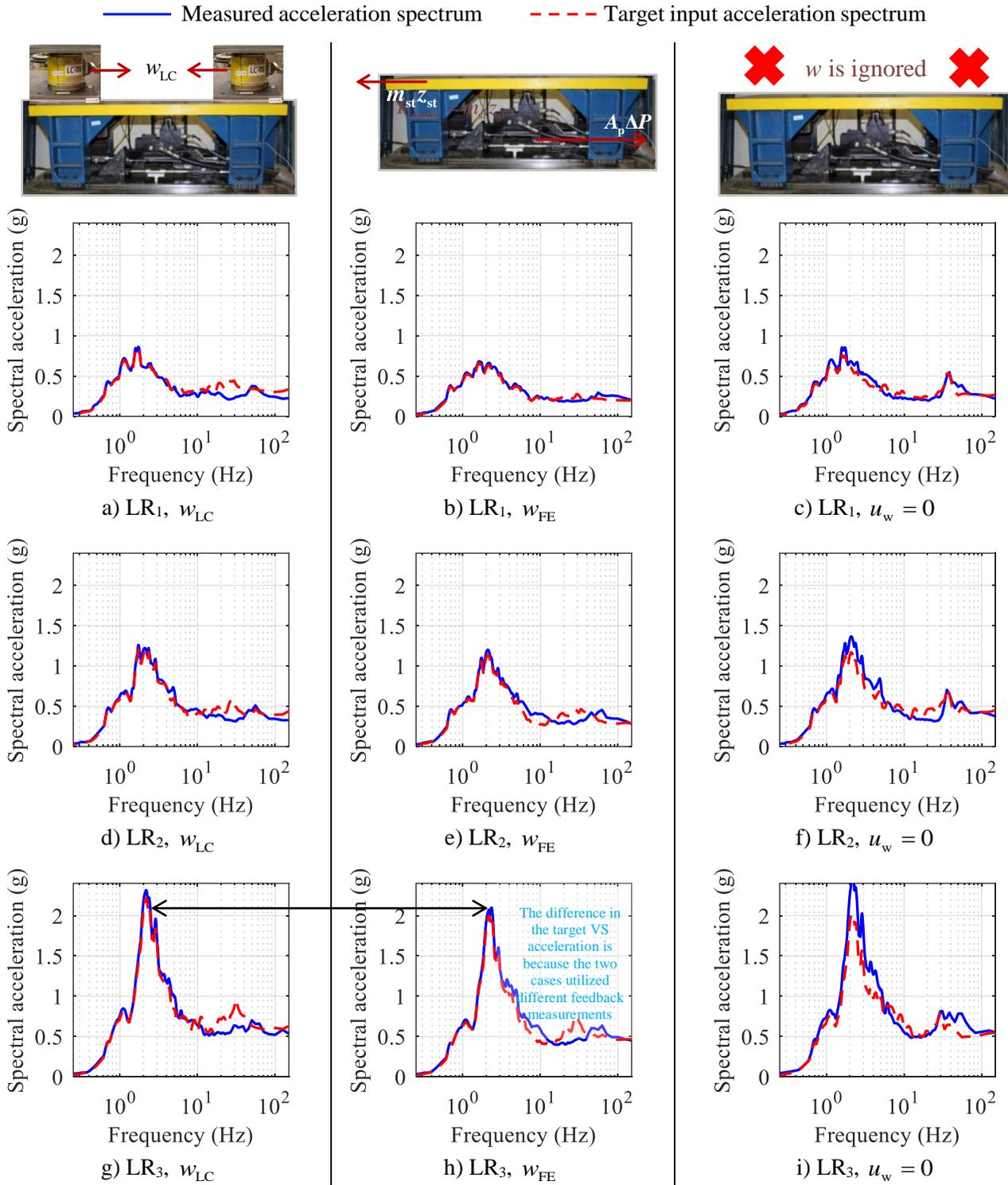
Figure C.2. Effect of different sources of feedback measurement on MIL performance imitating SD isolation systems for GM<sub>1</sub>
