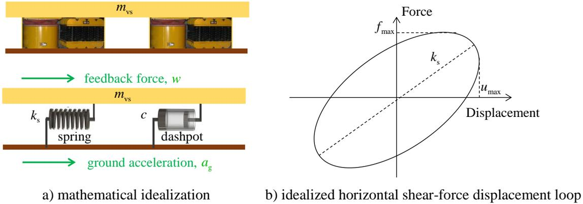
Figure 5.1. Linear spring-damper virtual system
