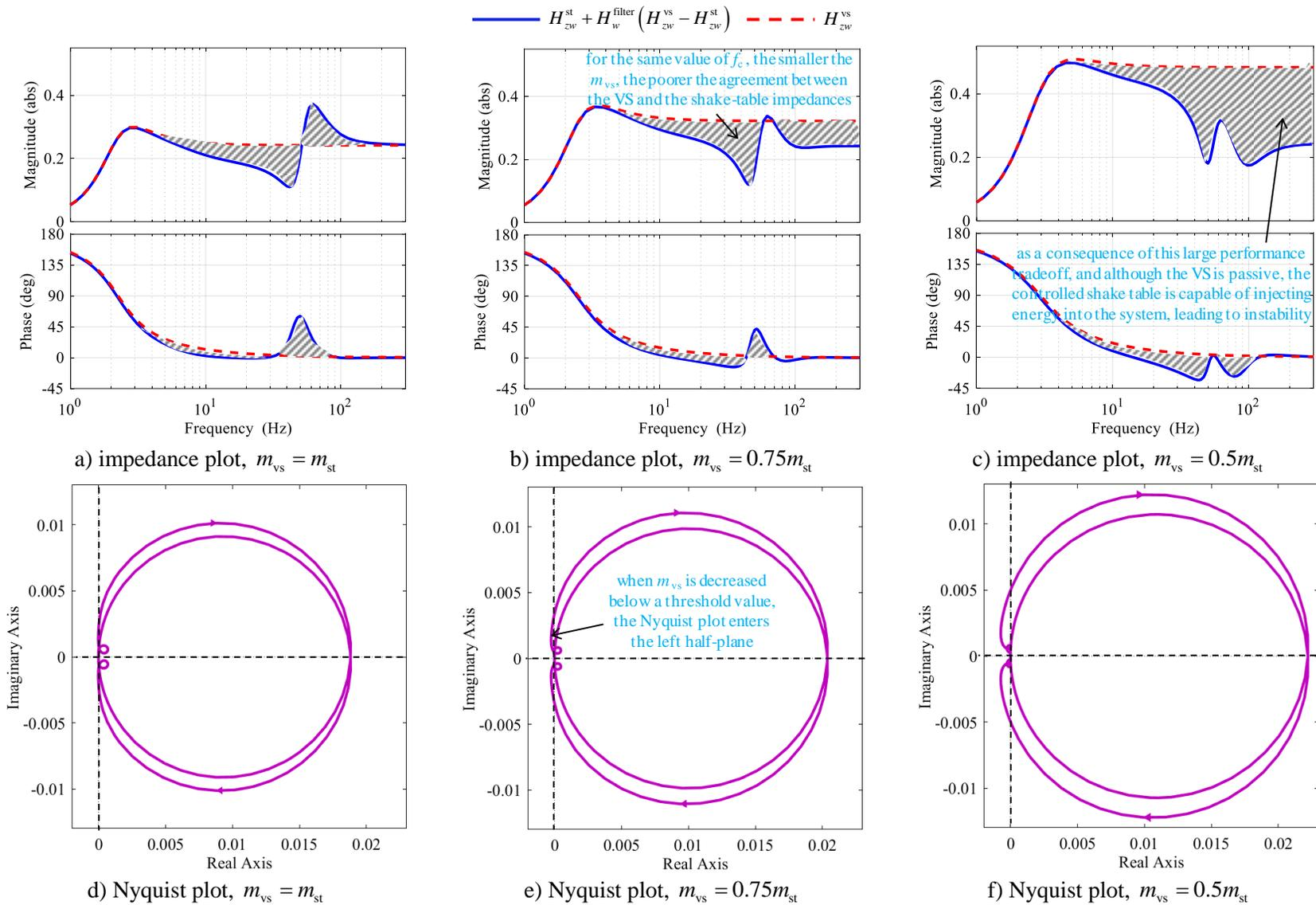
Figure 9.32. Understanding the effect of VS basemat mass,  $K_e = 5$  V/in,  $K_p = 0.001$  V/psi,  $\tau_s = 500$   $\mu$ s (2000 Hz), and  $f_c = 80$  Hz
