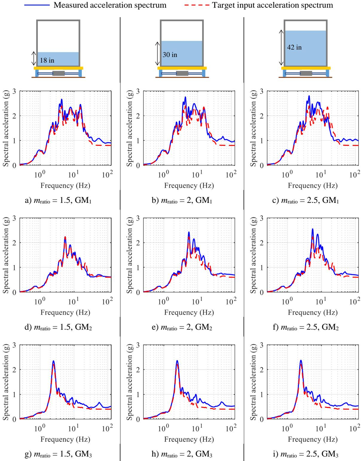
Figure 8.5. Results of acceleration-tracking experiments, different water depths and input motions,  $K_e = 5 \text{ V/in}$ ,  $K_p = 0.001 \text{ V/psi}$ ,  $f_c = 80 \text{ Hz}$ ,  $\tau_s = 500 \mu\text{s}$  [2000 Hz]
