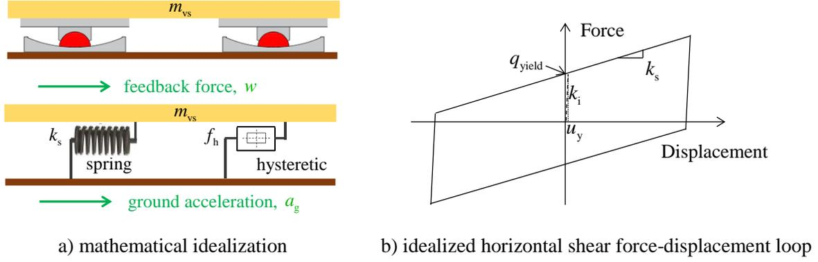
Figure 5.4. Nonlinear single concave Friction Pendulum VS
