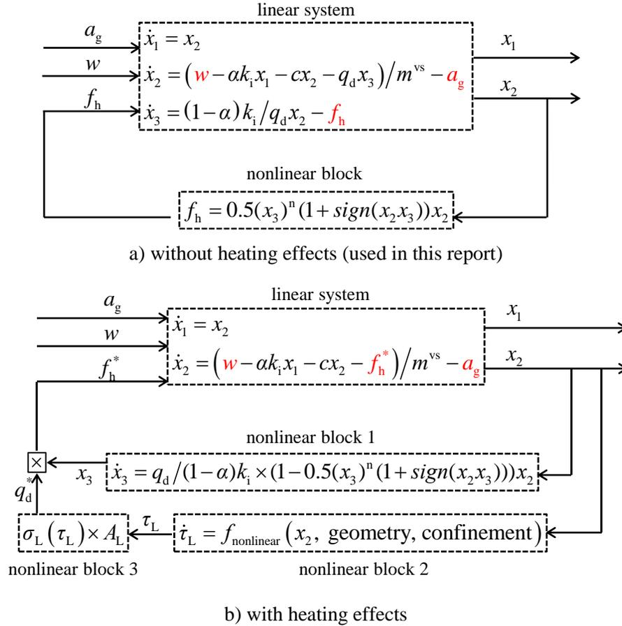
Figure 5.3. Modeling strategy for the LR system: linear system representation with nonlinear components viewed as external inputs in feedback
