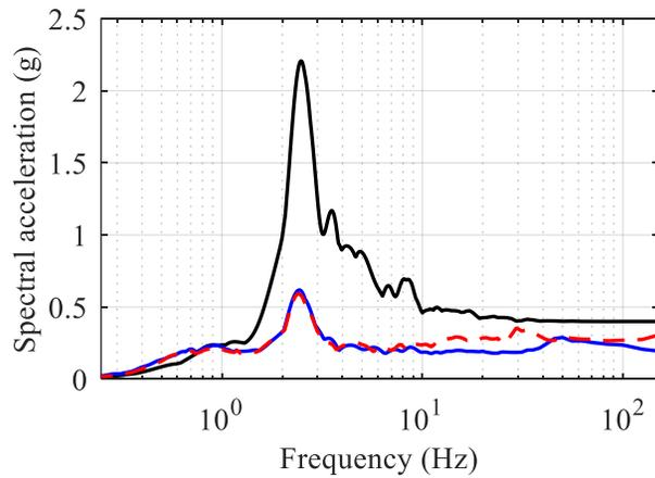
b) 5%-damped acceleration spectra
