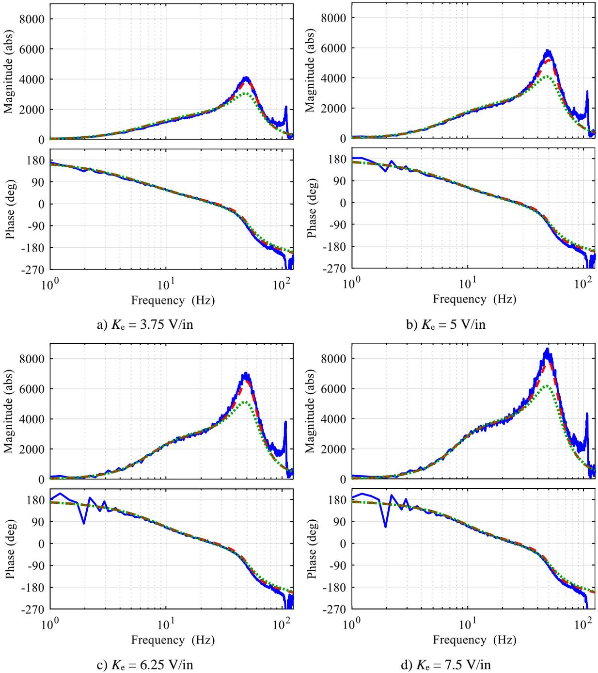
Figure 4.14. Experimental evaluation of the bare shake table for different values of  $K_e$ ;  $K_p = 0.0009$  V/p si and  $\tau_s = 500$   $\mu$ s.
