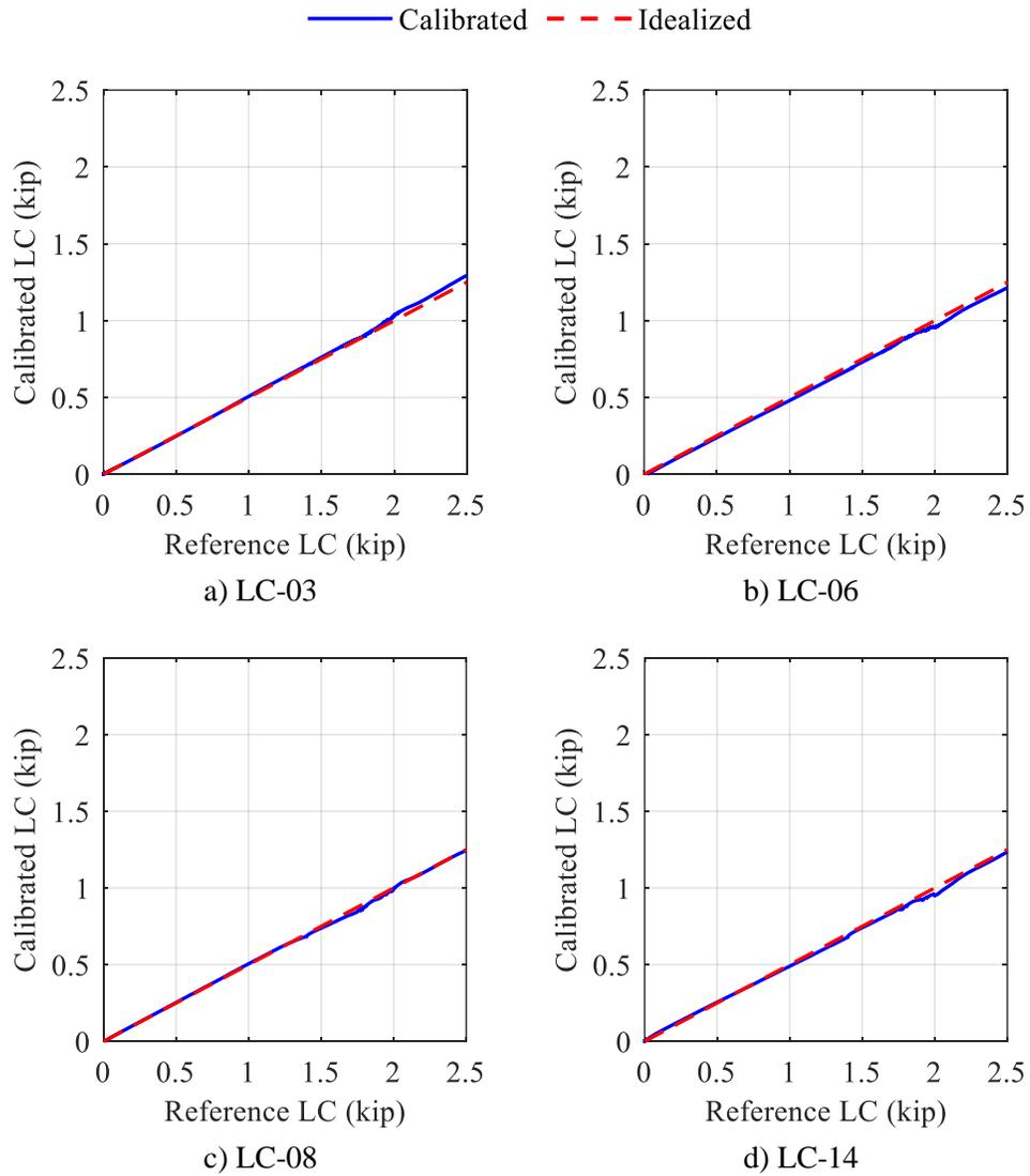
Figure A.2. Calibration charts for the shear-x channels
