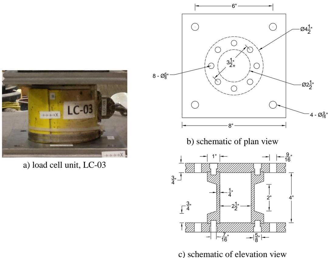
Figure 3.5. Reaction load cells for measuring the feedback force (Bracci *et al.*, 1992)
