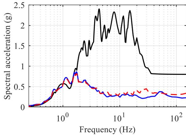
sb) 5%-damped acceleration spectra
