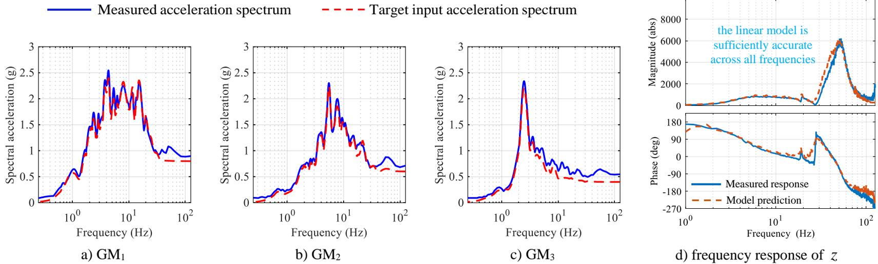
Figure 8.12. Results of acceleration-tracking experiments,  $K_e = 5$  V/in,  $K_p = 0.001$  V/psi,  $f_c = 80$  Hz,  $\tau_s = 500$   $\mu$ s [2000 Hz]
