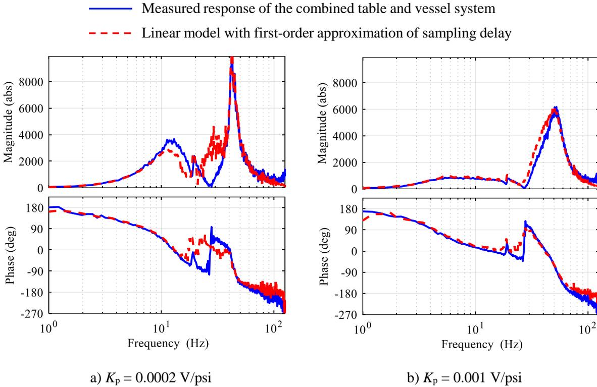
Figure 10.2. Experimental evaluation of the table and vessel system, acceleration responses, different values of  $K_p$ , water depth 36 inches,  $K_c = 5$  V/in, and  $\tau_s = 500 \mu s$
