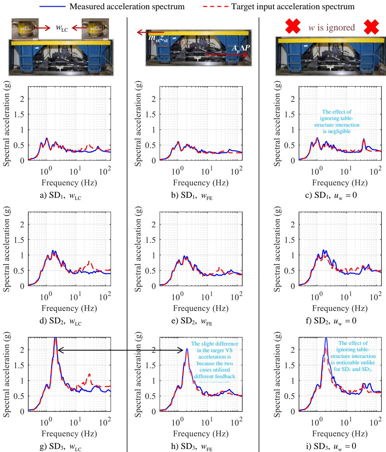
Figure C.1. Effect of different sources of feedback measurement on MIL performance imitating SD isolation systems for  $GM_1$
