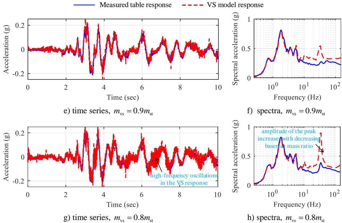
Figure 9-33. Effect of decreasing VS basemat mass ratio for imitating SD<sub>2</sub> system subjected to motion GM<sub>2</sub>,  $f_c = 80$  Hz,  $K_e = 5$  V/in,  $K_p = 0.001$  V/psi,  $\tau_s = 500$   $\mu$ s (2000 Hz) (cont'd)
