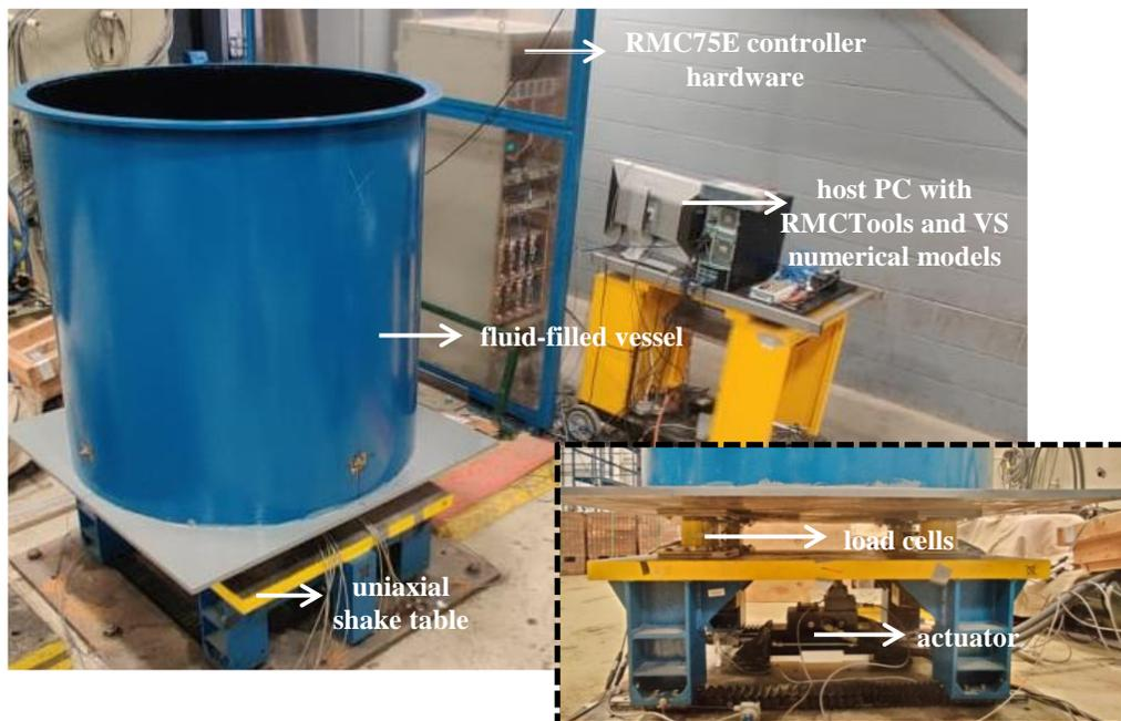
Figure 3.1. MIL test setup for the 1D base-isolated fluid-filled cylindrical vessel
