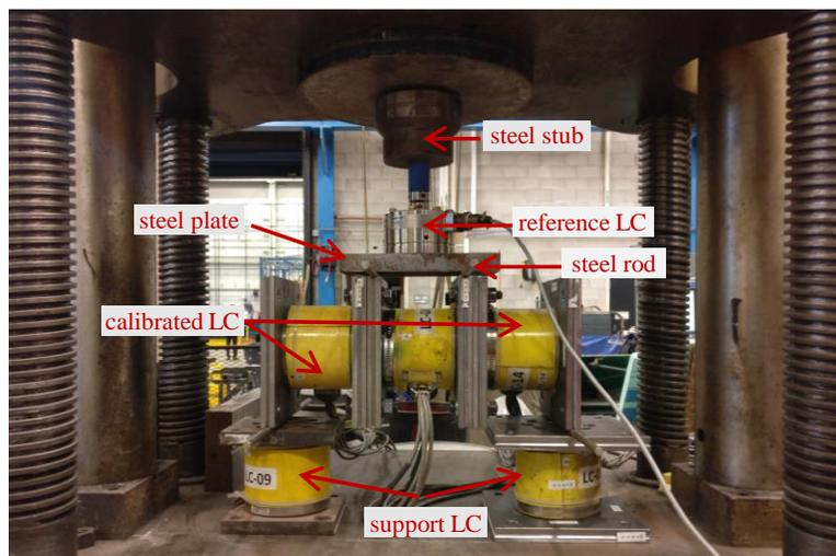
Figure A.1. Calibration setup for the load cells
