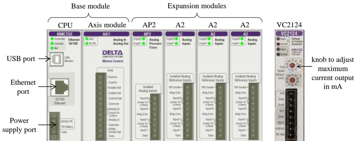
Figure 3.6. RMC controller hardware
