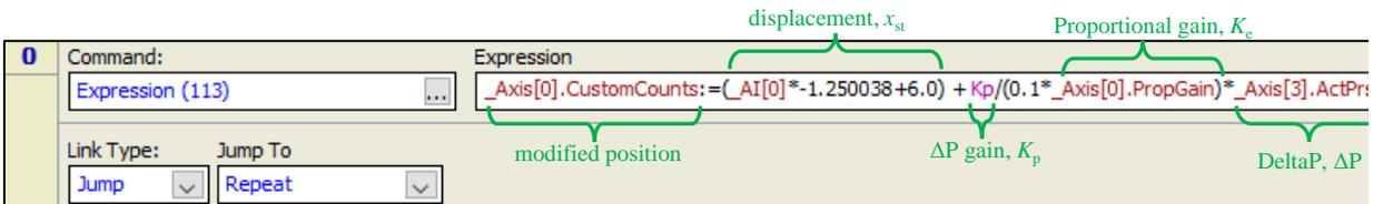
Figure 7.6. User program for implementing the hydraulic control loop in the RMCTools
