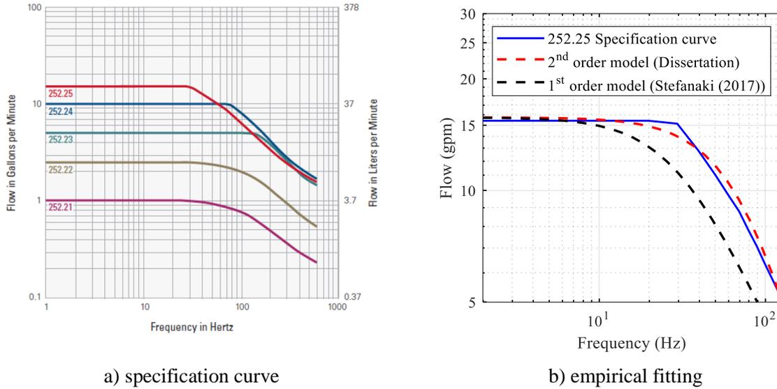
Figure 4.3. Modeling of servovalve dynamics using MTS specification curve (MTS, 2003)
