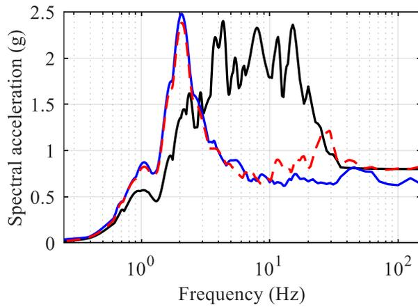
b) 5%-damped acceleration spectra
