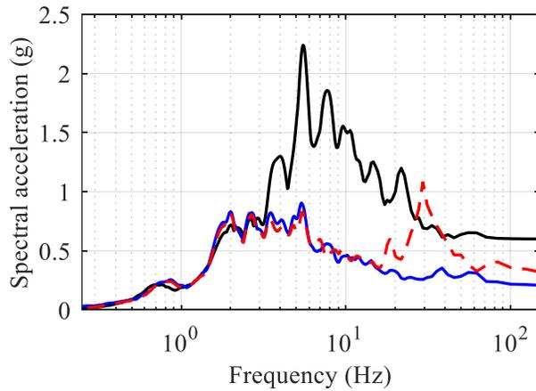
b) 5%-damped acceleration spectra
