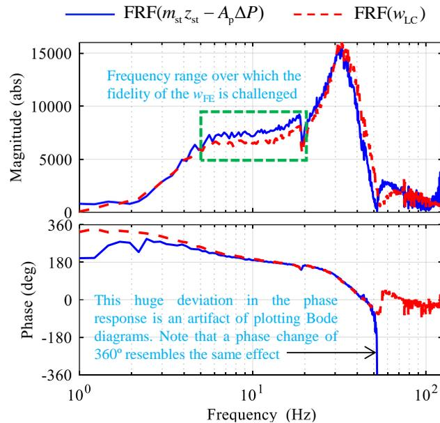
Figure 8.7. Frequency response measurements of the combined table and the vessel system,  $d_w = 36$  inches,  $K_e = 5$  V/in,  $K_p = 0.001$  V/psi, and  $\tau_s = 500$   $\mu$ s [2000 Hz]
