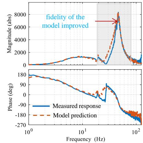
Figure 8.11. Results of acceleration-tracking experiments,  $K_e = 5$  V/in,  $K_p = 0.0006$  V/psi,  $f_c = 80$  Hz,  $\tau_s = 500$   $\mu$ s [2000 Hz]
