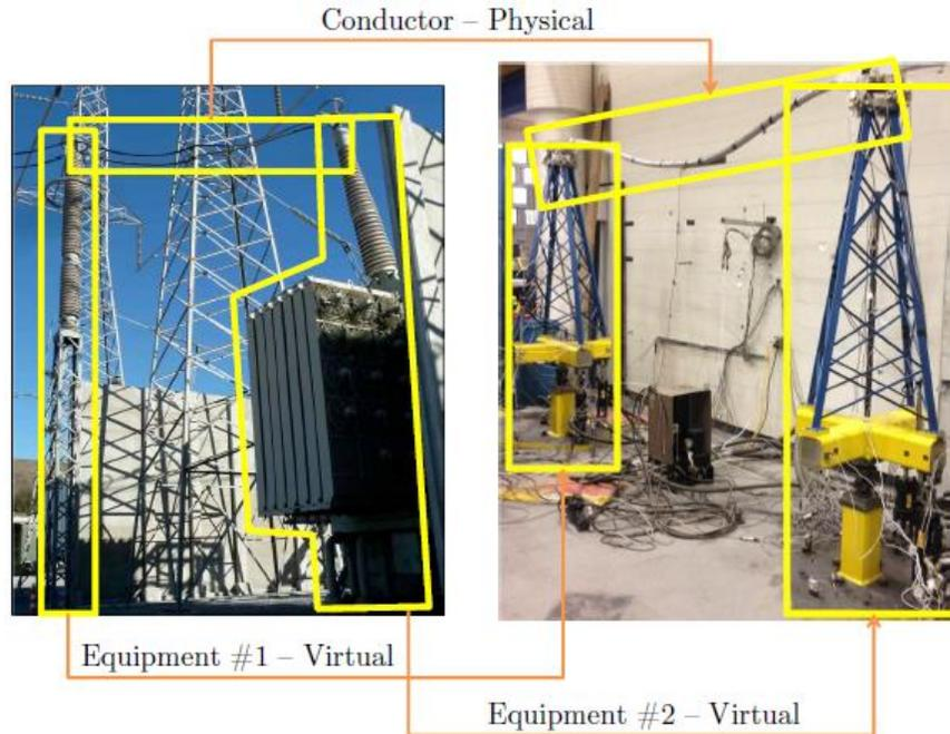
Figure 2.3. MIL test configuration for physical flexible bus conductors with interconnected equipment represented virtually using the 2DOF shakers (Kote, 2019)
