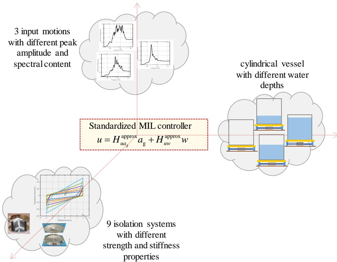
Figure 1.6. Validation of MIL controls for a family of physical and virtual systems
