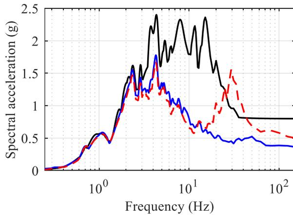
b) 5%-damped acceleration spectra
