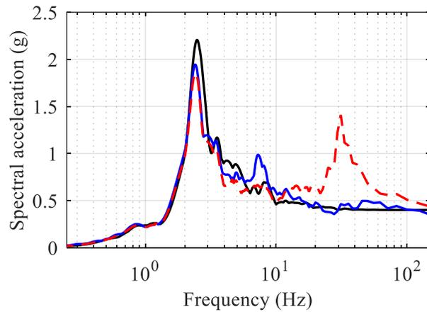
b) 5%-damped acceleration spectra
