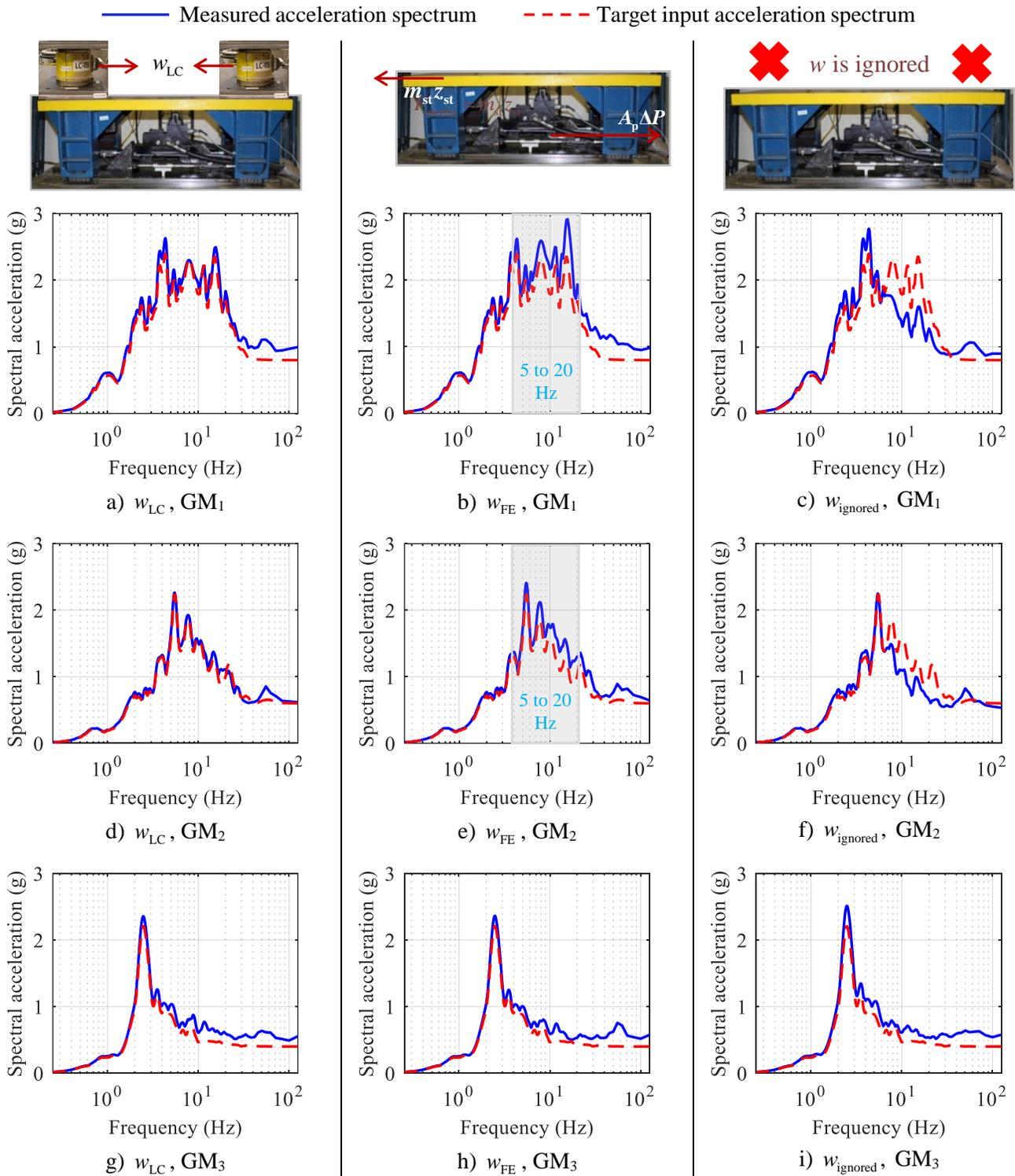
Figure 8.8. Results of acceleration-tracking experiments, different feedback measurements, empty vessel,  $K_c = 5 \text{ V/in}$ ,  $K_p = 0.001 \text{ V/psi}$ ,  $f_c = 80 \text{ Hz}$ ,  $\tau_s = 500 \mu\text{s}$  [2000 Hz]
