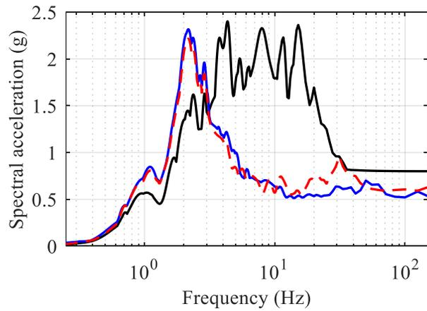
b) 5%-damped acceleration spectra
