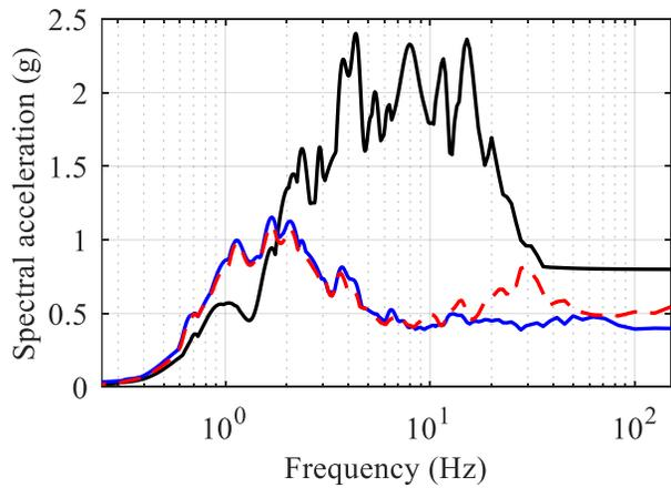
b) 5%-damped acceleration spectra
