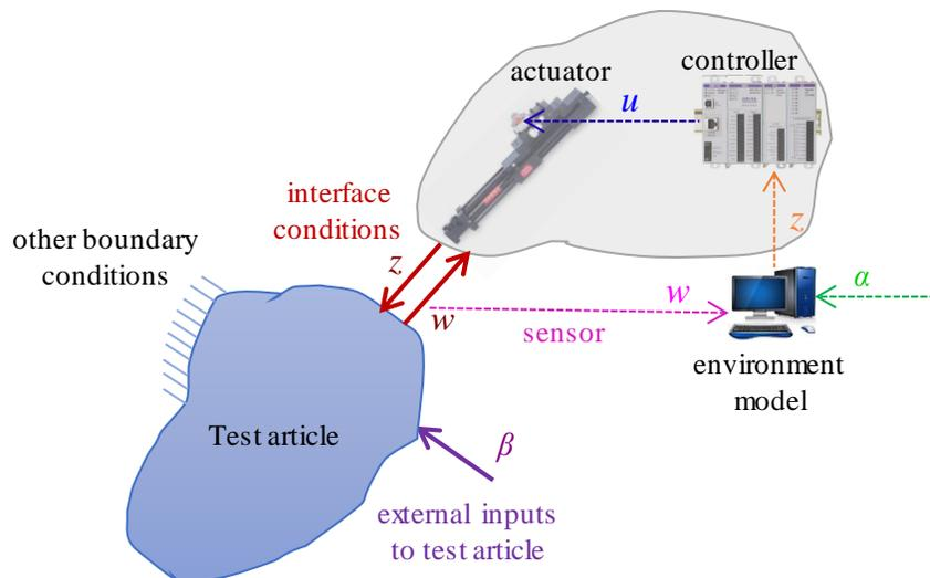
c) MIL testing; solid lines represent physical inputs and dashed lines represent electronic signals
