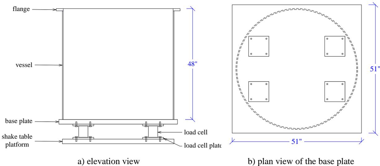
Figure 3.2. Elevation and plan views of the test article
