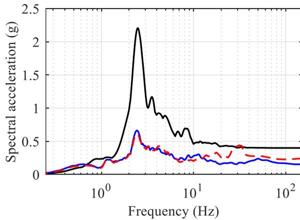
b) 5%-damped acceleration spectra
