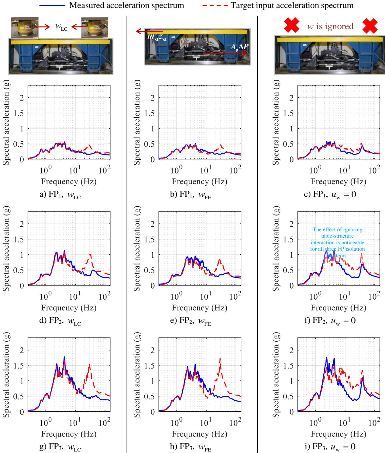
Figure C.3. Effect of different sources of feedback measurement on MIL performance imitating SD isolation systems for  $GM_1$
