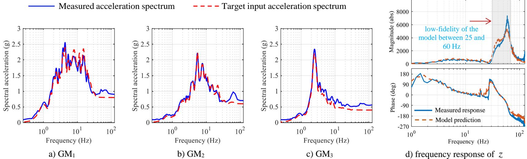
Figure 8.13. Results of acceleration-tracking experiments,  $K_e = 5$  V/in,  $K_p = 0.0014$  V/psi,  $f_c = 80$  Hz,  $\tau_s = 500$   $\mu$ s [2000 Hz]
