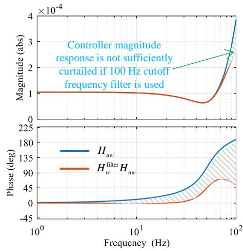
a) controller frequency response,  $f_c = 100$  Hz
