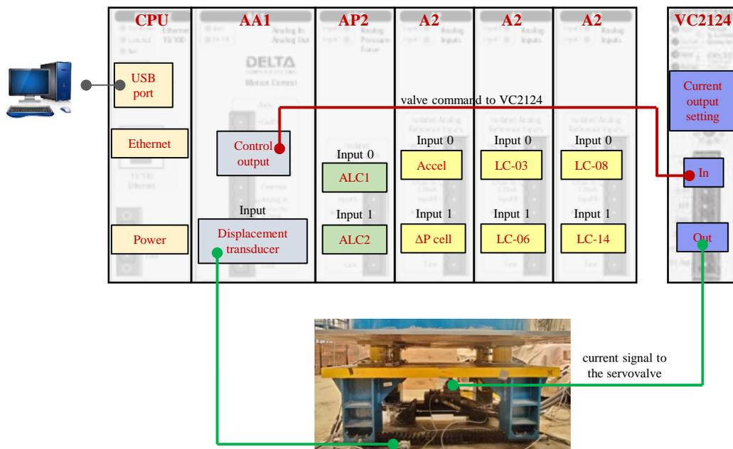
Figure 7.2. Configuring the RMC75E hardware with the uniaxial shake table
