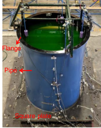
(b) tank containing water (dyed to green): view from the south and top
