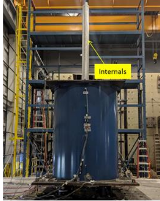
Figure 5.12. Internals attached to the vessel head for hammer impact tests
