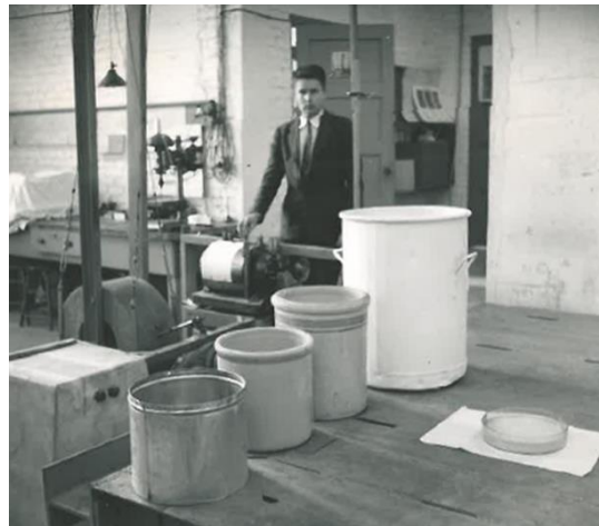
Figure 2.7. Cylindrical tanks on shaking table, adapted from Plate XXIV in Morris (1938)
