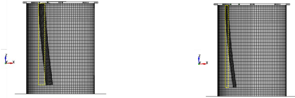
(a) FE model 3A (without fluid), frequency = 15.7 Hz
