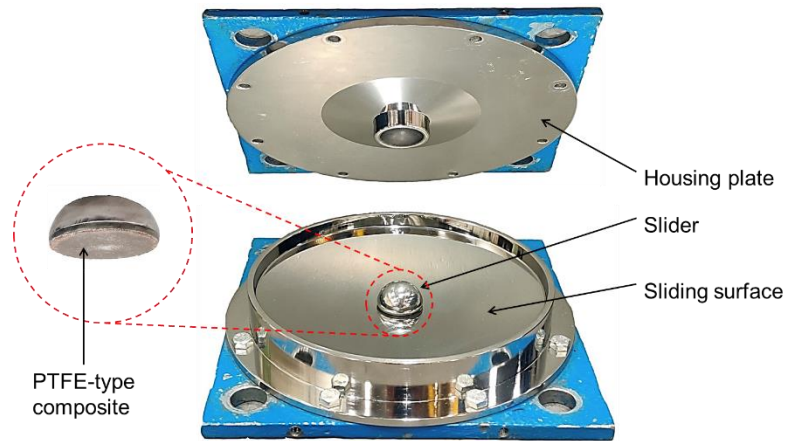
Figure 7.3. Components of an SFP isolator (Lal et al. 2021)
