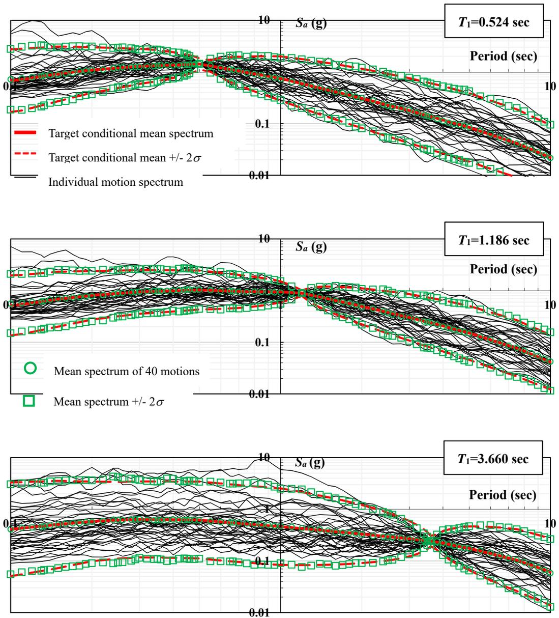
Figure B-8 Spectra of Scaled Motions and Conditional Spectra for Return Period of 949 Years and Period  $T_1$  Equal to 0.524, 1.186 and 3.660 Seconds
