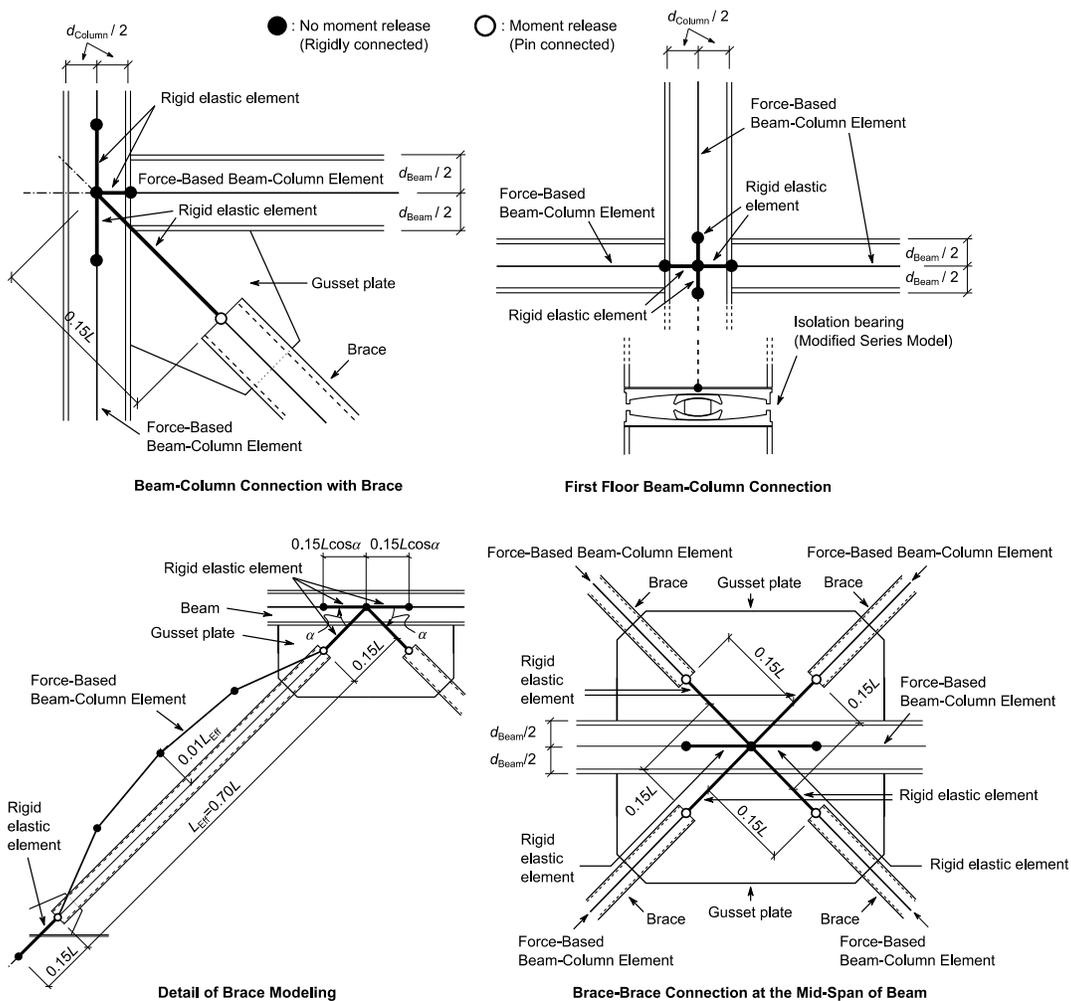
Figure 3-4 Details of Model of Connections
