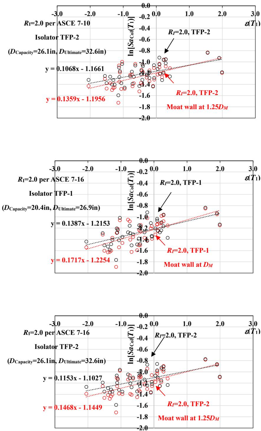
Figure A-6 Relationship between  $\ln[Sa_{CoI}(T_1)]$  and  $\epsilon(T_1)$  for Isolated Buildings with SCBF Designed for  $R_I=2.0$  and Isolator TFP-1 ( $D_{Capacity}=20.4in, D_{Ultimate}=26.9in$ ) or Isolator TFP-2 ( $D_{Capacity}=26.1in, D_{Ultimate}=32.6in$ ) with and without Moat Wall
