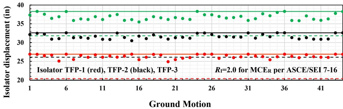
Figure 4-3 Peak Isolator Displacements at Collapse of Buildings with SCBF Designed for the  $MCE_R$  per ASCE/SEI 7-16 and without moat walls
