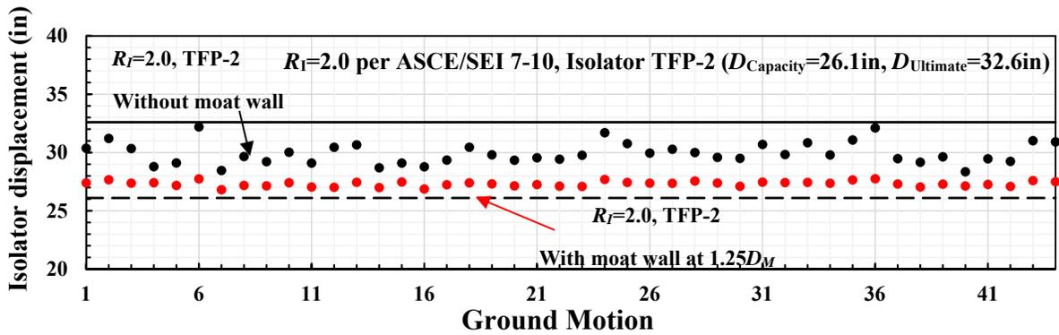
Figure 4-6 Peak Isolator Displacements at Collapse of Buildings with SCBF Designed per ASCE/SEI 7-10, Isolator TFP-2 with and without Moat Wall at Distance  $1.25D_M$
