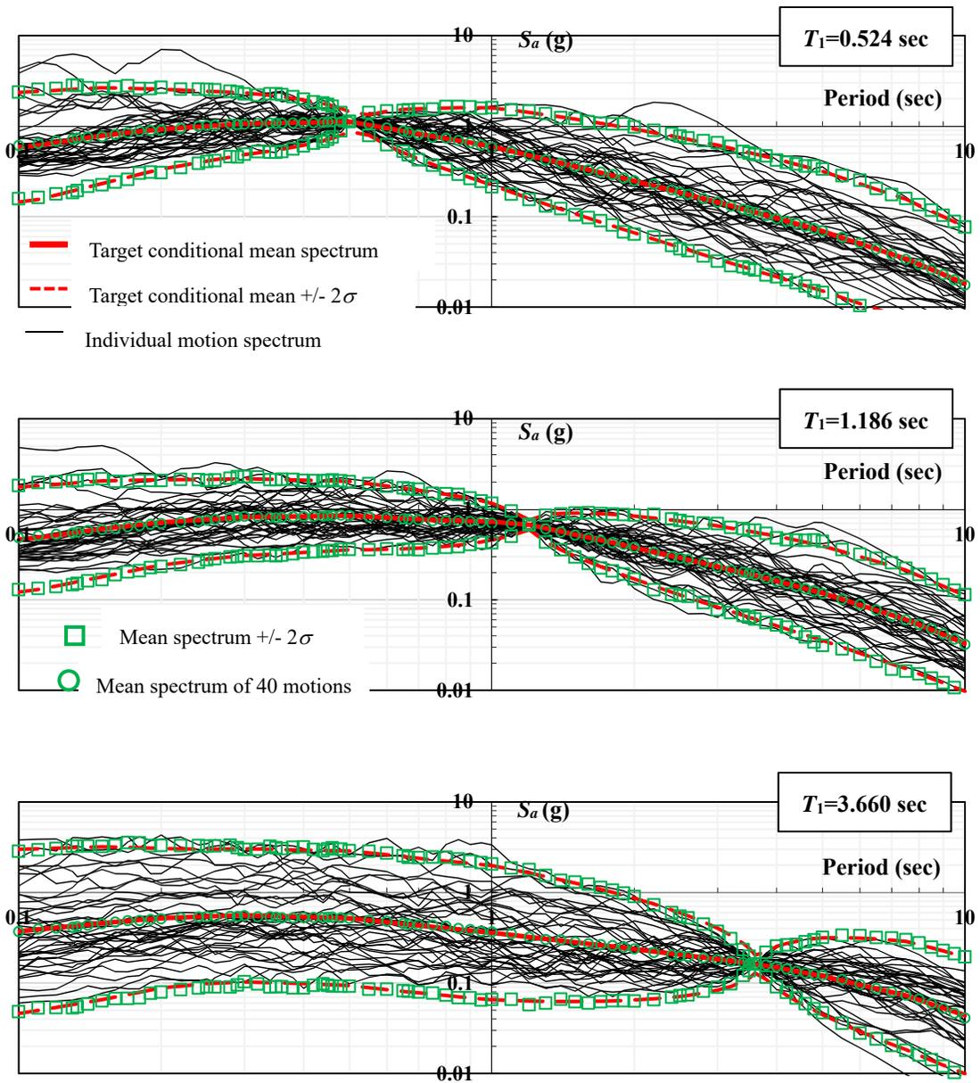
Figure B-7 Spectra of Scaled Motions and Conditional Spectra for Return Period of 475 Years and Period  $T_1$  Equal to 0.524, 1.186 and 3.660 Seconds
