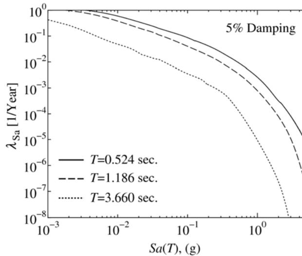
Figure B-1 Seismic Hazard Curves for  $T_1=0.524, 1.186$  and  $3.660$  Seconds
