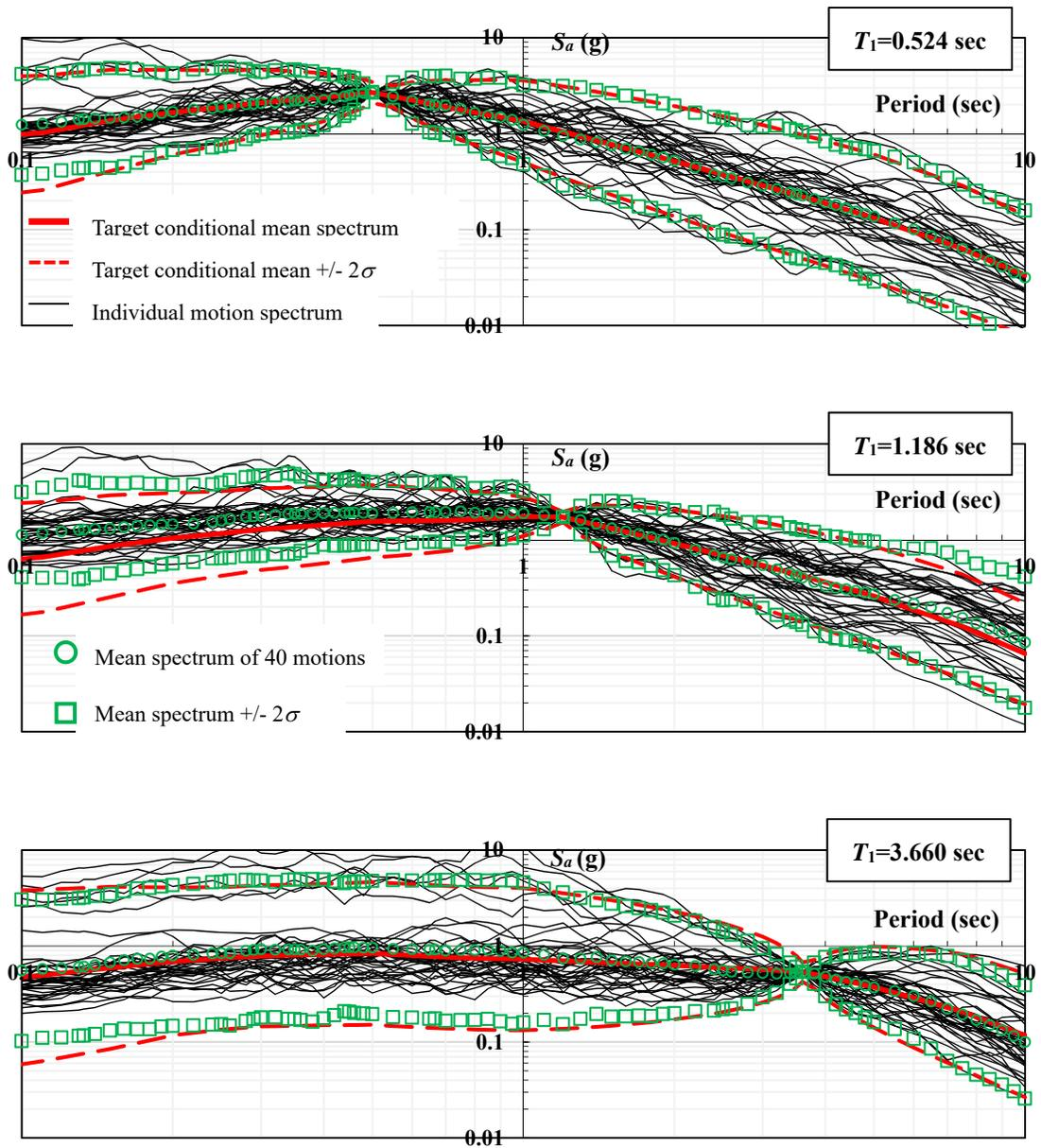
Figure B-12 Spectra of Scaled Motions and Conditional Spectra for Return Period of 7462 Years and Period  $T_1$  Equal to 0.524, 1.186 and 3.660 Seconds
