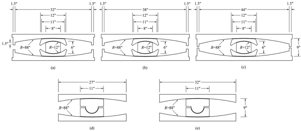
Figure 2-2 Triple FP (TFP) and Double Concave (DC) Isolators of Different Displacement Capacities; (a) TFP-1, (b) TFP-2, (c) TFP-3, (d) DC-1 and (e) DC-2
