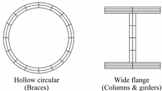
Figure 3-3 Fiber Discretization Used for HSS Brace and Wide Flange Column and Beam
