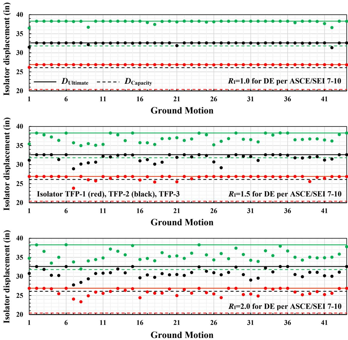
Figure 4-2 Peak Isolator Displacements at Collapse of Buildings with SMF Designed for the DE per ASCE/SEI 7-10 and without moat walls
