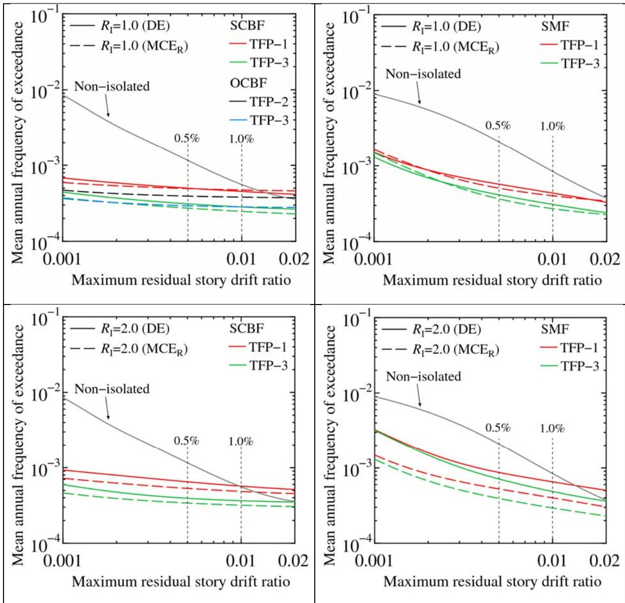
Figure 5-2 Mean Annual Frequency of Exceeding Limits on Peak Residual Story Drift Ratio
