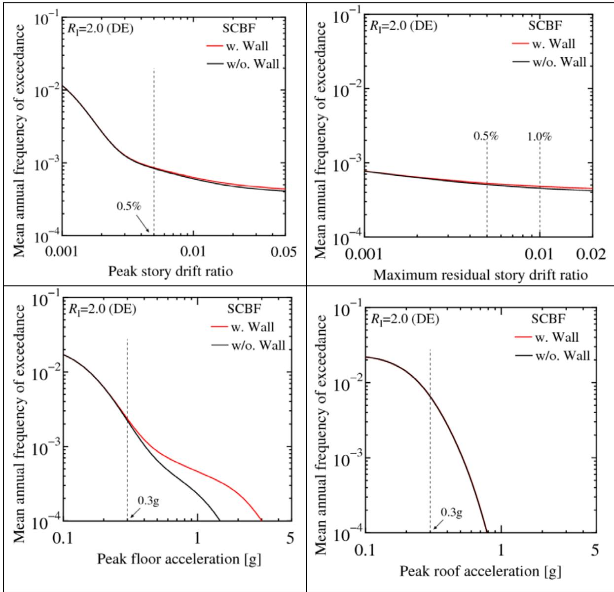
Figure 5-6 Comparisons of Mean Annual Frequency of Exceeding Limits on Drift, Residual Drift and Peak Acceleration for SCBF Designed per ASCE 7-10 for  $R_1=2$ , Isolator TFP-2 without and with Moat Wall at  $1.25D_M$
