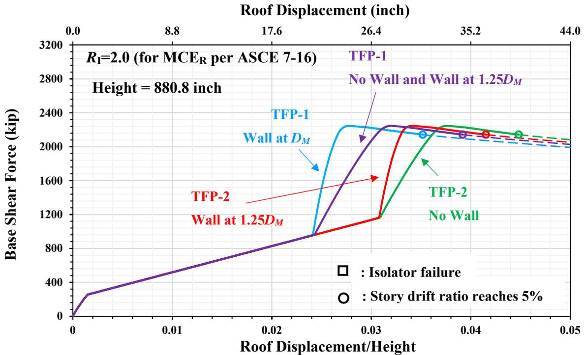
Figure 2-5 Pushover Curves of SCBF in Case of Isolators TFP-1 with  $D_{Capacity}=20.4in (=D_M)$  and TFP-2 with  $D_{Capacity}=26.1in (=1.25D_M)$  and Moat Walls Placed at Distances  $D_M$  and  $1.25D_M$
