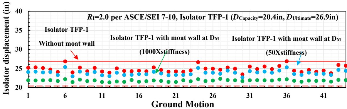
Figure 4-5 Peak Isolator Displacements at Collapse of Buildings with SCBF Designed per ASCE/SEI 7-10, Isolator TFP-1 with and without Moat Wall at Distance  $D_M$
