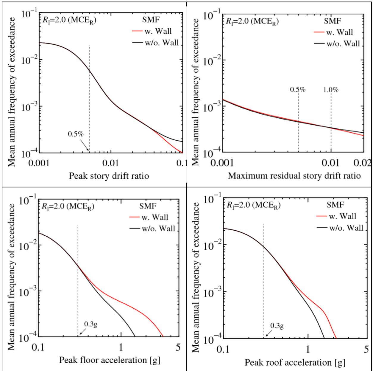
Figure 5-9 Comparisons of Mean Annual Frequency of Exceeding Limits on Drift, Residual Drift and Peak Acceleration for SCBF Designed per ASCE 7-16 for  $R_I=2$ , Isolator TFP-2 without and with Moat Wall at  $1.25D_M$
