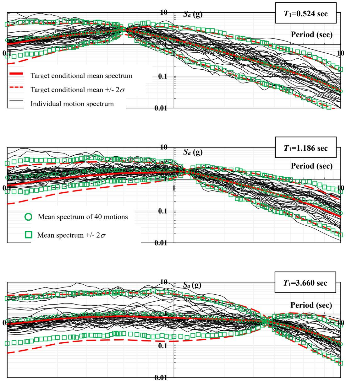
Figure B-13 Spectra of Scaled Motions and Conditional Spectra for Return Period of 10000 Years and Period  $T_1$  Equal to 0.524, 1.186 and 3.660 Seconds
