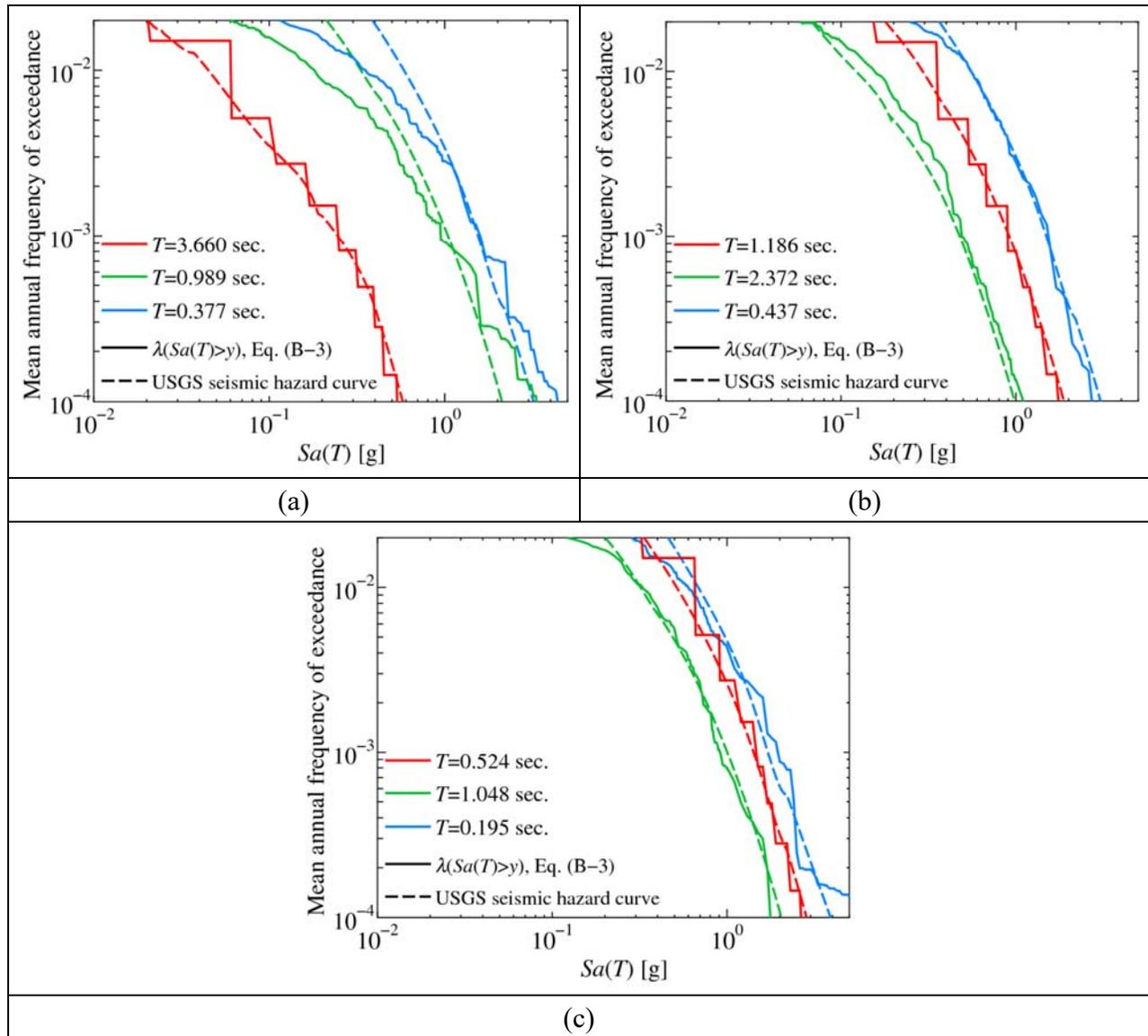
Figure B-14 Comparison of Calculated Mean Annual Frequency Rates Based on Selected Ground Motions (Solid Lines) and USGS Seismic Hazard Curves Dashed Lines) for (a) Isolated Buildings, (b) Non-isolated SMF Building and (c) Non-isolated SCBF Building
