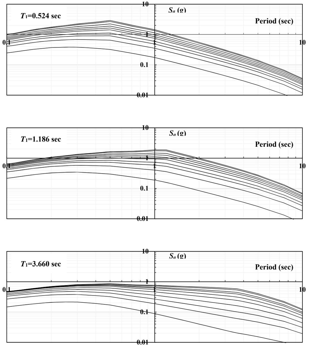
Figure B-3 Conditional Mean Spectra for Return Period of 43, 144, 289, 475, 949, 1485, 2475, 3899, 7462 and 10000 Year and for Building Period  $T_1=0.524$ , 1.186 and 3.660 Second
