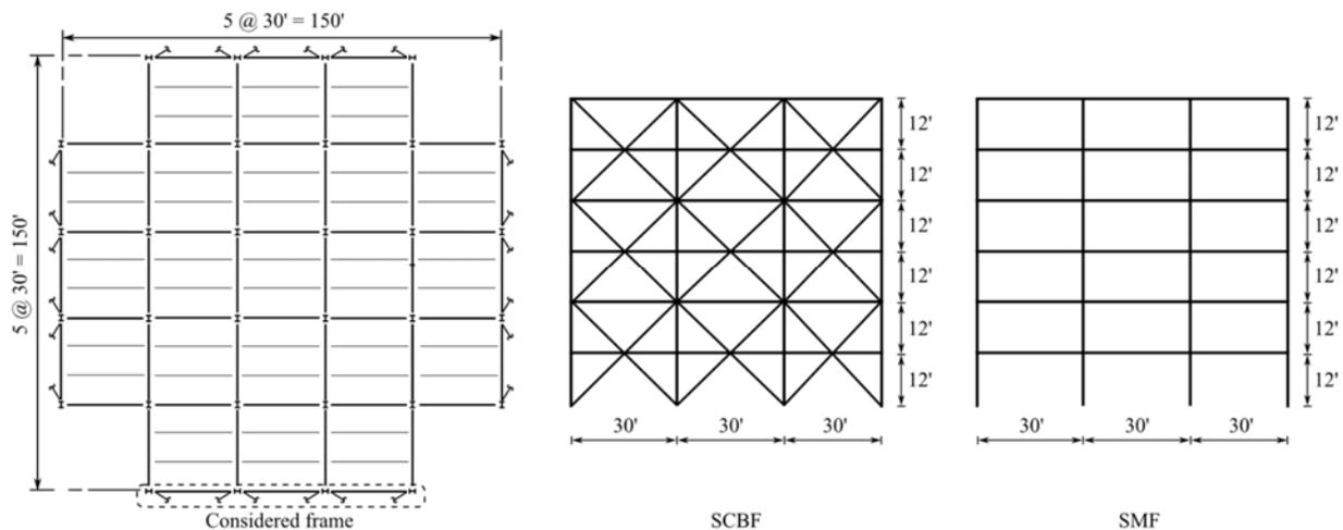
Figure 2-1 Archetypical Building Plan and Views of Braced and Moment Frames
