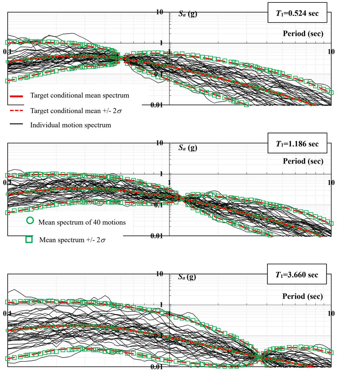
Figure B-4 Spectra of Scaled Motions and Conditional Spectra for Return Period of 43 Years and Period  $T_1$  Equal to 0.524, 1.186 and 3.660 Seconds
