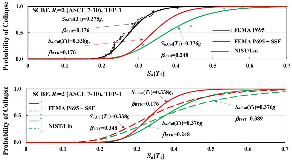
Figure 6-1 Comparison of Fragility Curves for Isolated SCBF, Case  $R_f=2$ , Isolator TFP-1 Obtained by Different Methodologies
