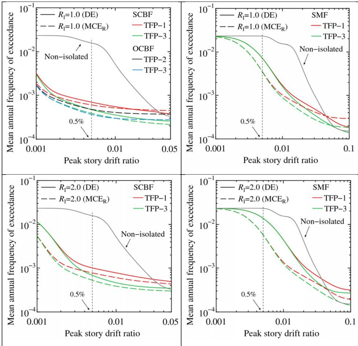
Figure 5-1 Mean Annual Frequency of Exceeding Limits on Peak Story Drift Ratio
