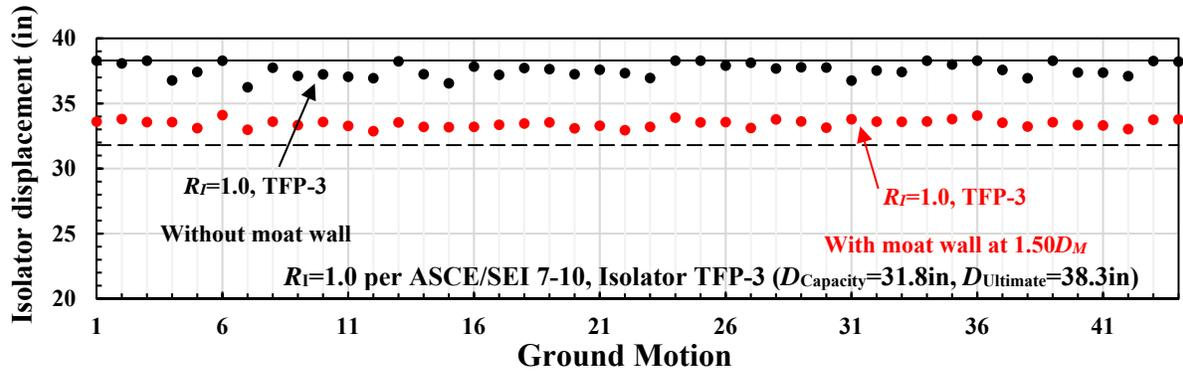
Figure 4-8 Peak Isolator Displacements at Collapse of Buildings with SCBF Designed per ASCE/SEI 7-10, Isolator TFP-3 with and without Moat Wall at Distance 1.5D<sub>M</sub>
