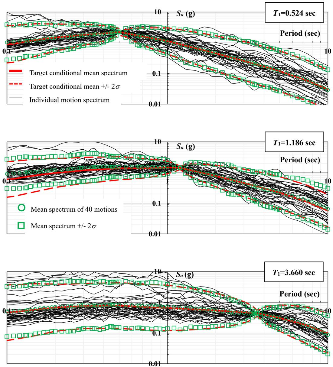
Figure B-11 Spectra of Scaled Motions and Conditional Spectra for Return Period of 3899 Years and Period  $T_1$  Equal to 0.524, 1.186 and 3.660 Seconds
