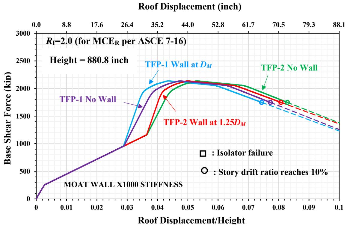
Figure 2-6 Pushover Curves of SMF in Case of Isolators TFP-1 with  $D_{Capacity}=20.4\text{in}$  ( $=D_M$ ) and TFP-2 with  $D_{Capacity}=26.1\text{in}$  ( $=1.25D_M$ ) and Moat Walls Placed at Distances  $D_M$  and  $1.25D_M$
