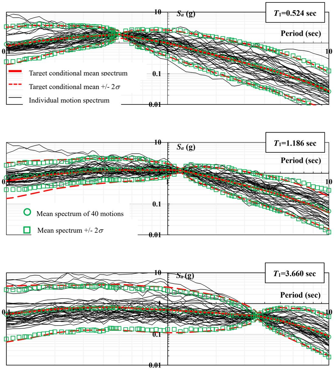
Figure B-10 Spectra of Scaled Motions and Conditional Spectra for Return Period of 2475 Years and Period  $T_1$  Equal to 0.524, 1.186 and 3.660 Seconds
