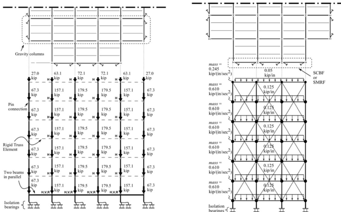
Figure 3-1 Representation of Gravity and Seismic Force-Resisting Frames of Isolated Building
