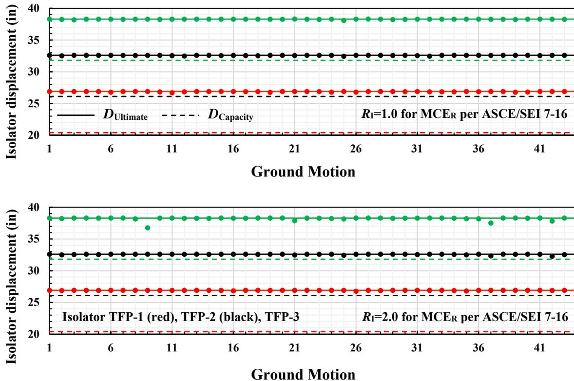
Figure 4-4 Peak Isolator Displacements at Collapse of Buildings with SMF Designed for the MCE<sub>R</sub> per ASCE/SEI 7-16 and without moat walls
