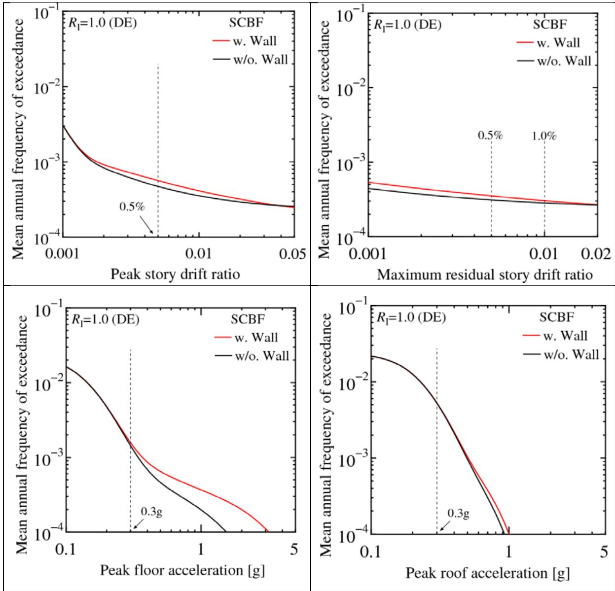
Figure 5-7 Comparisons of Mean Annual Frequency of Exceeding Limits on Drift, Residual Drift and Peak Acceleration for SCBF Designed per ASCE 7-10 for  $R_I=I$ , Isolator TFP-3 without and with Moat Wall at  $1.50D_M$  (design without moat wall meets criteria for continued functionality per Zayas et al, 2017)
