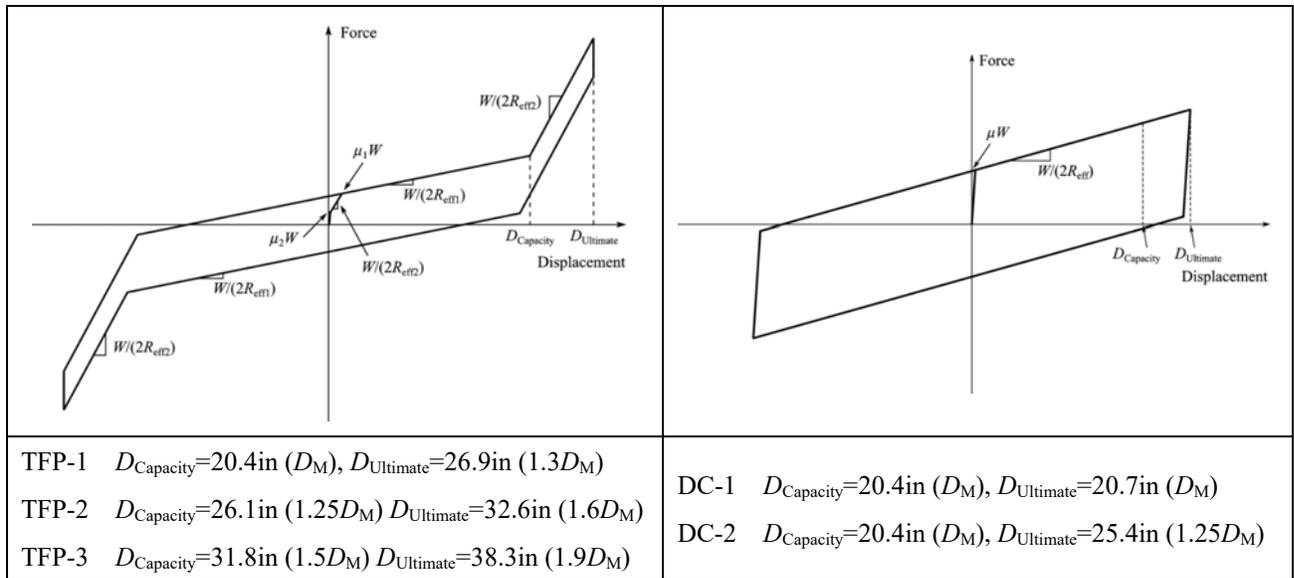
Figure 2-3 Force-Displacement Relationships of Triple FP (Left) and Double Concave (Right) Isolators
