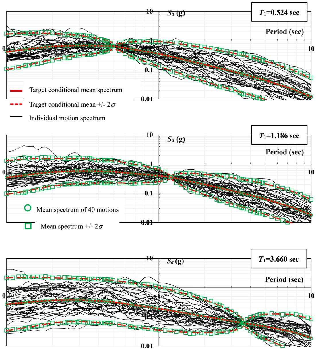
Figure B-5 Spectra of Scaled Motions and Conditional Spectra for Return Period of 144 Years and Period  $T_1$  Equal to 0.524, 1.186 and 3.660 Seconds
