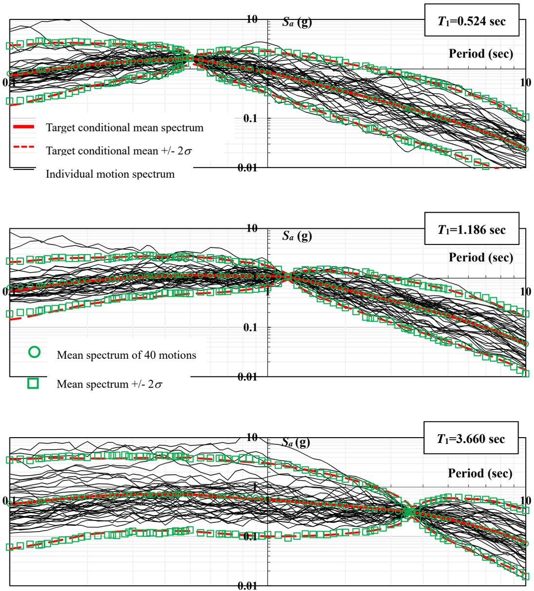
Figure B-9 Spectra of Scaled Motions and Conditional Spectra for Return Period of 1485 Years and Period  $T_1$  Equal to 0.524, 1.186 and 3.660 Seconds
