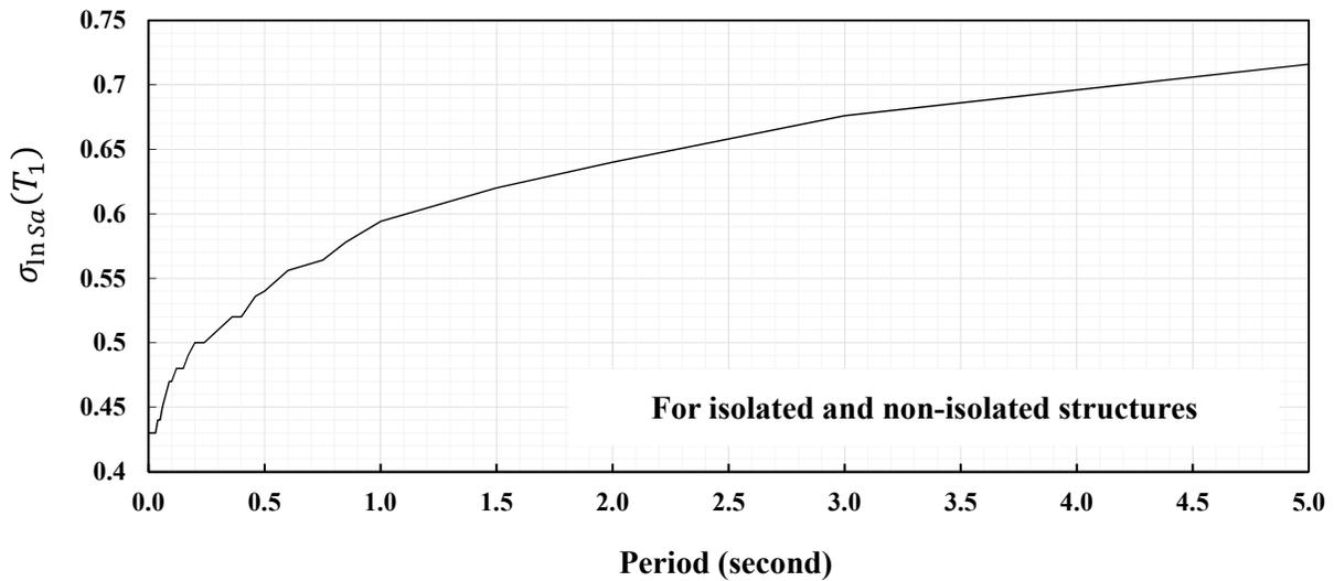
Figure A-2 Standard Deviation of Natural Logarithm of Spectral Acceleration
