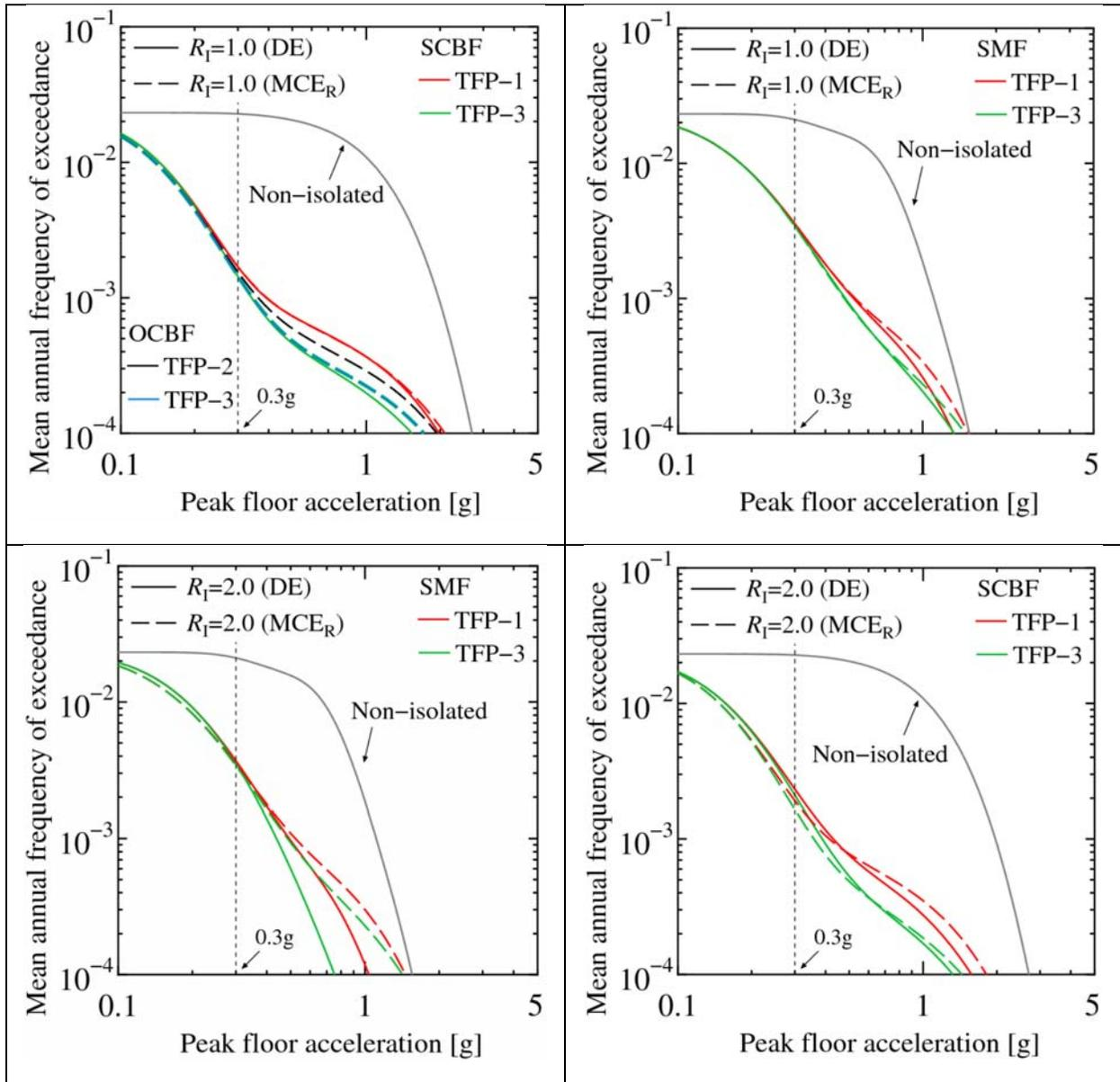
Figure 5-3 Mean Annual Frequency of Exceeding Limits on Floor Acceleration
