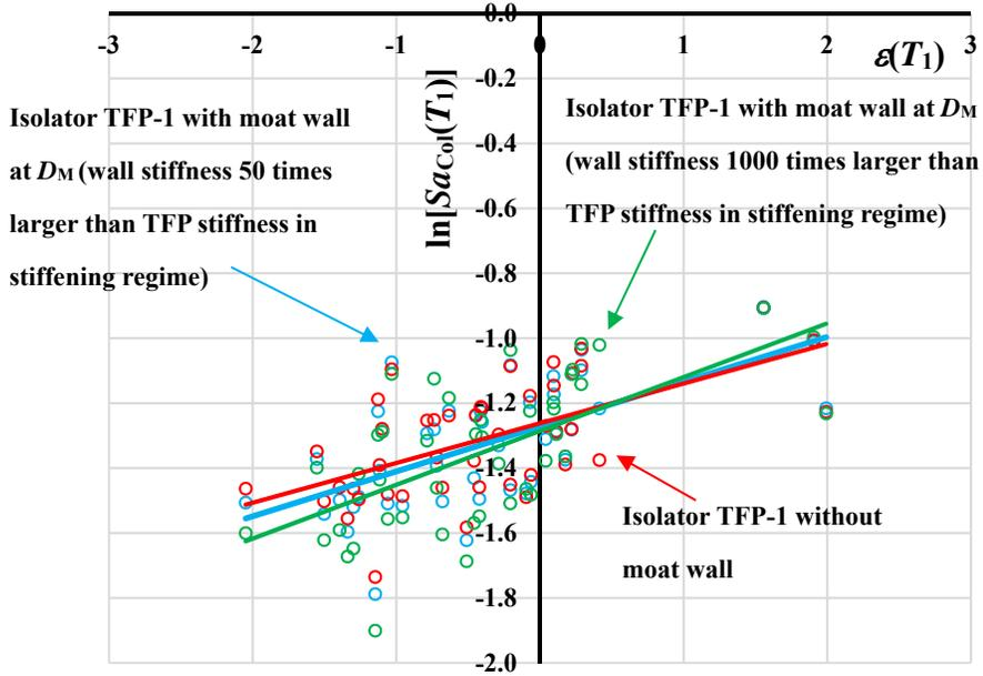
Figure A-5 Relationship between  $\ln[S_{aCOL}(T_1)]$  and  $\varepsilon_j(T_1)$  for Isolated Buildings with SCBF Designed for  $R=2.0$  per ASCE/SEI 7-10 and Isolator TFP-1 ( $D_{Capacity}=20.4\text{in}$ ,  $D_{Ultimate}=26.9\text{inch}$ ) with and without Moat Wall
