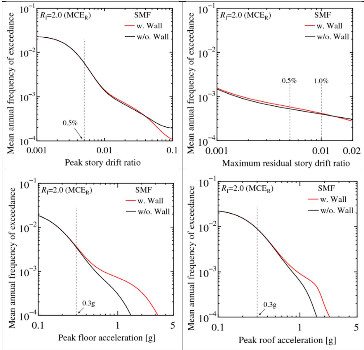
Figure 5-8 Comparisons of Mean Annual Frequency of Exceeding Limits on Drift, Residual Drift and Peak Acceleration for SMF Designed per Minimum Criteria of ASCE 7-16 ( $R=2$ , Isolator TFP-1) without and with Moat Wall at  $D_M$
