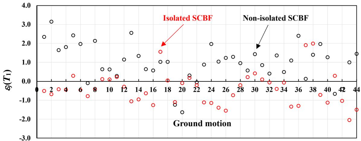
Figure A-3 Calculated Values of  $\varepsilon_j(T_1)$  for Each of 44 Ground Motions (Isolated SCBF:  $R_1=1.0$  (DE), TFP-1)
