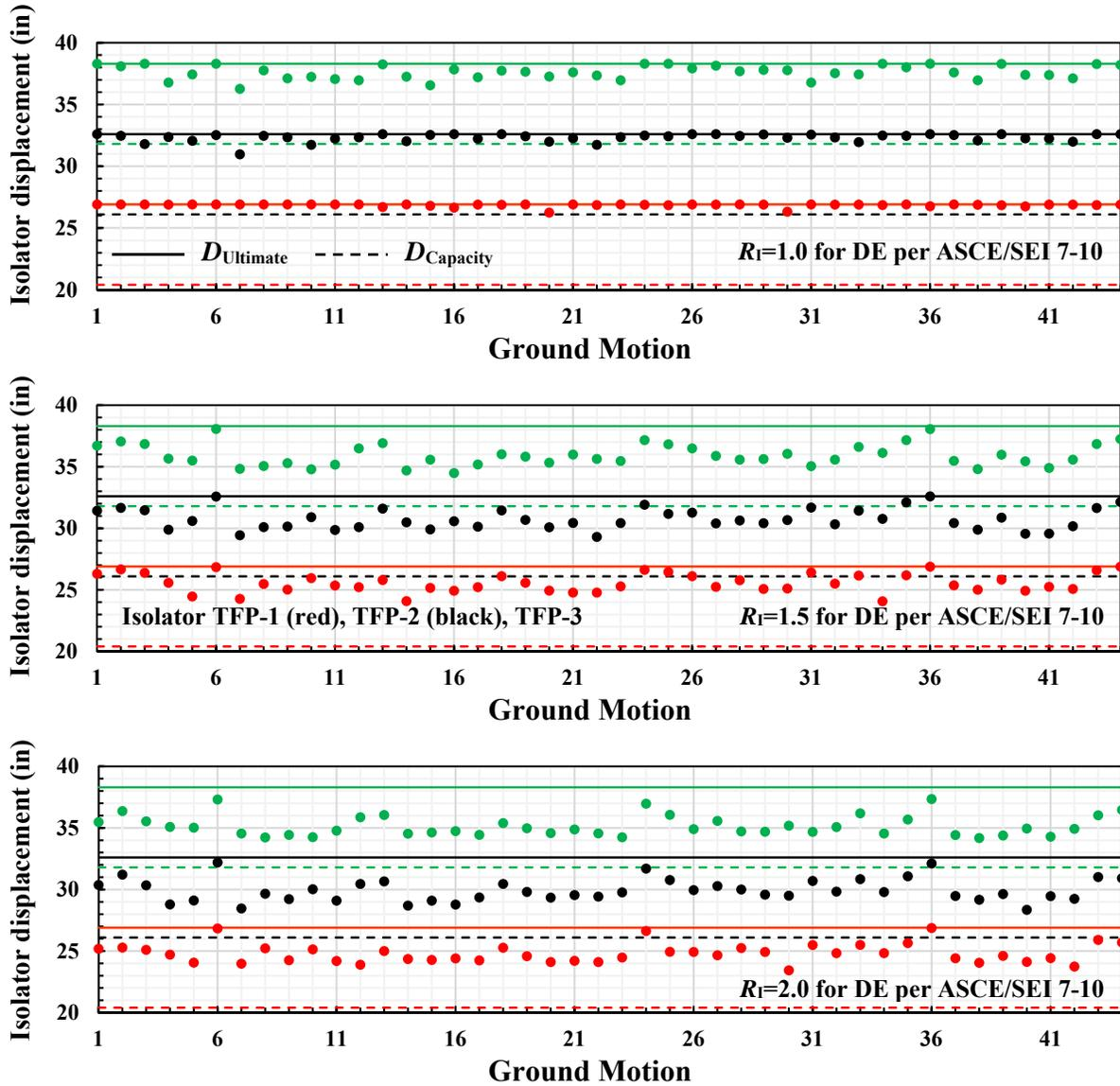
Figure 4-1 Peak Isolator Displacements at Collapse of Buildings with SCBF Designed for the DE per ASCE/SEI 7-10 and without moat walls
