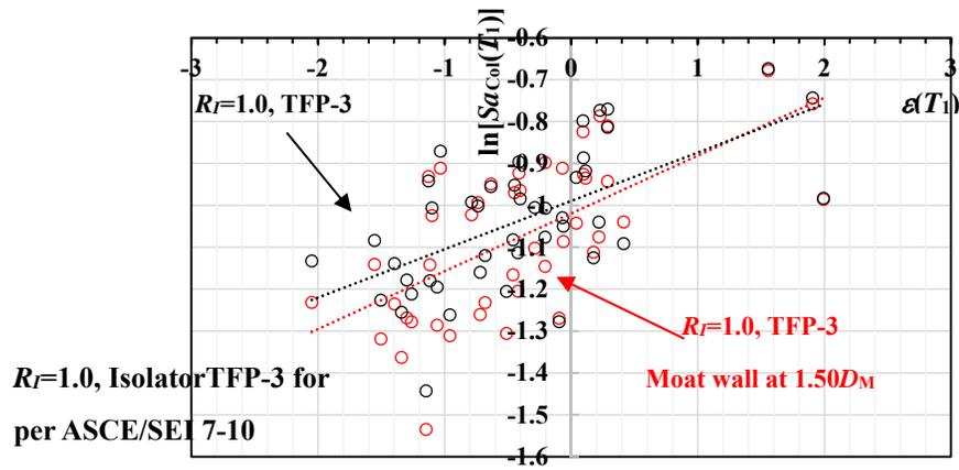
Figure A-7 Relationship between  $\ln[Sa_{Col_j}(T_1)]$  and  $\epsilon_j(T_1)$  for Isolated Buildings with SCBF Designed for  $R=1.0$  per ASCE/SEI 7-10 and Isolator TFP-3 ( $D_{Capacity}=31.8\text{in}$ ,  $D_{Ultimate}=38.3\text{inch}$ ) with and without Moat Wall
