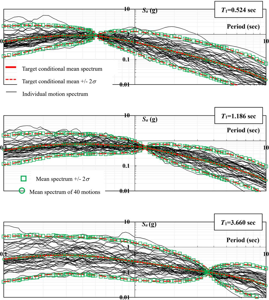
Figure B-6 Spectra of Scaled Motions and Conditional Spectra for Return Period of 289 Years and Period  $T_1$  Equal to 0.524, 1.186 and 3.660 Seconds
