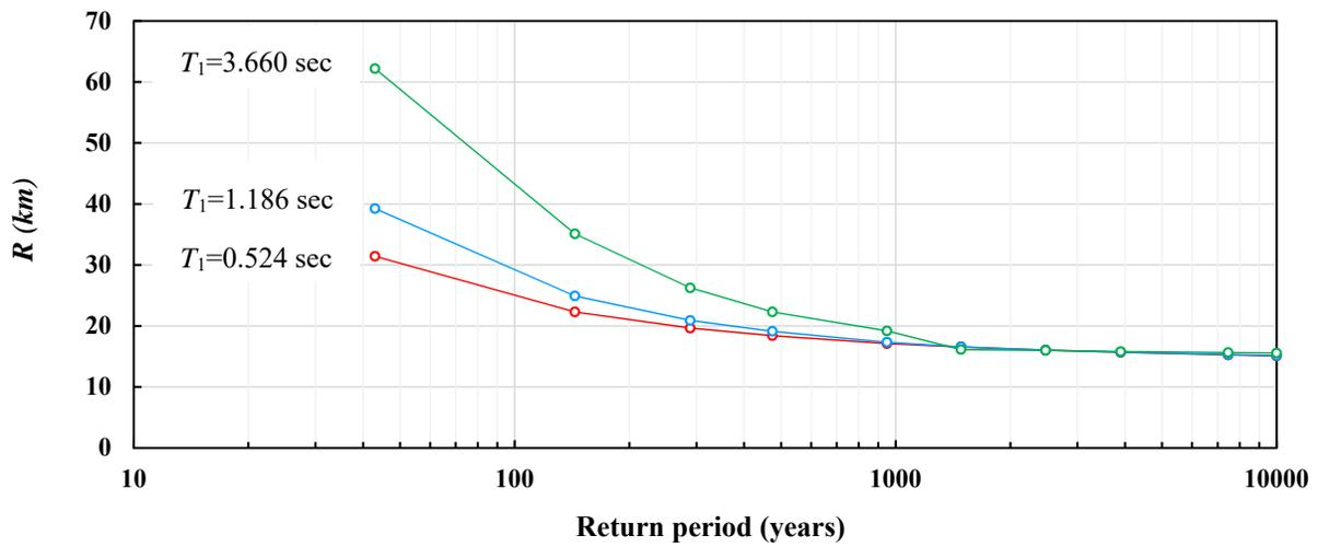
Figure B-2 Mean Causal Earthquake Magnitude  $M$  and Distance  $R$  as Function of Return Period
