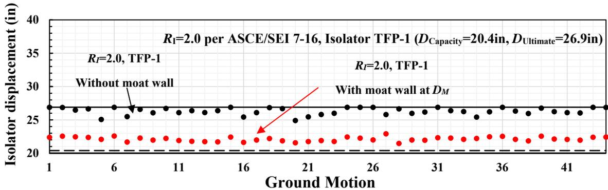
Figure 4-7 Peak Isolator Displacements at Collapse of Buildings with SCBF Designed per ASCE/SEI 7-16, Isolator TFP-1 with and without Moat Wall at Distance  $D_M$
