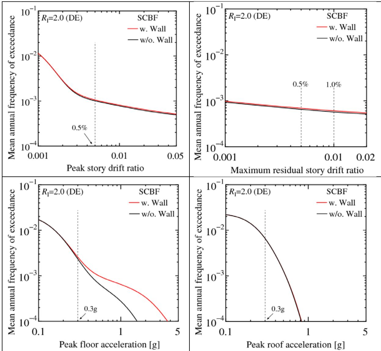
Figure 5-5 Comparisons of Mean Annual Frequency of Exceeding Limits on Drift, Residual Drift and Peak Acceleration for SCBF Designed per Minimum Criteria of ASCE 7-10 ( $R_1=2$ , Isolator TFP-1) without and with Moat Wall at  $D_M$
