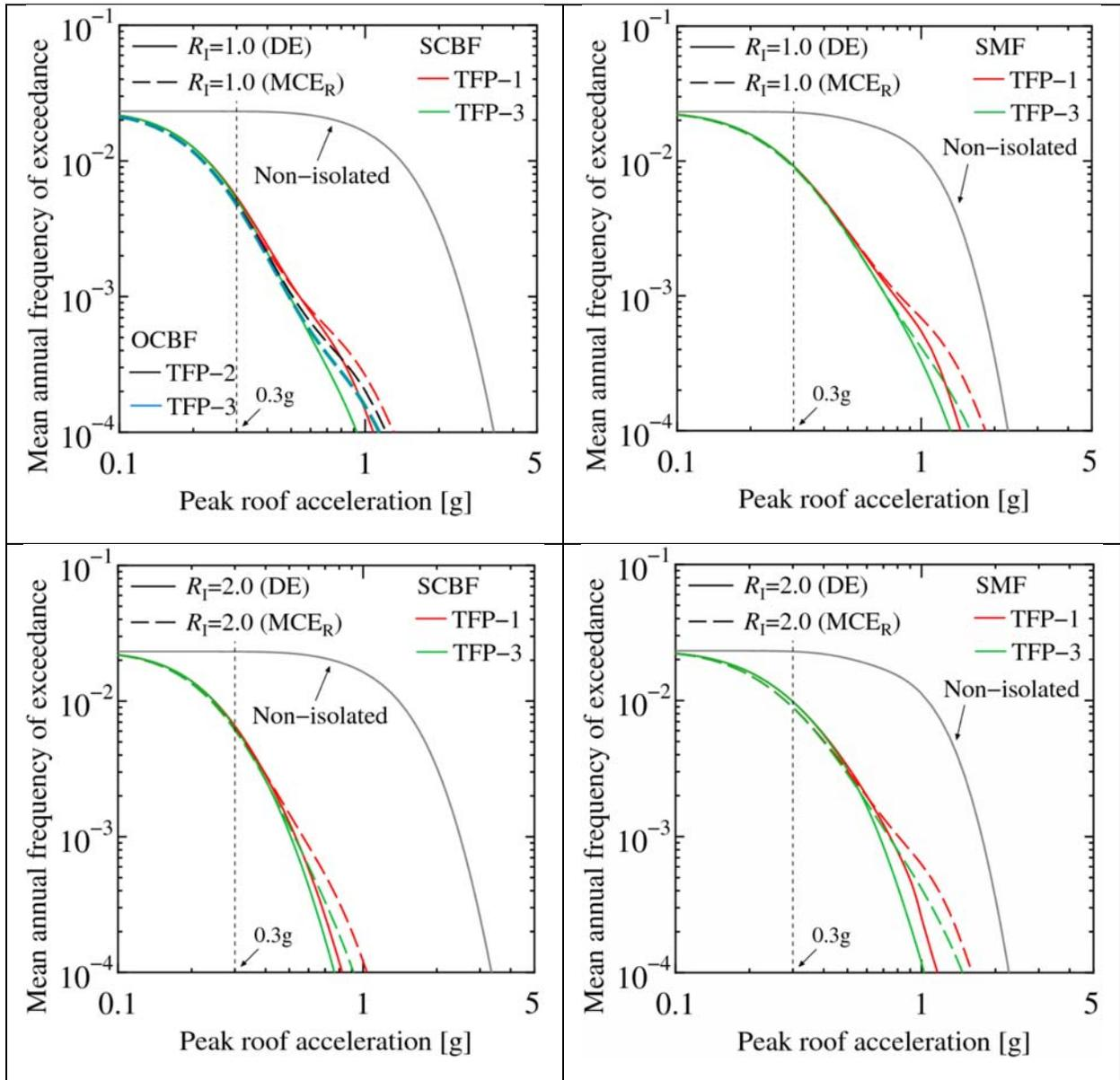
Figure 5-4 Mean Annual Frequency of Exceeding Limits on Roof Acceleration
