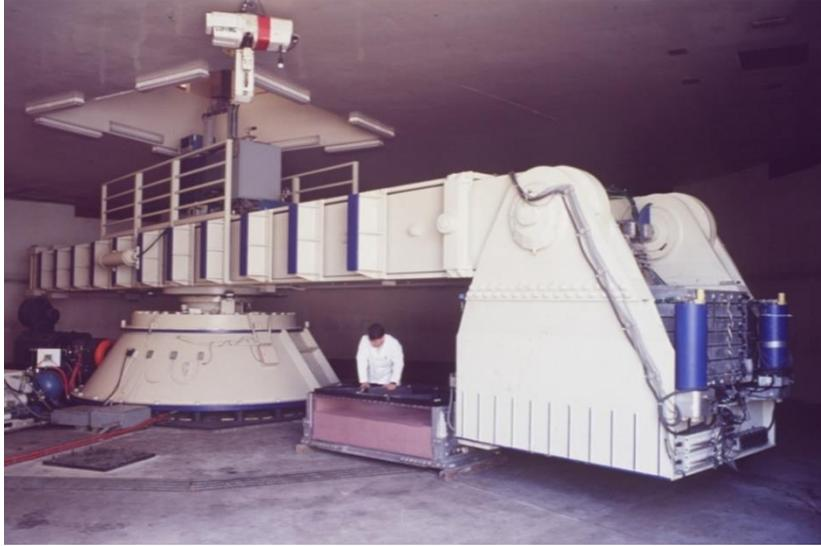
a. Photograph of the UC Davis Geotechnical Centrifuge showing the horizontal arm, the swing bucket, and the laminar box
