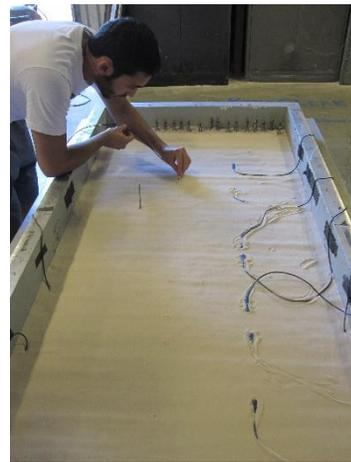
d. Laminar box right after pluviation
