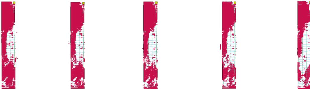
(b) Zero axial pressure, damage function
