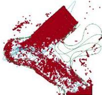
(h) Axial pressure:  $0.4 f'_c$ , damage function
