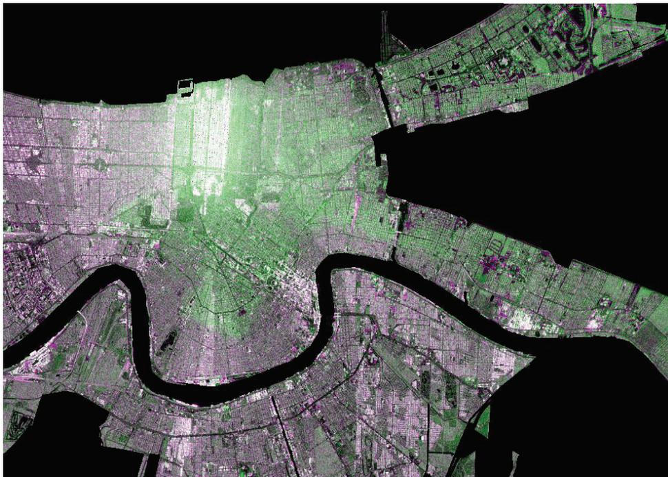
**Figure 2-4. Urban flood signature in New Orleans detected after hurricane Katrina using fine beam mode Radarsat I imagery. A false color composite was produced where red = non-flood (13th April 2006), green = flood (9th September 2005), and blue = non-flood.**
