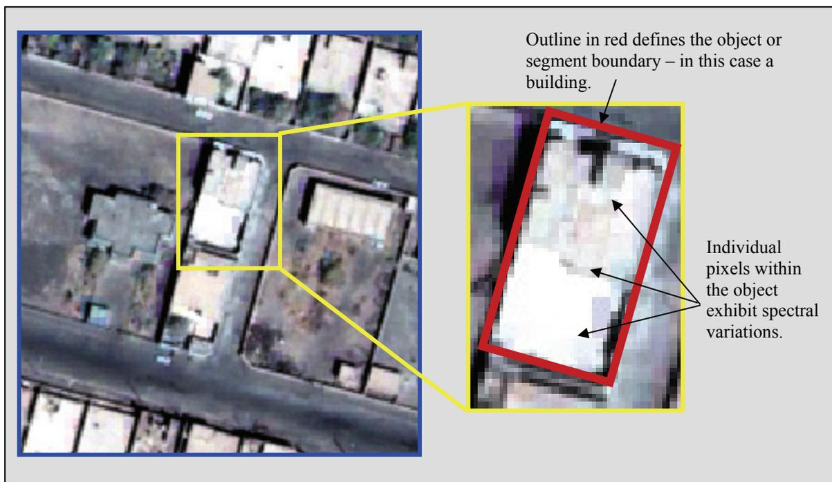
**Figure 2-3 For Object-Based Analysis the Basic Processing Unit is a Segment – in this Case a Building. Traditional Image Processing Techniques Instead Analyze Individual Pixels, which may Exhibit Considerable Variability within a given Object.**
