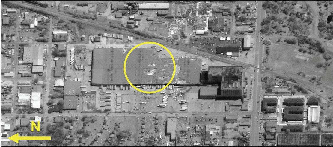
**Figure 2-7. IKONOS Panchromatic Image with Sufficiently Fine Spatial Resolution (1 m) to Observe Building Damage from the March 28, 2000, Ft. Worth, TX Tornado. This Image was Acquired March 29, 2000, the Morning Following the Tornado. In Addition to Roof Damage, the Image Shows Damaged and Scattered Semi-Trucks in the Parking Lot. Credit: GeoEye and Mulligan (2003).**
