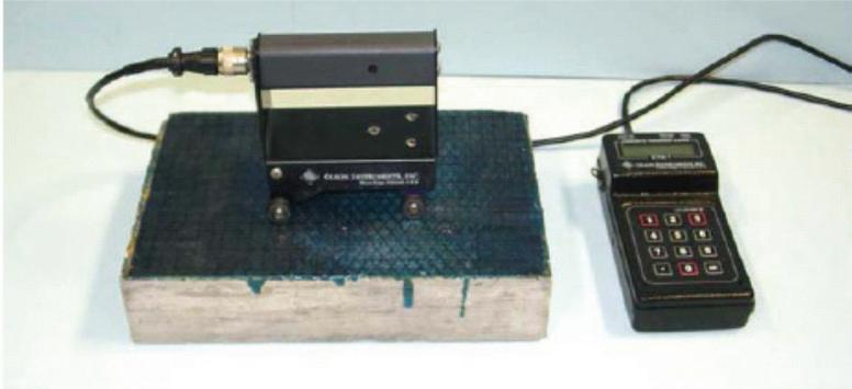
**Figure 4-15. Olson Instruments Impact-Echo Tester**
