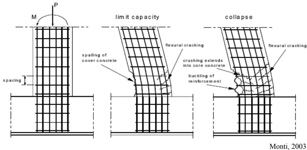
**Figure 2-8. Lateral Collapse Mechanism of an Under-designed Column without FRP Jacketing**
