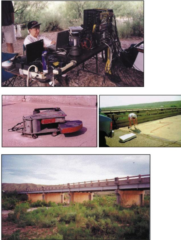
**Figure 3-5. Health Monitoring and Damage Detection for Alamosa Canyon and I-40 Bridges Carried out by Los Alamos National Laboratory**
