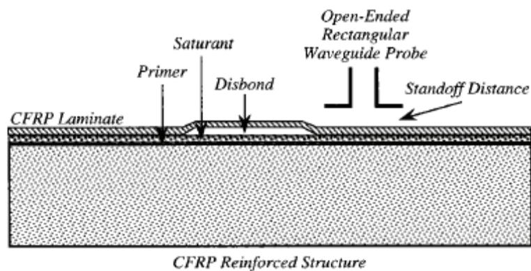
**Figure 4-5. Schematic of Microwave Measurement Approach**
