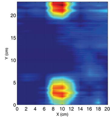
(b) Scanned Area on FRP-Wrapped Concrete (c) Real-Time Image Indicating Debonds
