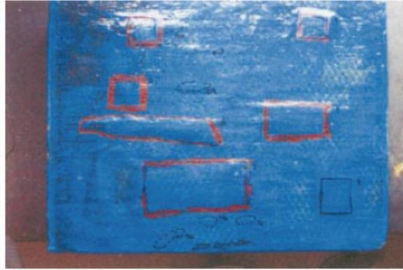
**Figure 4-6. Top View of Carbon Fiber Reinforced Polymer Laminate Adhered to Mortar Substrate (Sample) with Disbonded Regions Produced by Injecting Air in between Laminate and Substrate**
