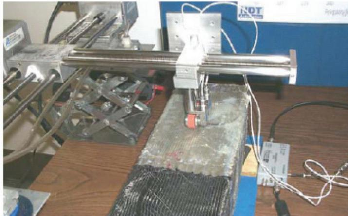
**Figure 4-18. Inspection of a FRP-Concrete Sample Using Rolling Sensors Mounted on a Scanning Bridge**
