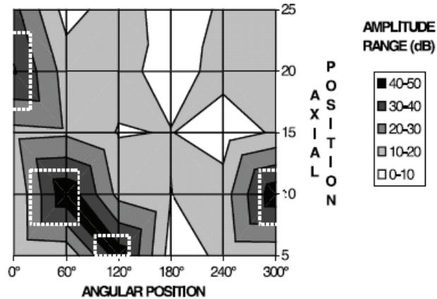
**Figure 4-12. Amplitude Map of the First Echo on a Concrete Cylindrical Specimen Wrapped with CFRP. The High-Echo-Amplitude Areas (Dark Spots) Locate the Artificial Bonding Defects (Dashed Line)**
