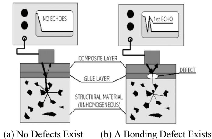
**Figure 4-10. High Frequency Ultrasonic Tests on External Composites Strengthening Applied to Concrete**
