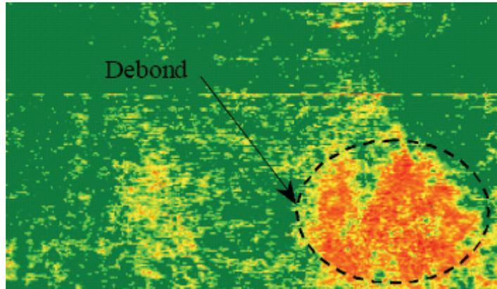
**Figure 4-22. C-Scan Image of an FRP/Concrete Sample showing a Debond between the FRP and Concrete**
