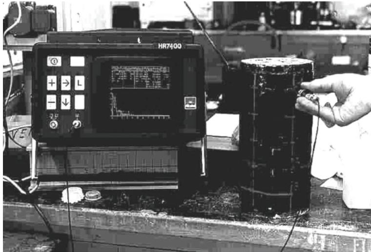
**Figure 4-11. Experimental Setup for Ultrasonic Testing of Concrete Cylinder Wrapped with CFRP**
