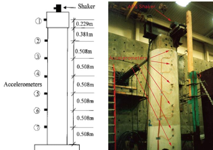
**Figure 4-2. Locations of Accelerometers and Shaker for Glass Fiber-Jacketed Column Test**
