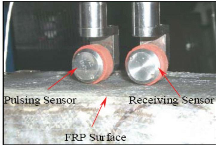
**Figure 4-19. Detail of the Rolling Sensors During Inspection of an FRP/Concrete Sample**
