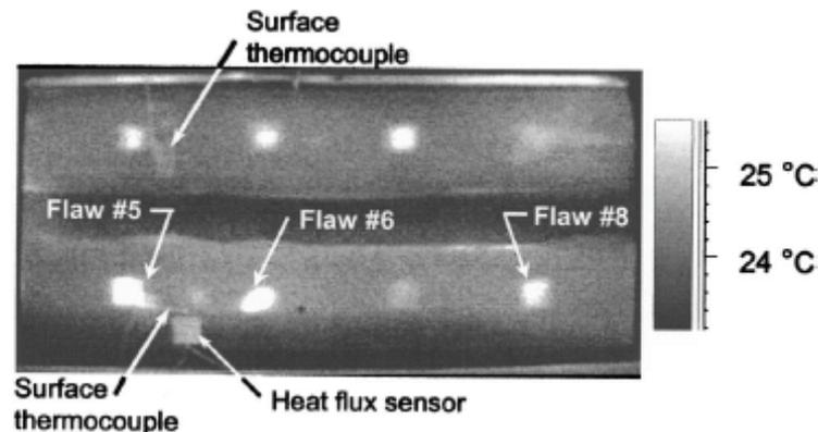
**Figure 4-8. Thermogram of Test Object During Qualitative Detection of Simulated Subsurface Flaws**
