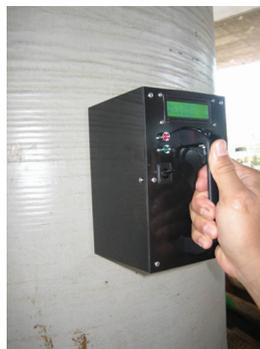
**Figure 4-3. Hand-Held Debond Detector for Inspection of FRP-Wrapped Concrete Structure**
