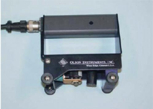
**Figure 4-16. Impact-Echo Tester Modified with Air Coupled Receiver**
