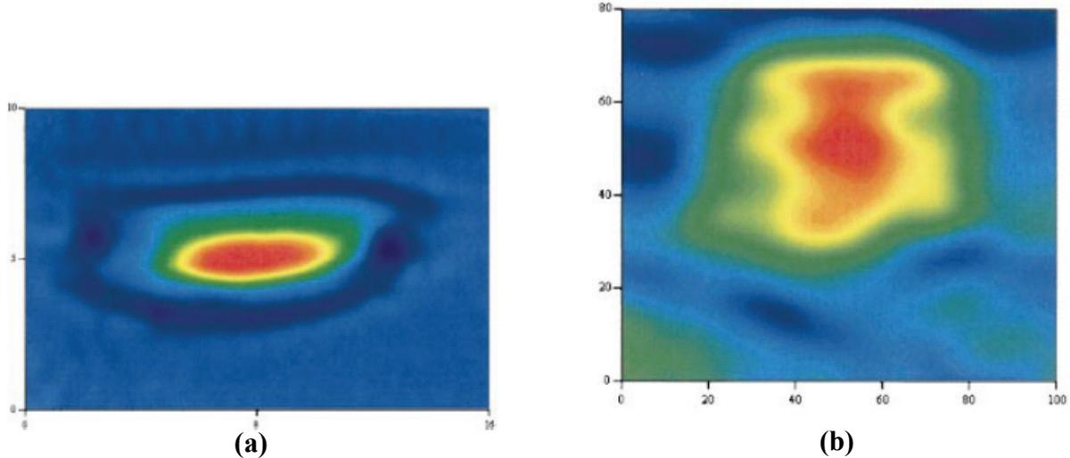
**Figure 4-7. (a) Microwave Image of Disbond at Frequency of 24 GHz and Standoff Distance of 7 mm; (b) Microwave Image of Square-shaped Disbond at Frequency of 10 GHz and Standoff Distance of 1.5 mm using Orthogonal Polarization (dimensions in millimeters)**
