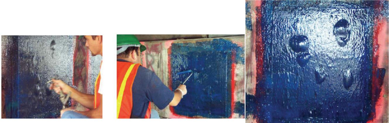
**Figure 4-14. “Forced” Creation of Delaminations by Air Injection**
