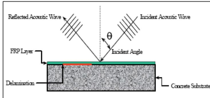
**Figure 4-17. Setup Used for the Theoretical Simulation of Wave Propagation on FRP-Concrete Structures**
