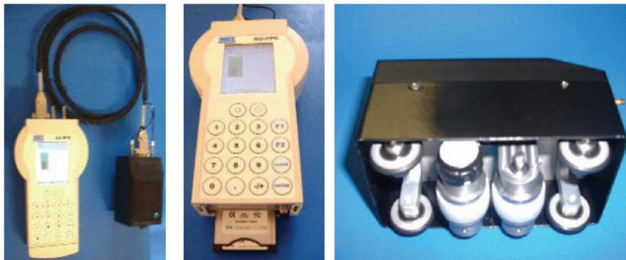
**Figure 4-20. Inspection System for Composite Wrap Inspection on Concrete Structures**
