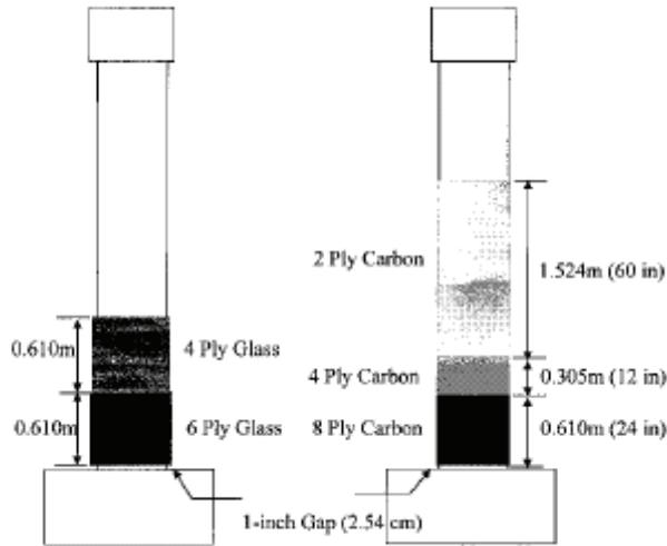
**Figure 4-1. Jackets for Test Columns**
