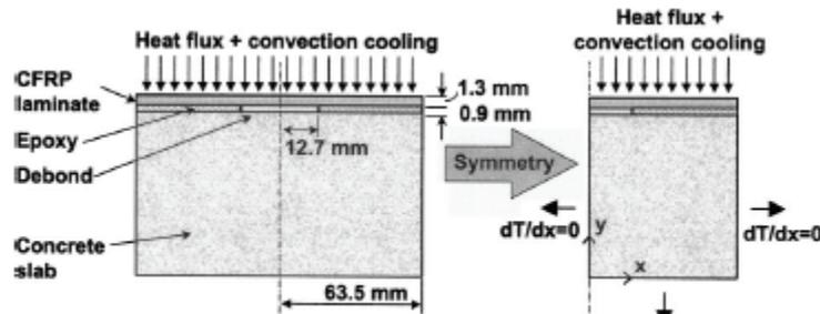
Figure 4-9. Test Object Used in Finite-element Simulations
