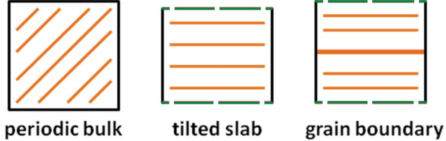
**Figure 2-8** The three systems considered in excess potential energy calculations of a grain boundary. Orange lines are Miller planes; Green dashed lines are fixed free surfaces.
