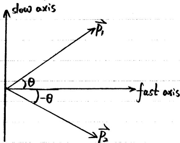
That means the transmitted light is rotated by an angle  $2\theta$ .
