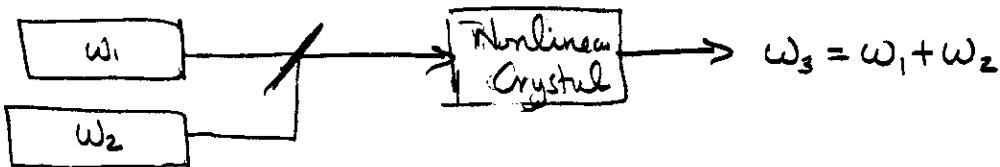
Notice: Although the incident waves at  $\omega_1$  &  $\omega_2$  produce polarization densities at  $0, 2\omega_1, 2\omega_2, \omega_1 + \omega_2$  and  $\omega_1 - \omega_2$ , all waves not necessarily generated.
