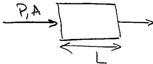
$$\begin{aligned} \phi &= \frac{2\pi n(I)L}{\lambda_0} \\ &= 2\pi(n + n_2 \frac{P}{A}) \frac{L}{\lambda_0}. \end{aligned}$$
