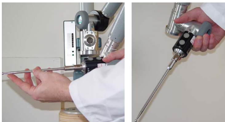
Fig. 1. The electromechanical arm used in this study had six degrees of freedom, a working radius of 2 m and accuracy of 0.3 mm. The probe tip is shown here.
