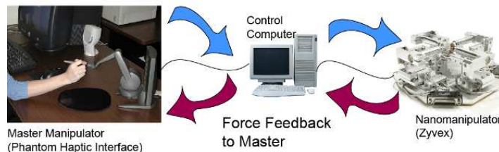
Nanomanipulation with vision-based force sensing and feedback
