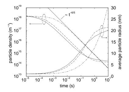
Fig. 2: Particle number density and average radius during coagulation. The full lines denote particle charging including UV photo-detachment, the dashed lines with reduced photo-detachment. The dash-dotted lines show the behavior of a neutral aerosol.
