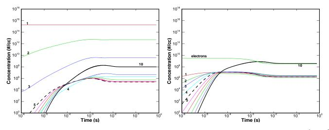
Fig. 1: Clustering of neutral silicon hydrides (left) and anionic silicon hydrides (right) for  $n_i = 3 \times 10^9$  cm<sup>-3</sup> and 100 mTorr and a gas temperature of 500 K. The numbers at the curves denote the number of Si atoms per cluster.
