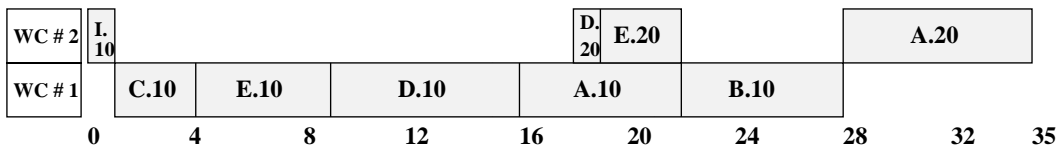
Figure 5: Gantt Chart of the Optimal Schedule for the example given in Figure 1 (without transportation operations)
