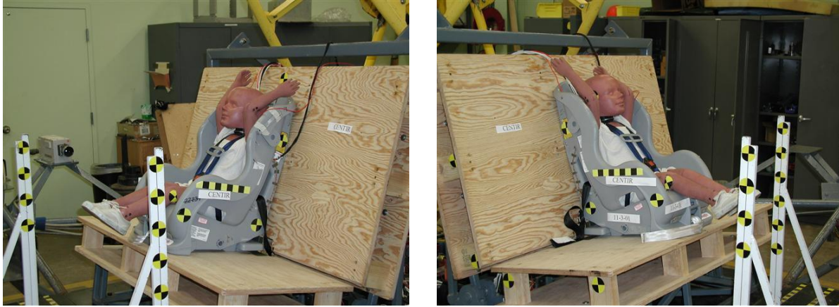
(a) North side (b) South side Figure 11. CRS and dummy appearance immediately after a typical sled test.
