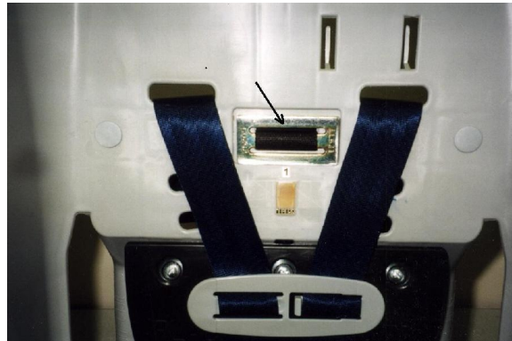
Figure 6. Tether strap mounting location on the CRS shell.
