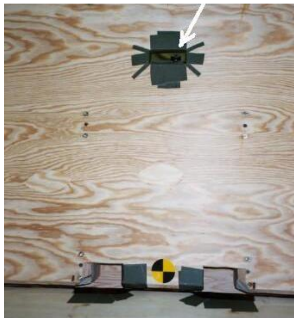
Figure 7. Test bench back assembly showing notch made to accommodate the tether strap.
