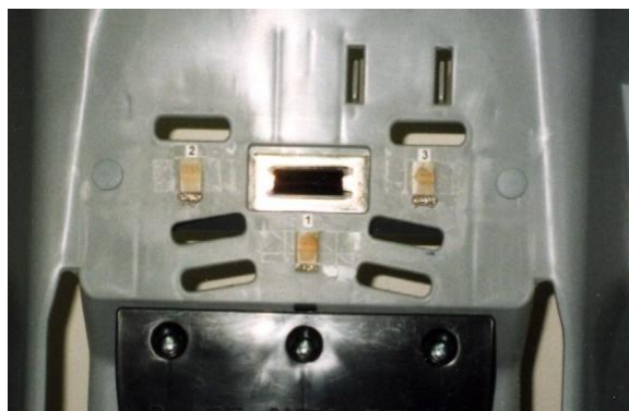
Figure 15. Strains were also measured at locations 2 and 3, beneath slots that permit harness strap passage.
