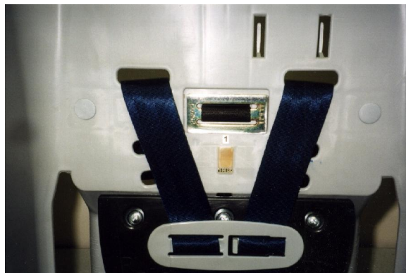
Figure 14. Strain gage rosette 1 was installed below the tether belt anchorage location.
