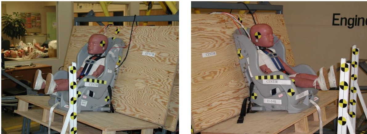
(a) North side of sled track (b) South side of sled track Figure 1. CRS and dummy appearance immediately before a typical sled test.
