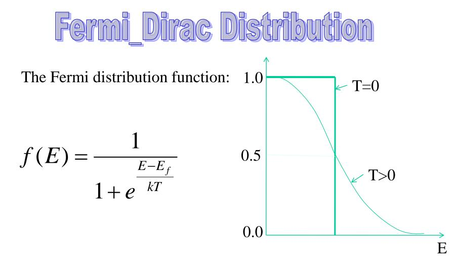
where, E is the electron energy,  $E_f$  is the Fermi energy, and T is the absolute temperature. Its physical meaning is that: f(E) is the probability of occupancy for an electron energy state at energy E by an electron
