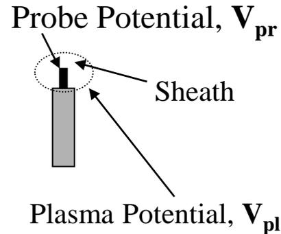
$$I_{\text{Probe}} = I_e^* - I_i^* \exp\left(\frac{-e(V_{pr} - V_{pl})}{kT}\right)$$
