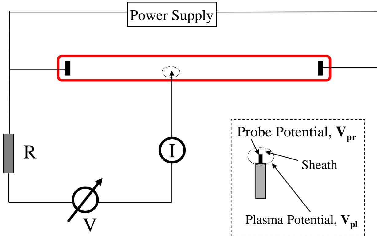
When we place a probe in plasmas, a “sheath” is around the probe formed. The potential drop across the sheath is needed to measure plasma potential.
