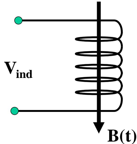
$$V_{ind} = kN \frac{d\Phi}{dt}$$
