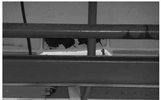
(e) Residual shear deformations of EBF link
