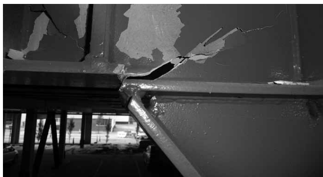
(c) Fractured link at lower level EBF
