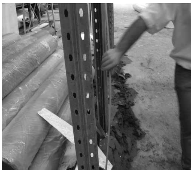
(b) Close-up of buckled brace
