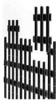
a. three-column module used in the construction of Tower 2 (adapted from Hart et al., 1978)
