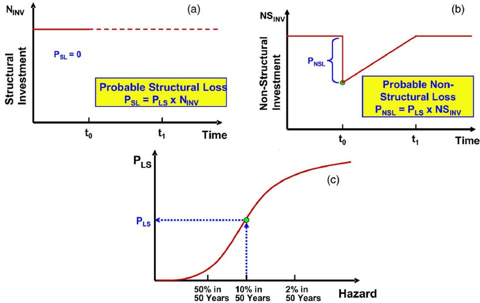
**Figure 10.** Probable nonstructural loss in case of linear-elastic structural response: (a) structural resilience curve; (b) nonstructural resilience curve; and (c) probability of exceeding limit state.
