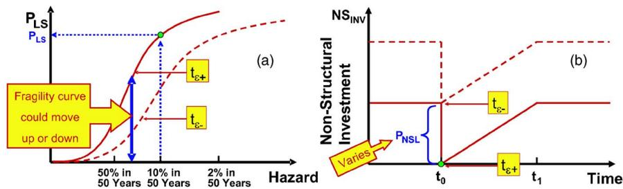
**Figure 14.** Case of nonlinear structural seismic response: (a) probability of nonstructural losses, and (b) corresponding shifts in nonstructural seismic resilience curve.
