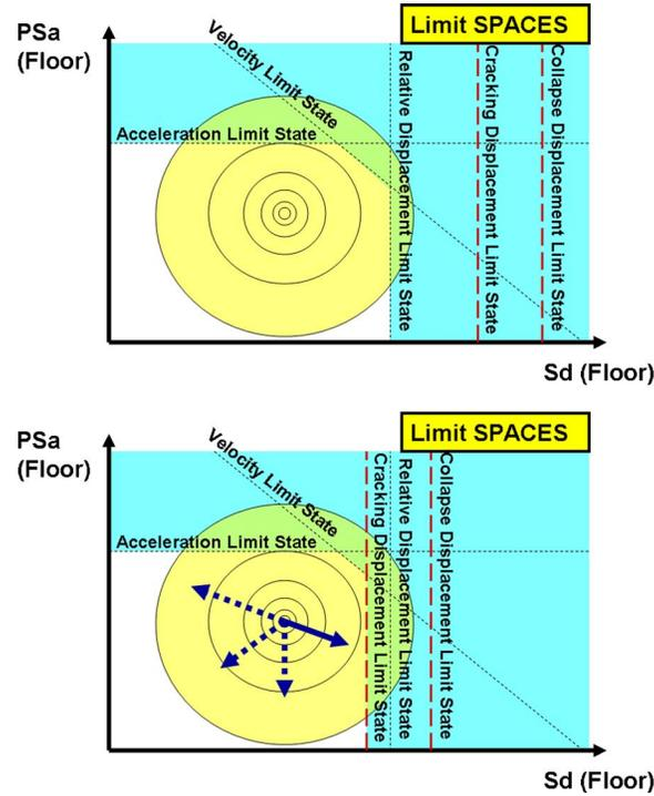
**Figure 8.** Probability that response exceeds limit space: (a) nonstructural limit states reached prior to structural limit states; and (b) different sequence of limit states.
