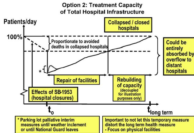
**Figure 5.** Quantification of seismic resilience of acute care facilities as patients/day treatment capacity of the total available hospital infrastructure.
