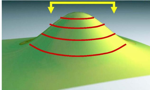
**Figure 7.** Definition of point of view and isoprobability contours of two-dimensional bell curve.
