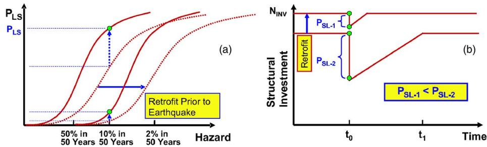
**Figure 13.** Case of nonlinear structural seismic response: (a) Bruneau/Reinhorn assumption of sliding proportional fragility curve sets; and (b) enhancement of resilience curve consequently to reduced probability of losses due to seismic retrofit prior to earthquake.
