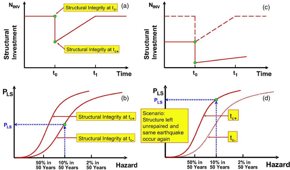
**Figure 11.** Case of nonlinear structural seismic response: (a) structural resilience curve and corresponding loss in structural integrity; (b) probability of structural loss before earthquake; (c) new structural resilience curve if structure left unrepaired; and (d) probability of failure upon repeat of earthquake.
