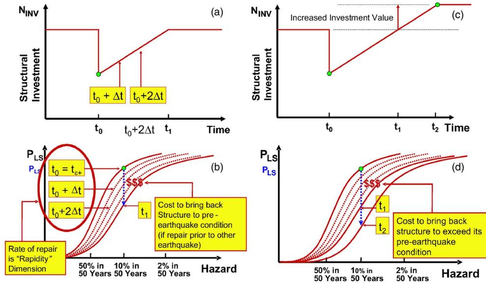
**Figure 12.** Case of nonlinear structural seismic response: (a) improvement in structural resilience as structure is repaired over time; (b) corresponding reduction in probability of structural losses; (c) increased resiliency to above pre-earthquake condition; and (d) corresponding improvement in probability of structural losses.
