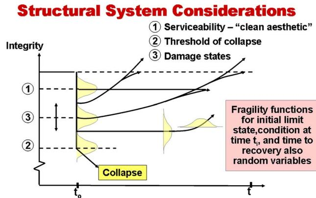
**Figure 6.** Probabilistic aspect of seismic resilience (structural integrity example).
