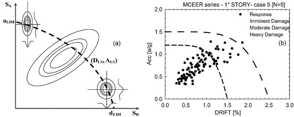
**Figure 9.** Response function and limit states in actual building: (a) response and limit state distributions, and (b) actual data.
