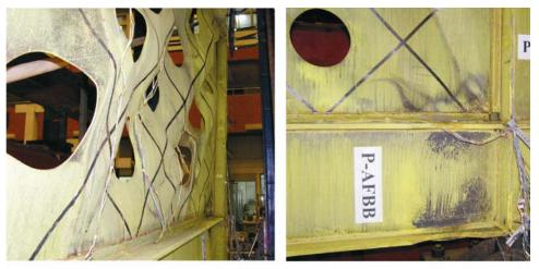
Buckled Panel Following Test RBS Yielding Figure 9 - Buckled panel and RBS yielding of SPW specimen<sup>34</sup>
