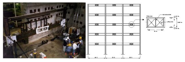
Figure 3 - Frame modified with mid-span truss opening<sup>14</sup>
