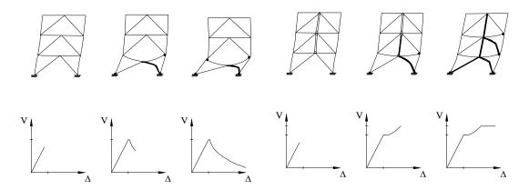
Figure 7 - Push-over curves for inverted-v-braced frames and suspended zipper frames (Roberto Leon, Georgia Tech, Personal Communication, 2004)
