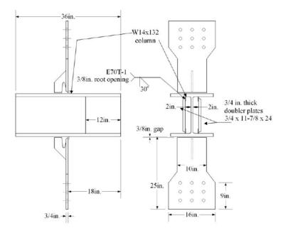
Figure 2: Detail with doubler plates welded to column flange away from web<sup>8</sup>
