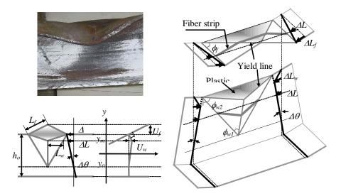
Figure 10 - Yield line plastic hinge model of local buckling<sup>35</sup>
