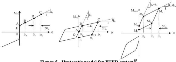
Figure 5 - Hysteretic model for PTED system<sup>15</sup>
