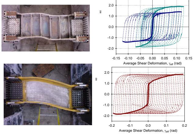
Figure 11 - Deformation near end of test cyclic test results for shear links with high performance steel (top) and low-yield steel (bottom)<sup>37</sup>
