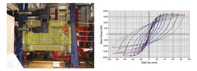
Figure 8 - SPSW specimen with cutout corners (right) and typical hysteresis loops solid wall specimen<sup>34</sup>
