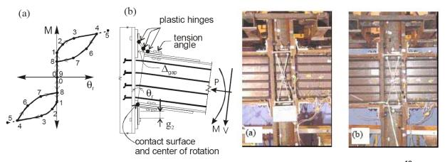
Figure 6 - Post-tension moment connection with top and bottom seat angles<sup>19</sup>
