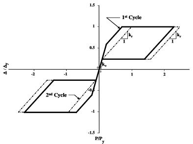
Figure 15 - Hysteretic behavior of rocking truss pier<sup>40</sup>
