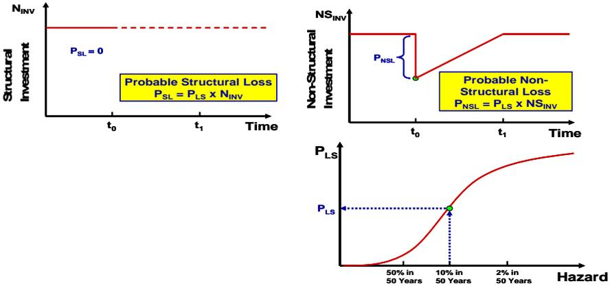
Figure 6: Probable non-structural loss in case of linear-elastic structural response
