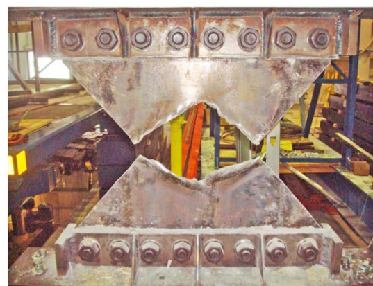
Fig. 13. (a) Link shear versus total rotation hysteretic curve for restrained specimen; (b) link condition after testing
