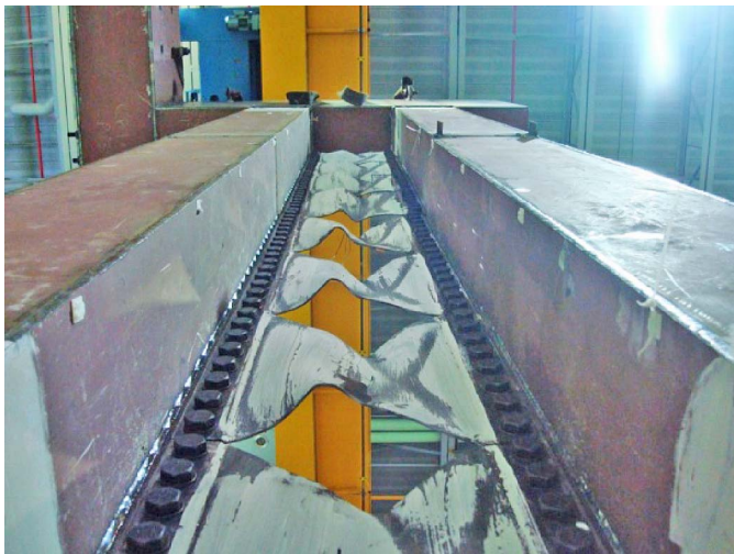
Fig. 7. SPSL's yielding at 1.6% drift
