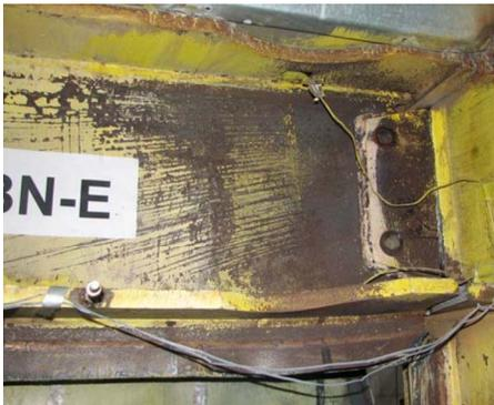
**Fig. 15.** Web of the intermediate HBE of SPSW at the end of testing (Qu et al. 2008)
