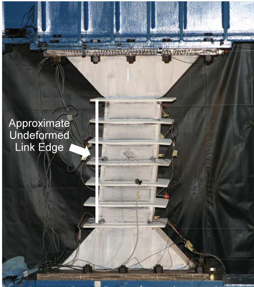
Fig. 9. Specimen X2L1.2 deformed at 0.09 rad
