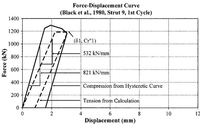
Fig. 15. Hysteretic energy ratio from the first cycle of strut 9 [based on data from Black et al. (1980)]
