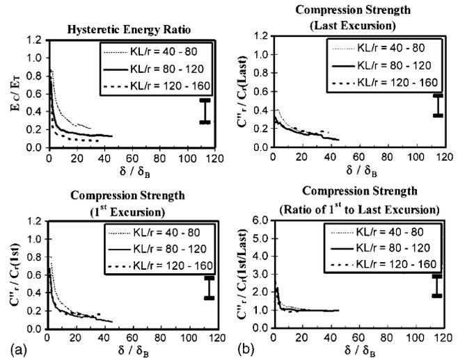
Fig. 13. Averages of data by  $KL/r$  value ranges for wide flange section
