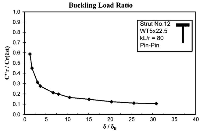
Fig. 6. Example of normalized maximum compression strength reached upon repeated cycling data,  $C''_r/C_r(\text{first})$
