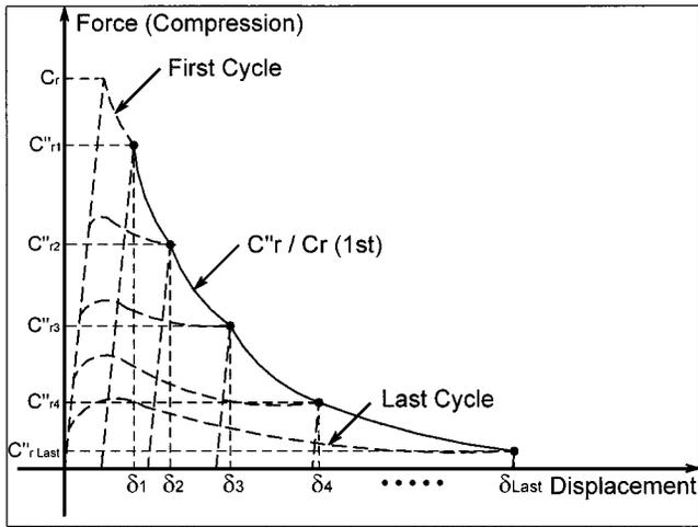
Fig. 4. Definition of normalized buckling capacity,  $C''_r/C_r$  (first)
