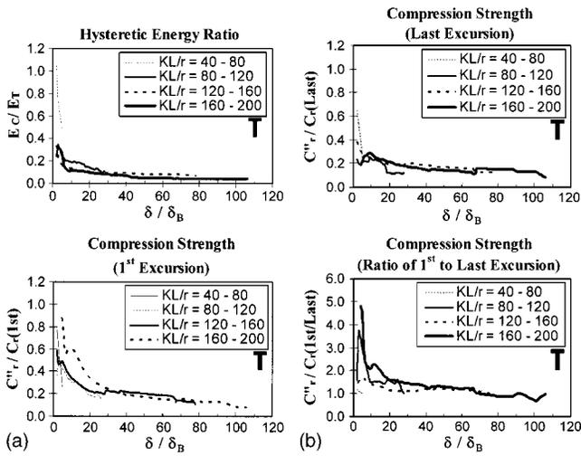
Fig. 14. Averages of data by  $KL/r$  value ranges for double angles, back-to-back
