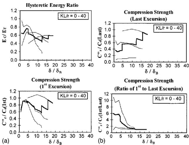
Fig. 10. All structural shapes with  $KL/r=0-40$  (average shown by thicker line)
