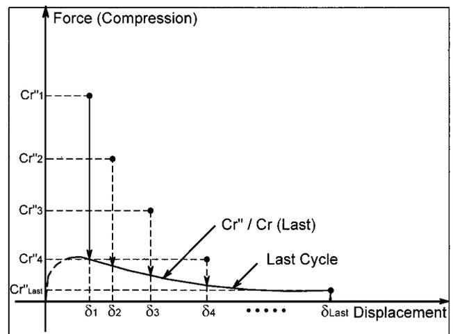
Fig. 7. Definition of normalized buckling capacity,  $C''_r/C_r(\text{last})$
