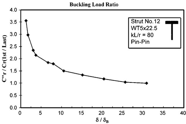
Fig. 9. Example of normalized maximum compression strength reached upon repeated cycling data,  $C''_r/C_r(\text{first/last})$
