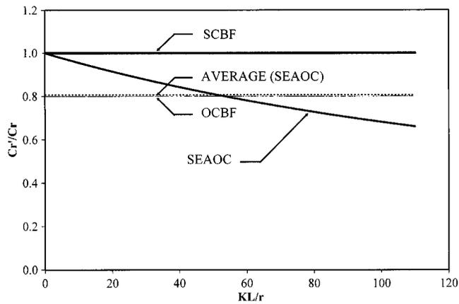
**Fig. 1.** Normalized codified equations of reduced buckling strength due to inelastic cyclic loading
