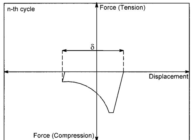
**Fig. 3.** Definition of axial displacement,  $\delta$
