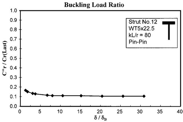
Fig. 8. Example of normalized maximum compression strength reached upon repeated cycling data,  $C''_r/C_r(\text{last})$
