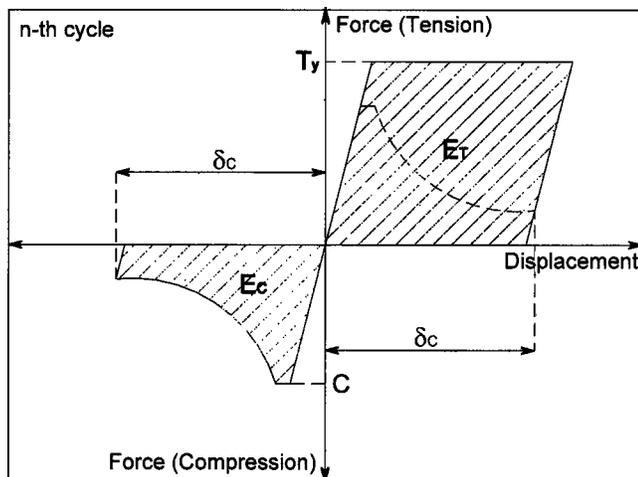
**Fig. 2.** Definition of dissipated energy ratio,  $E_c/E_T$
