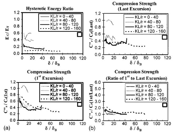
Fig. 12. Averages of data by  $KL/r$  value ranges for tubular sections
