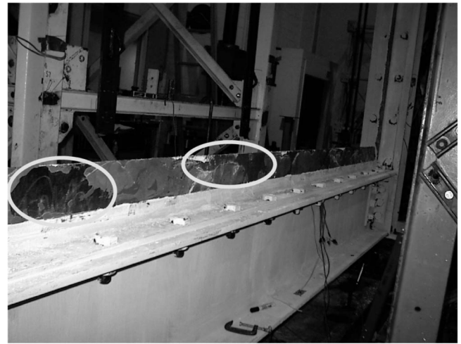
Fig. 9. Poor epoxy coverage (Specimen F1)
