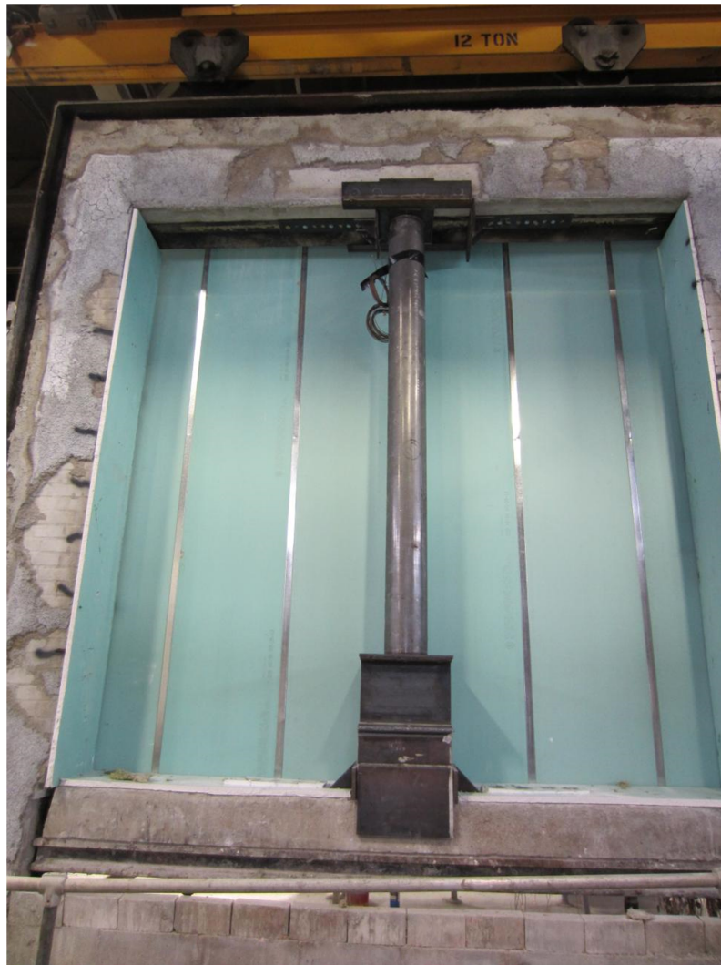
Figure 7. Specimen S3 installed in the vertical furnace
