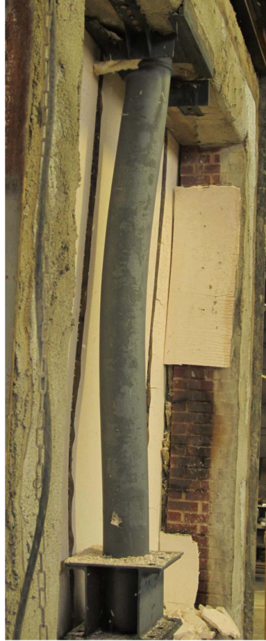
Figure 10. Final state of specimen S3 at the end of the fire test
