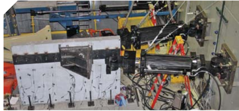
Figure 1: Squat wall testing at UB NEES Lab
