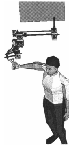
Fig. 2 Potential use of a passive manipulation assist device based on the SDCSC configuration to form a “virtual reconfigurable manipulation guide-rail” in an industrial setting
