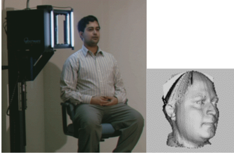
Figure 4: Geometric information of a human head obtained by a Cyberware 3030PS scanner. The information is obtained by scanning the head from different angles and registering the different images. The information of the chin is used to make the customized prototype in Figure 5.
