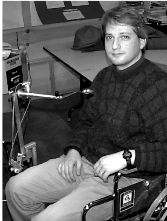
Figure 3. An articulated mechanism for feeding in a foot-controlled feeding device (Magpie) designed at the Nuffield Orthopaedic Center in Oxford, England (75).
