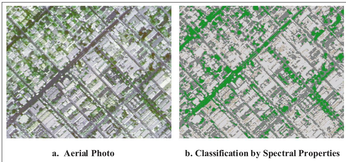
■ Figure 4. Classification of Building Shapes based on Multi-Spectral Analysis of Aerial Photographs
