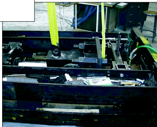
■ Figure 5. Loading Frame Sitting on Laboratory Floor
