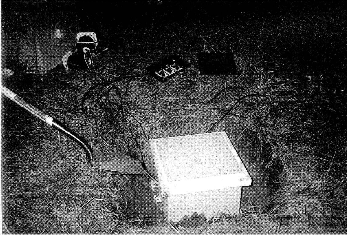
Figure 4-10 Placing Inner Sound Box
