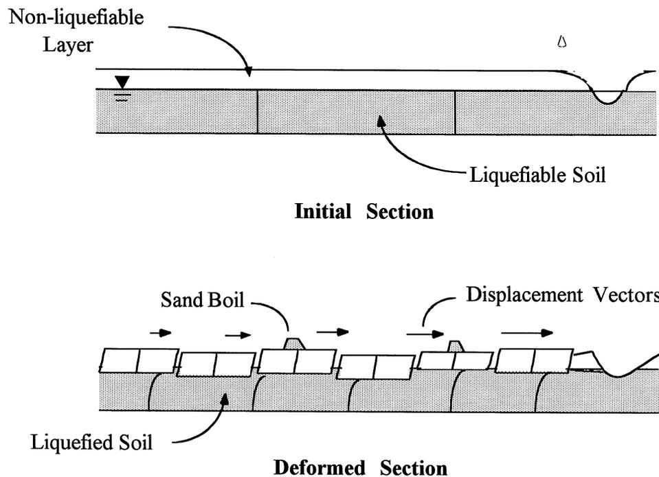
**FIGURE 2-1 Lateral Spreading Mechanism (after Youd, 1984)**
