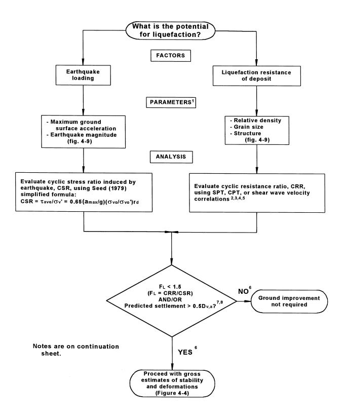
FIGURE 4-3 Assessment of Liquefaction Potential
