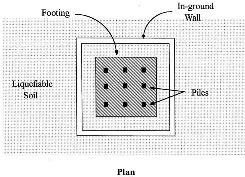
**FIGURE 5-9 Mixed-in-Place Wall Around Pile-Supported Pier (after Kawakami, 1996)**
