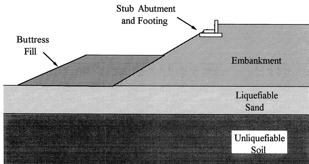
**FIGURE 5 -7 Section Showing Buttress Fill at Toe of Approach Embankment**
