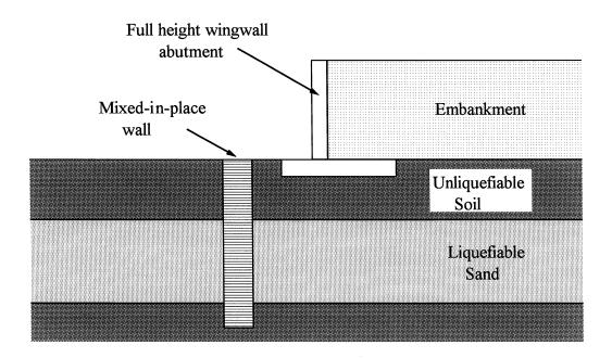
FIGURE 5-8 Section Showing Mixed-in-Place Wall in Front of Full-Height Wingwall Abutment
