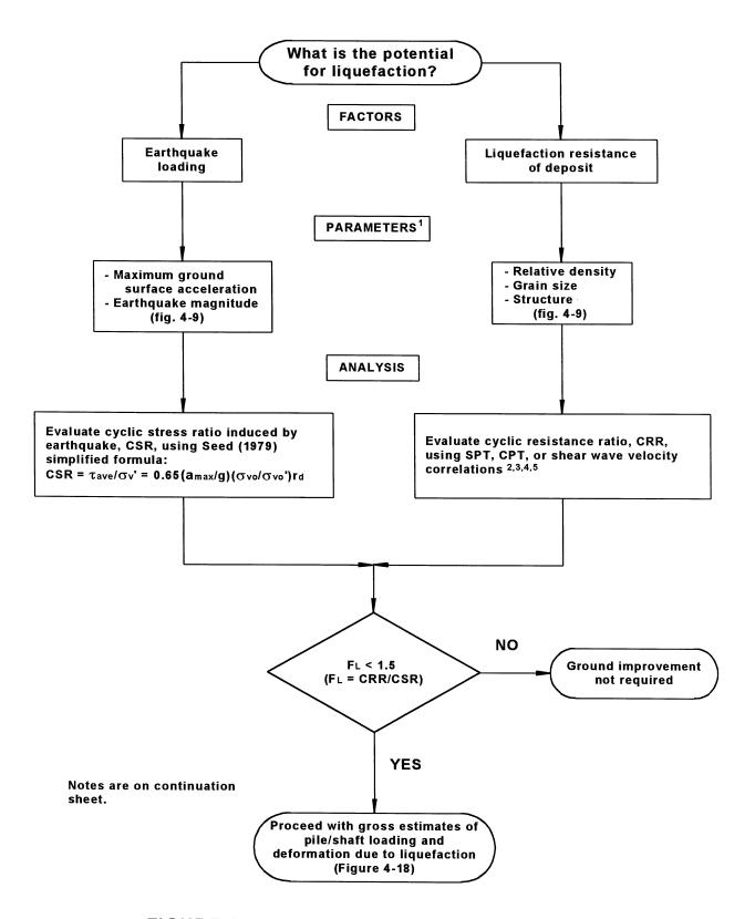
FIGURE 4-17 Assessment of Liquefaction Potential for Piles/Shafts
