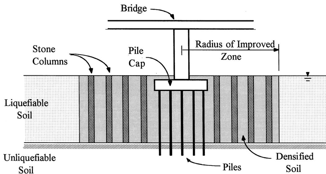
**FIGURE 5-5 Vibro System (Stone Column) Treatment Around a Pile-Supported Bridge Pier (after Jackura and Abghari, 1994)**
