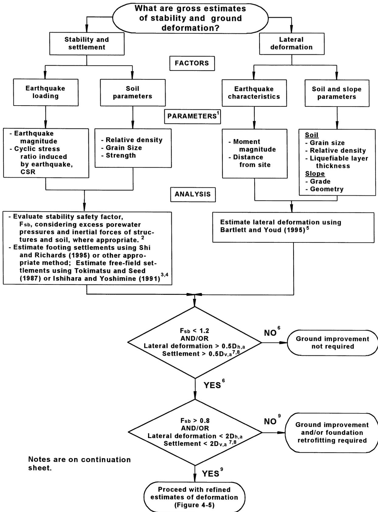
**FIGURE 4-4 Gross Stability and Deformation Estimates**
