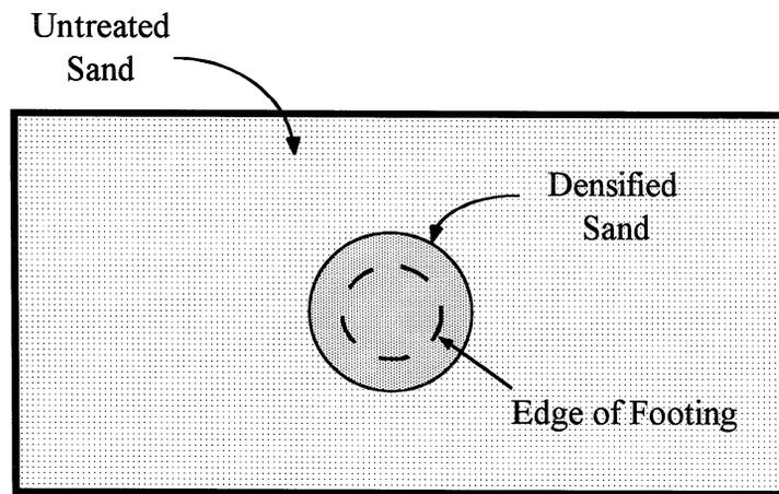
**FIGURE 5-21 Centrifuge Model of Footing on Densified Zone Tested by Liu and Dobry (after Liu and Dobry, 1997; dimensions in prototype scale)**
