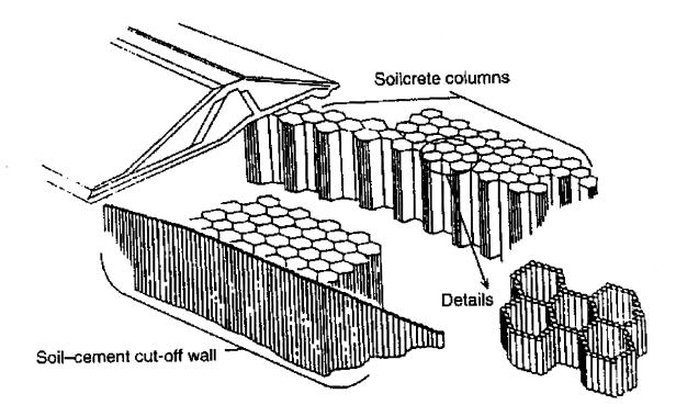
FIGURE A-4 Example Detail of Mixed-in-Place Columns Used to Form Containment Cells at Jackson Lake Dam Modification Project (Taki and Yang, (1991), "Soil-Cement Mixed Wall Technique," Proc., Geotechnical Engineering Congress 1991, Geotechnical Special Publication No. 27, ASCE. Reprinted by permission of ASCE.)
