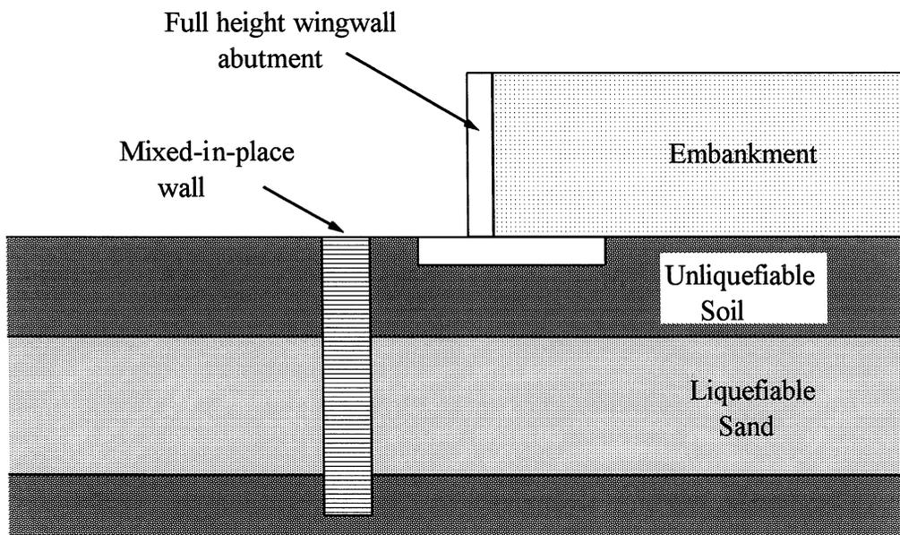
**FIGURE 5-8 Section Showing Mixed-in-Place Wall in Front of Full-Height Wingwall Abutment**
