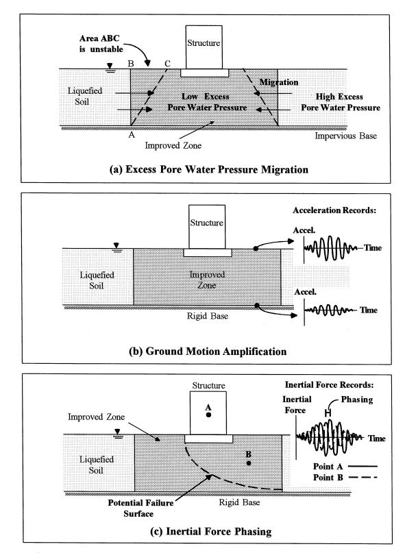
FIGURE 6-1 Factors Affecting Improved Ground Performance (after Mitchell et al. (1998), "Design Considerations in Ground Improvement for Seismic Risk Mitigation," Geotechnical Earthquake Engineering and Soil Dynamics III, Geotechnical Special Publication No. 30. Reprinted by Permission of ASCE.)
