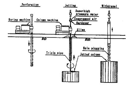
FIGURE A-2 Jet Grouting Process (from Ichibashi et al., (1992), "Jet Grouting in Airport Construction," Proc., Grouting, Soil Improvement and Geosynthetics, Geotechnical Special Publication No. 30, ASCE. Reprinted by permission of ASCE)
