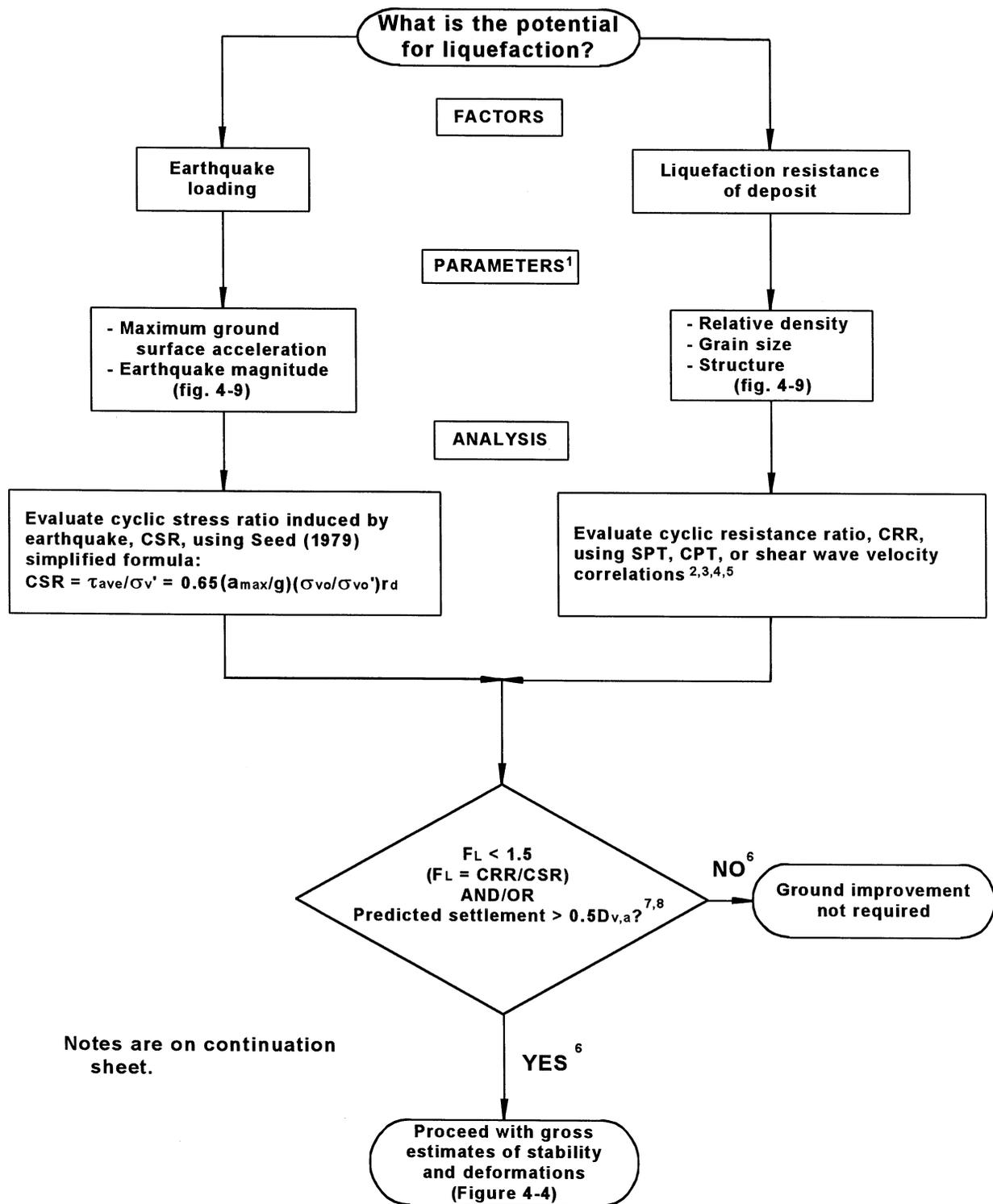
**FIGURE 4-3 Assessment of Liquefaction Potential**
