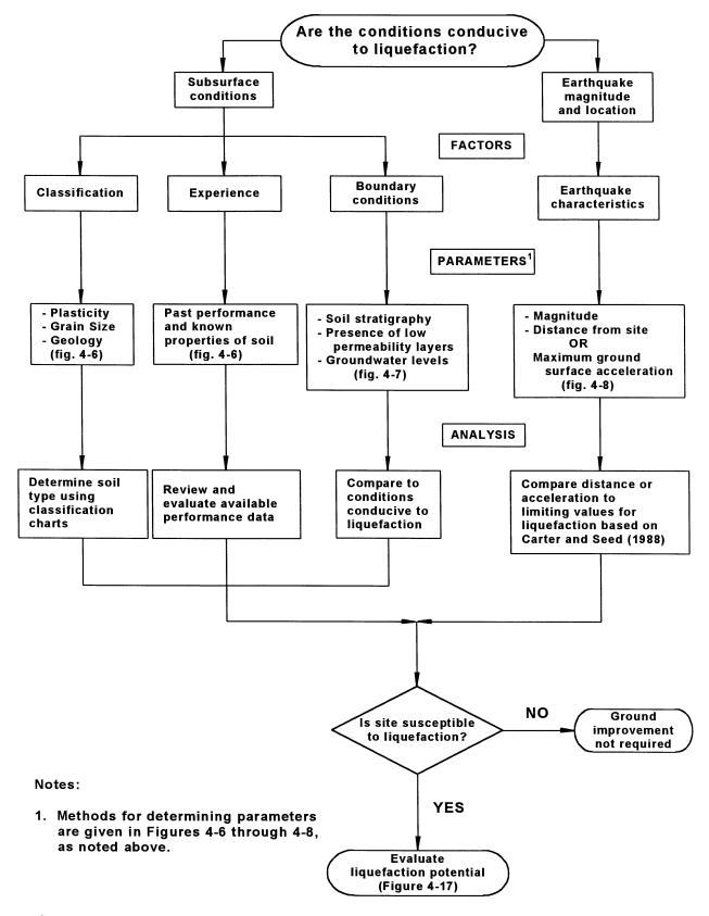
FIGURE 4-16 Preliminary Evaluation of Site and Earthquake Conditions for Piles/Shafts
