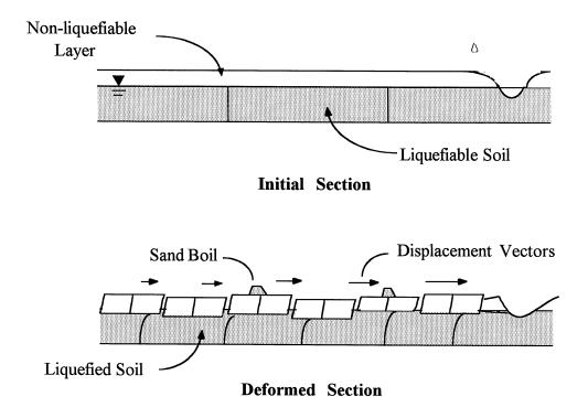
FIGURE 2-1 Lateral Spreading Mechanism (after Youd, 1984)
