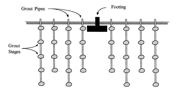
FIGURE 5-3 Section Showing Compaction Grouting Around Footing (after Graf, 1992)
