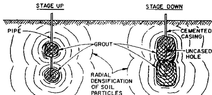
**FIGURE A-1 Compaction Grouting Densification Mechanism (from Graf (1992), "Compaction Grout, 1992," Proc., Grouting, Soil Improvement and Geosynthetics, Vol. II, Geotechnical Special Publication No. 30, ASCE. Reprinted by permission of ASCE)**
