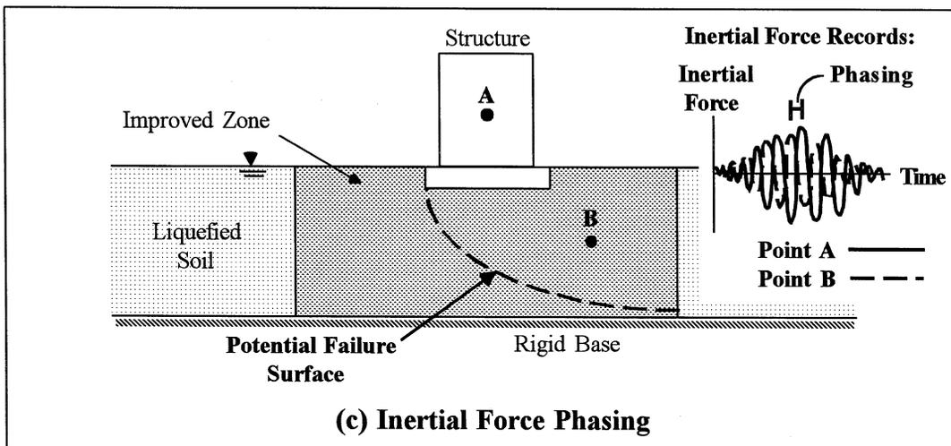
**FIGURE 6-1 Factors Affecting Improved Ground Performance (after Mitchell et al. (1998), "Design Considerations in Ground Improvement for Seismic Risk Mitigation," Geotechnical Earthquake Engineering and Soil Dynamics III, Geotechnical Special Publication No. 30. Reprinted by Permission of ASCE.)**
