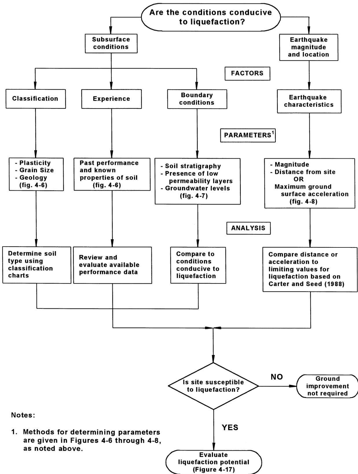
**FIGURE 4-16 Preliminary Evaluation of Site and Earthquake Conditions for Piles/Shafts**
