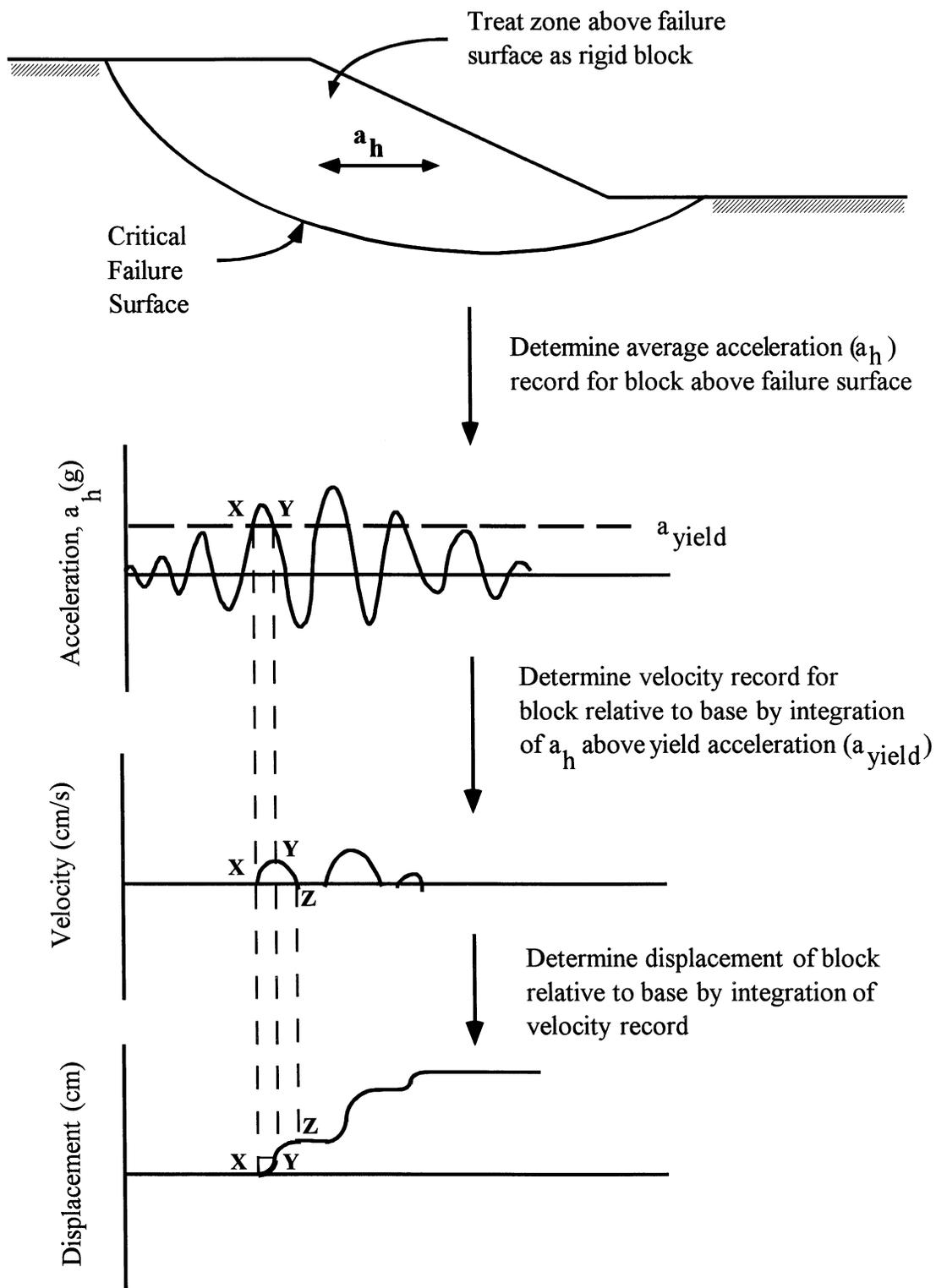
**FIGURE 3-2 Estimation of Displacements by Newmark (1965) Sliding Block Method (after Jibson, 1993)**
