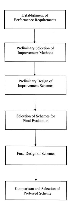
Figure 6-2 Remedial Measure Design Procedure
