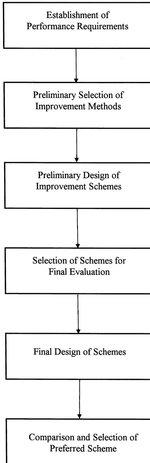
**Figure 6-2 Remedial Measure Design Procedure**
