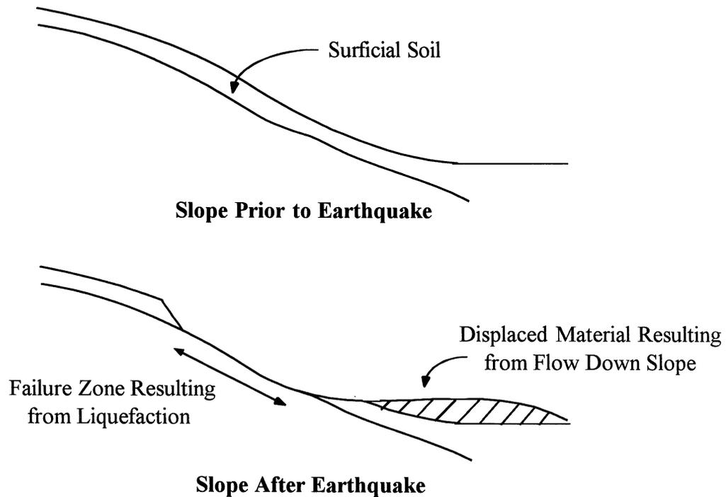
**FIGURE 2-4 Flow Failure (after Youd, 1984)**
