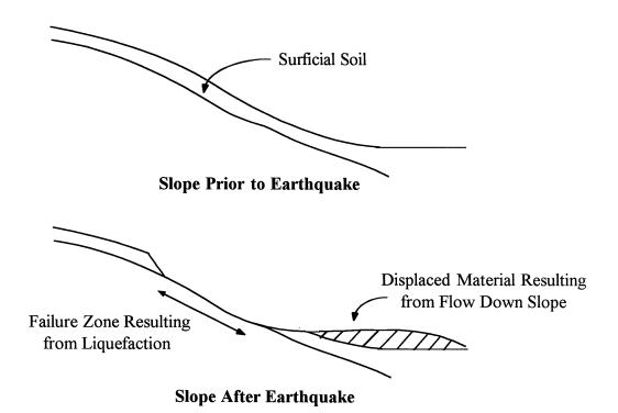
FIGURE 2-4 Flow Failure (after Youd, 1984)
