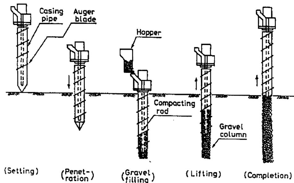
**Figure A-5 Gravel Drain Installation (from Ono et al. (1991), "Efficient Installation of Gravel Drains," Proc., 2nd International Conference on Recent Advances in Geotechnical Earthquake Engineering and Soil Dynamics, Vol. 1, University of Missouri, Rolla.)**
