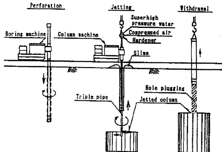
**FIGURE A-2 Jet Grouting Process (from Ichibashi et al., (1992), “Jet Grouting in Airport Construction,” Proc., Grouting, Soil Improvement and Geosynthetics, Geotechnical Special Publication No. 30, ASCE. Reprinted by permission of ASCE)**
