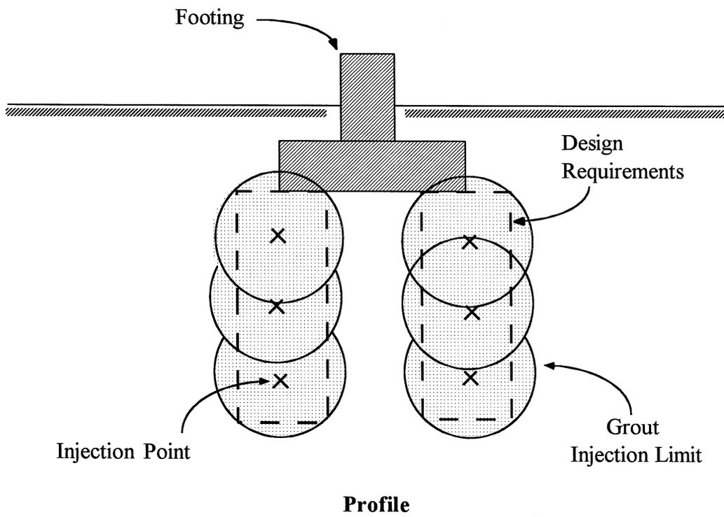
**FIGURE 5-4 Permeation Grouted Zone Beneath a Footing (after Andrus and Chung, 1995)**
