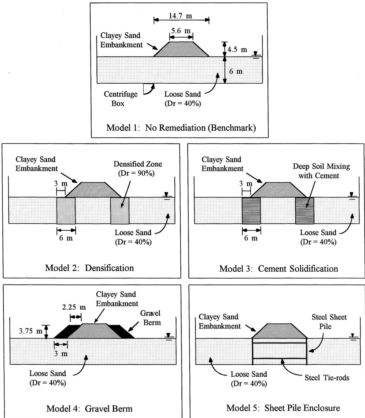
**FIGURE 5-14 Improvement Schemes for Embankment Modeled in Centrifuge Tests by Adalier (after Adalier et al., 1998; dimensions in prototype scale)**
