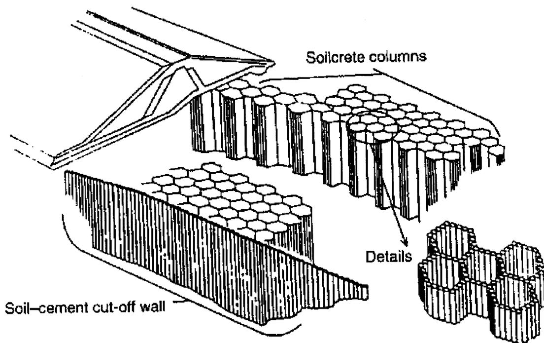
**FIGURE A-4 Example Detail of Mixed-in-Place Columns Used to Form Containment Cells at Jackson Lake Dam Modification Project (Taki and Yang, (1991), "Soil-Cement Mixed Wall Technique," Proc., Geotechnical Engineering Congress 1991, Geotechnical Special Publication No. 27, ASCE. Reprinted by permission of ASCE.)**
