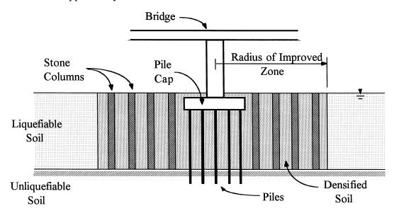
FIGURE 5-5 Vibro System (Stone Column) Treatment Around a Pile-Supported Bridge Pier (after Jackura and Abghari, 1994)
