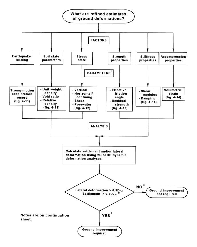
**FIGURE 4-5** Refined Deformation Estimates
