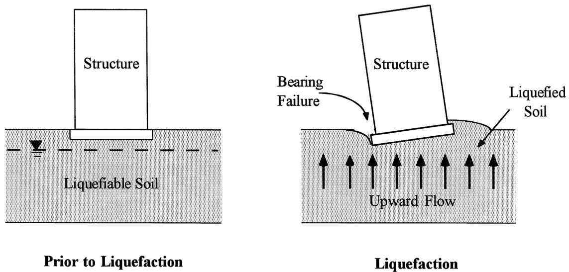
**FIGURE 2-2 Bearing Capacity Failure (after Youd, 1984)**
