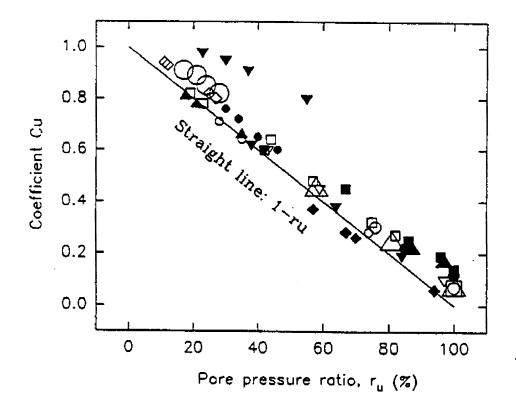
FIGURE 3-7 p-y Curve Degradation Parameter for Pile in Sand having Excess Pore Water Pressures (from Liu and Dobry, 1994)
