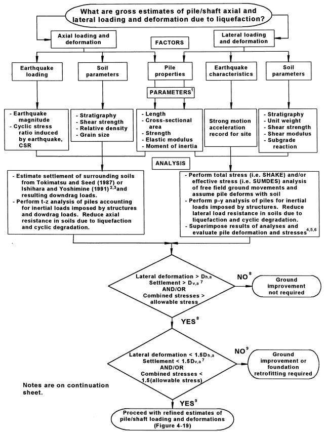
FIGURE 4-18 Gross Pile/Shaft Loading and Deformation Estimates
