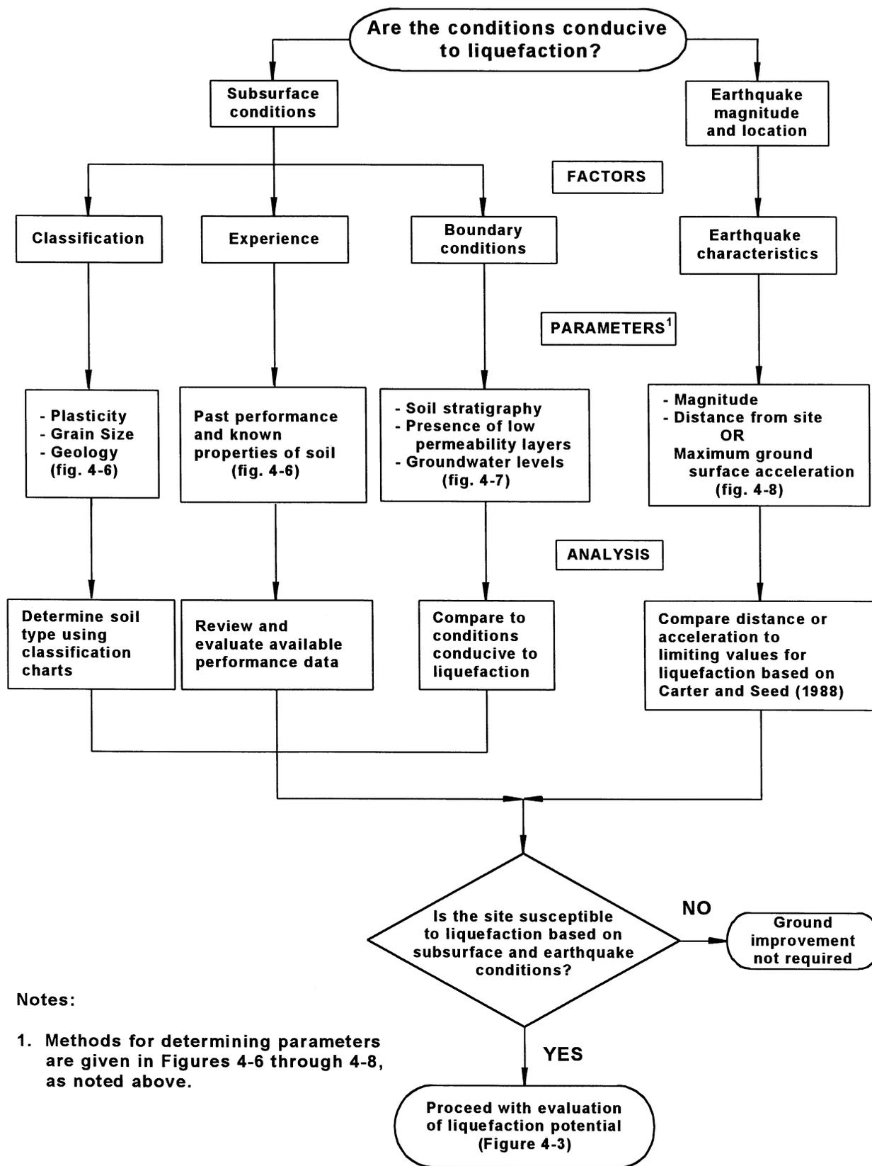
**FIGURE 4-2 Preliminary Evaluation of Site and Earthquake Conditions**
