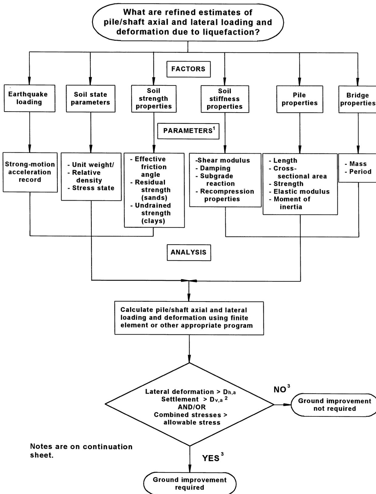
**FIGURE 4-19 Refined Pile/Shaft Loading and Deformation Estimates**
