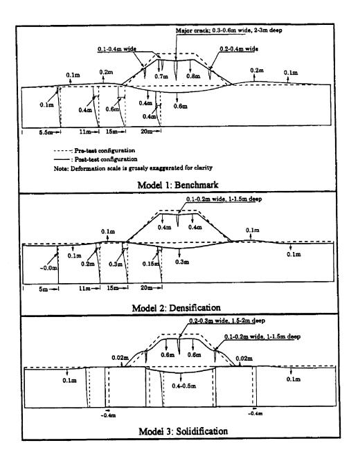
FIGURE 5-15 Ground Deformations (in Prototype Scale) Observed in Centrifuge Tests By Adalier (from Adalier et al., (1998). "Foundation Liquefaction Countermeasures for Earth Embankments," Journal of Geotechnical and Geoenvironmental Engineering, ASCE, Vol. 124, No. 6. Reprinted by permission of ASCE)
