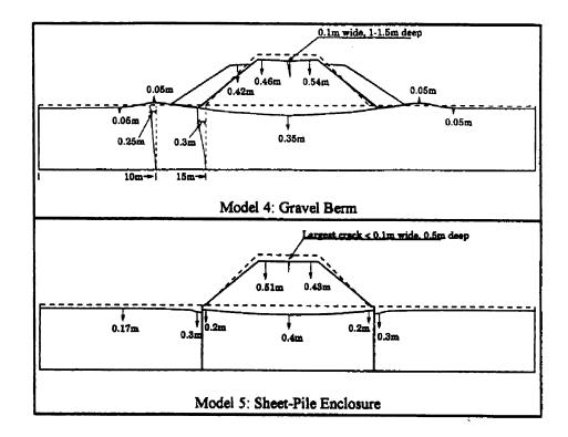
FIGURE 5-15 (cont.) Ground Deformations (in Prototype Scale) Observed In Centrifuge Tests by Adalier (from Adalier et al., (1998). "Foundation Liquefaction Countermeasures for Earth Embankments," Journal of Geotechnical and Geoenvironmental Engineering, ASCE, Vol. 124, No. 6. Reprinted by permission of ASCE)
