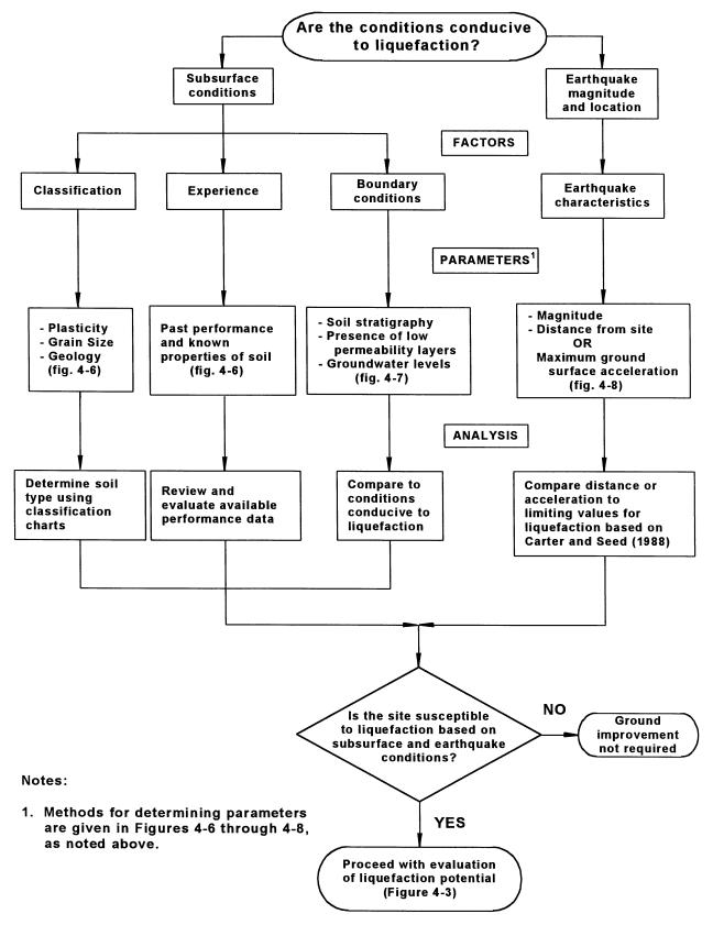
FIGURE 4-2 Preliminary Evaluation of Site and Earthquake Conditions
