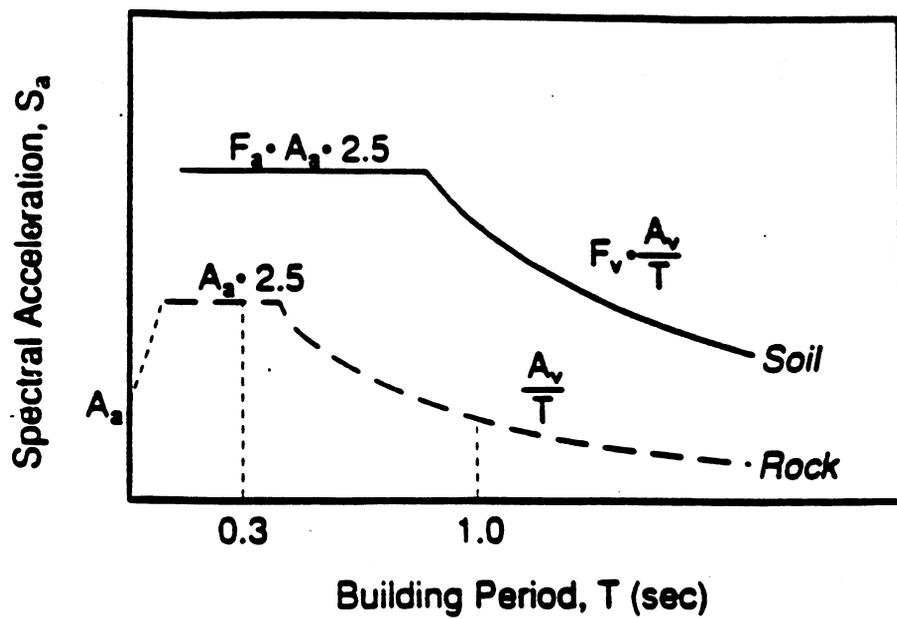
Figure 4-3 Two-factor approach to local site response incorporated into 1994 NEHRP and 1997 UBC (NEHRP, 1994)
