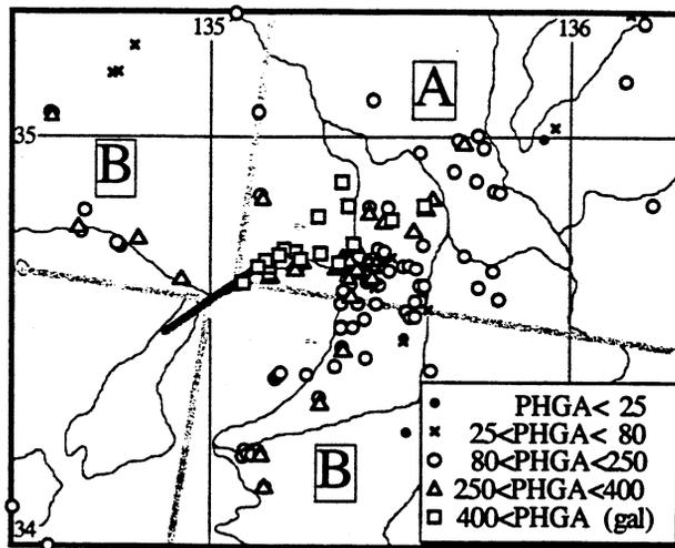
Figure 6-13 Distribution of peak ground horizontal accelerations with respect to the fault rupture in 1995 Kobe earthquake (Ejiri et al., 1996)
