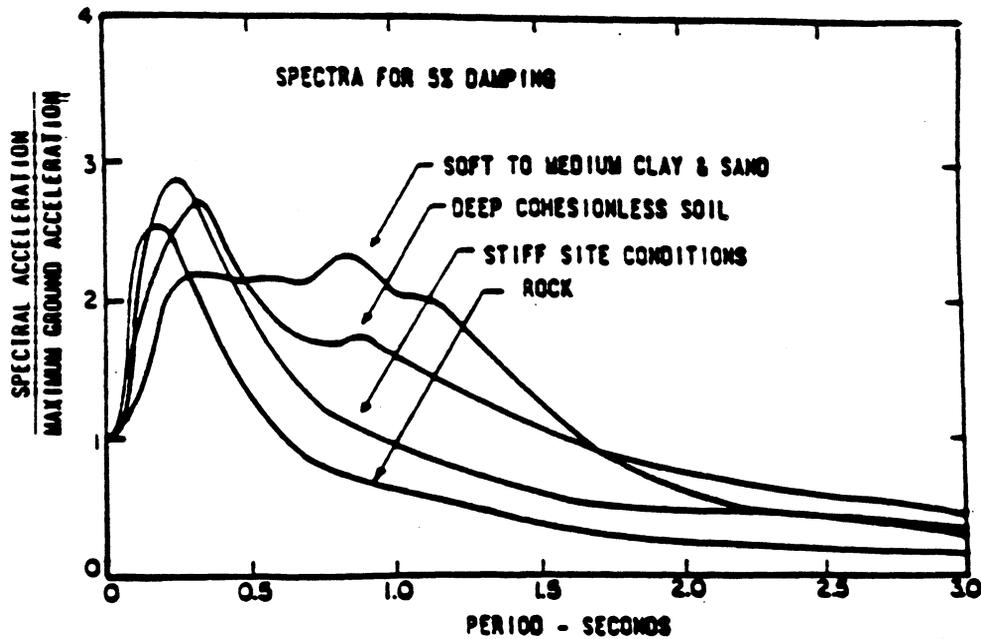
Figure 3-2 Average acceleration spectra for different site conditions (Seed et al., 1976a and 1976b)
