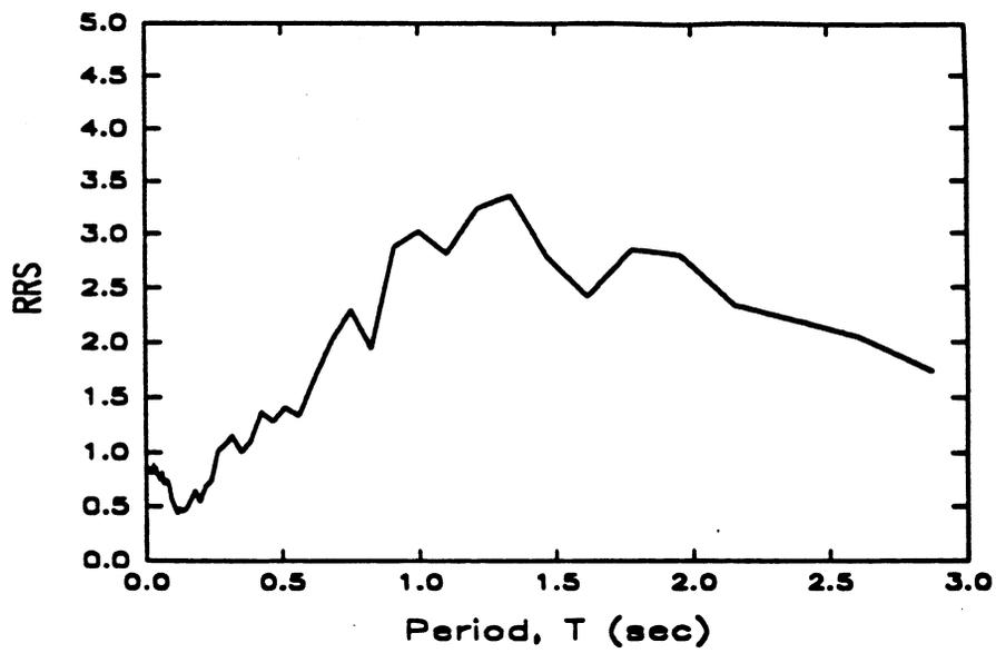
Figure 2-3 Determination of Ratio of Response Spectra (RRS) between soil and rock
