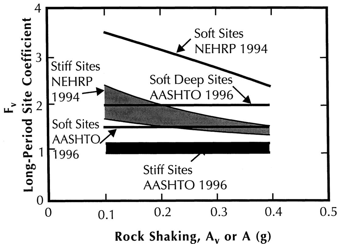
Figure 4-4 Influence of level of rock shaking on short and long period site coefficients at soft (E) and stiff (C and D) sites in new building codes (values from Table 3)
