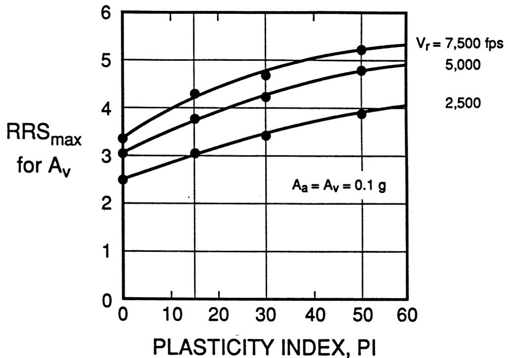
Figure 4-2 Variation of  $RRS_{max}$  of uniform layer of soft clay on rock from analyses (Dobry et al., 1994; NEHRP, 1994)
