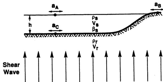
Figure 2-5 Uniform soil layer on elastic rock subjected to vertical shear waves
