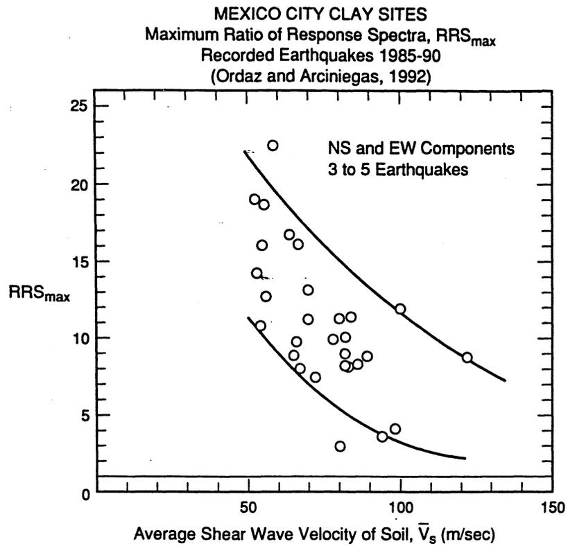
Figure 2-4 Maximum Ratio of Response Spectra,  $(RRS)_{max}$ , versus  $\bar{V}_s$ , recorded on Mexico City clay sites during five earthquakes between 1985 and 1990 (Ordaz and Arciniegas, 1992)
