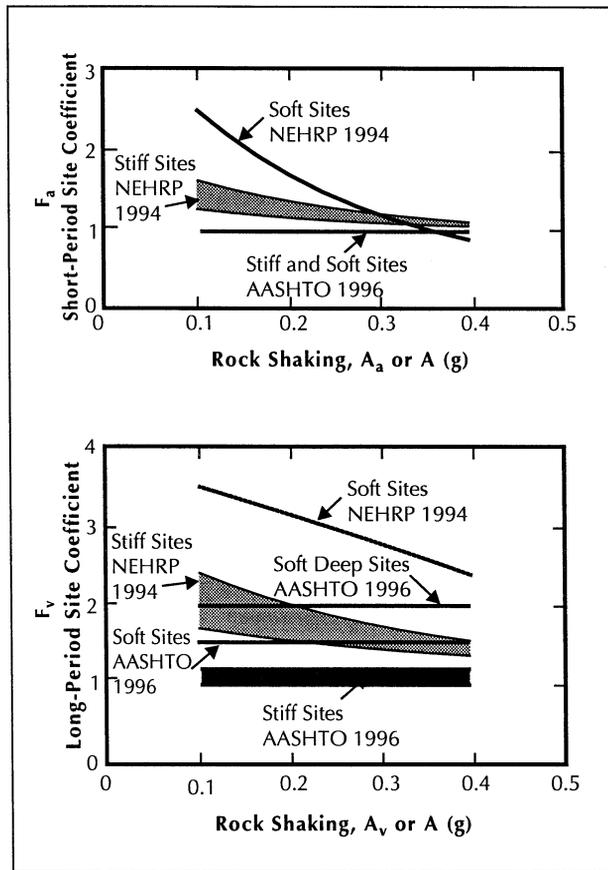
Figure 5-1 Comparison of Site Coefficients Contained in New Building Codes (NEHRP 1994 and UBC 1997) and in Specifications for Highway Bridges (AASHTO 1996)
