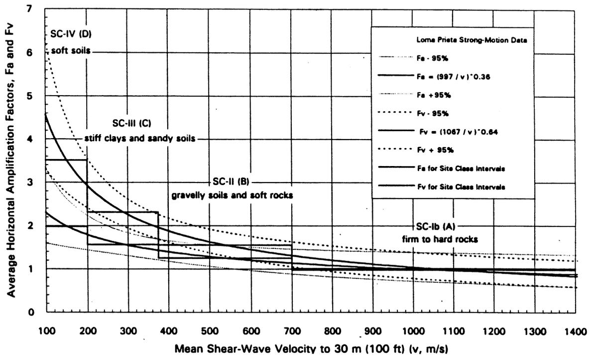
Figure 2-9 Short-period  $F_a$  and mid-period  $F_v$  amplification factors with respect to “firm to hard” rock plotted as a continuous function of mean shear wave velocity using the regression equations derived from the strong-motion recordings of the Loma Prieta earthquake. The 95 percent confidence intervals for the ordinate to the true population regressions line and the amplification factors for the simplified site classes also are shown (Borcherdt, 1994)
