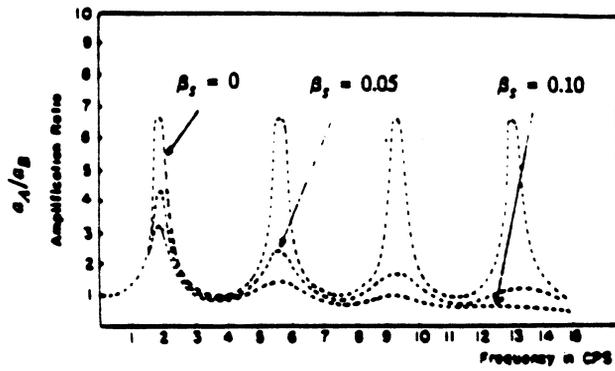
Figure 2-6 Amplification ratio soil/rock for  $h = 100$  ft (30.5m),  $V_s = 1.88$  cps, and  $IR = 6.7$  (Roesset, 1977).
