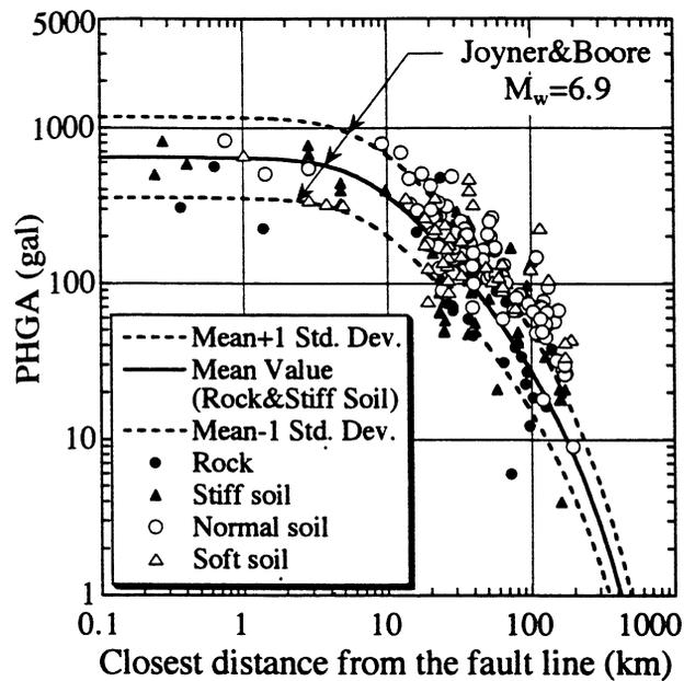
Figure 6-14 Attenuation of peak ground acceleration with distance for different site conditions in 1995 Kobe earthquake (Ejiri et al., 1996)
