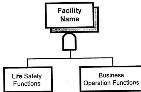
Figure 3-1: Facility Top Logic Model
