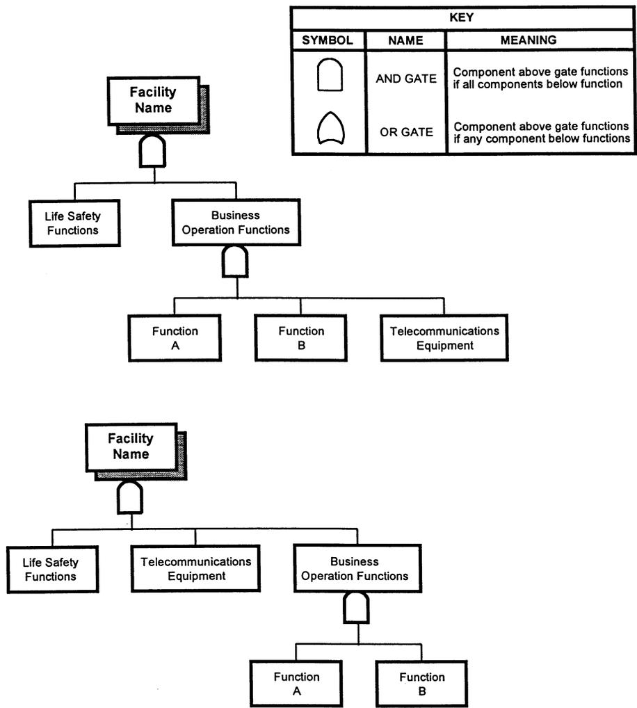
**Figure 2-2: Equivalent Logic Model Configurations**
