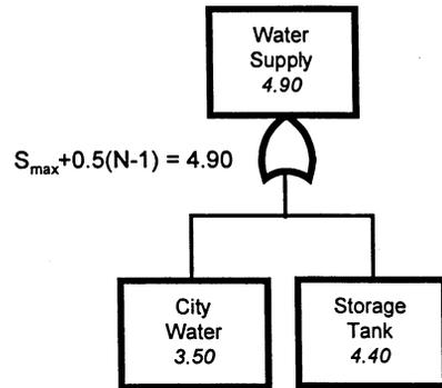
The water supply can be provided by either an on-site storage tank or a connection to the municipal water supply. The score for this redundant subsystem is dependent on the number of redundant components ( $N = 2$ ) and the highest component score ( $S_{\max} = 4.40$ ). The formula to calculate the water supply score is shown above.
