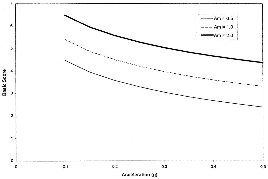
Figure 4-5: Scores based on annual probability of failure (Beta = 0.4)
