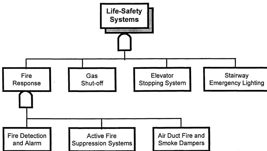
Figure 3-3: Life-Safety Systems/Fire Response Level Logic
