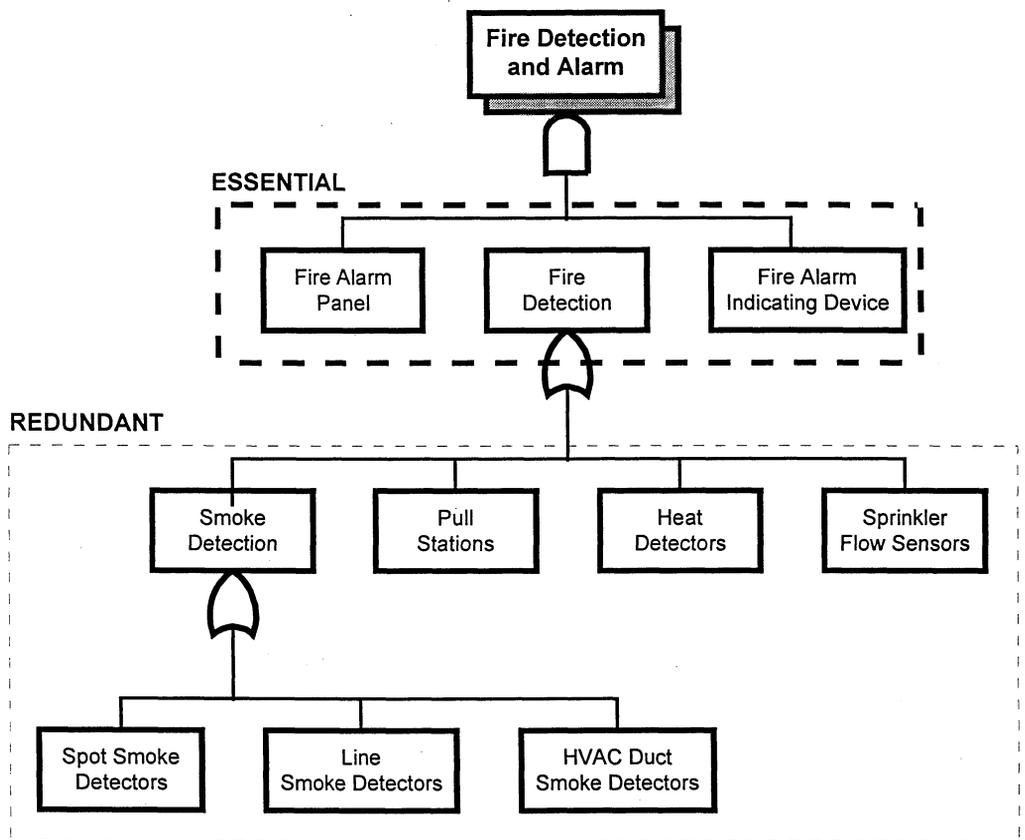
Figure 3-4: Fire Detection and Alarm Logic Example
