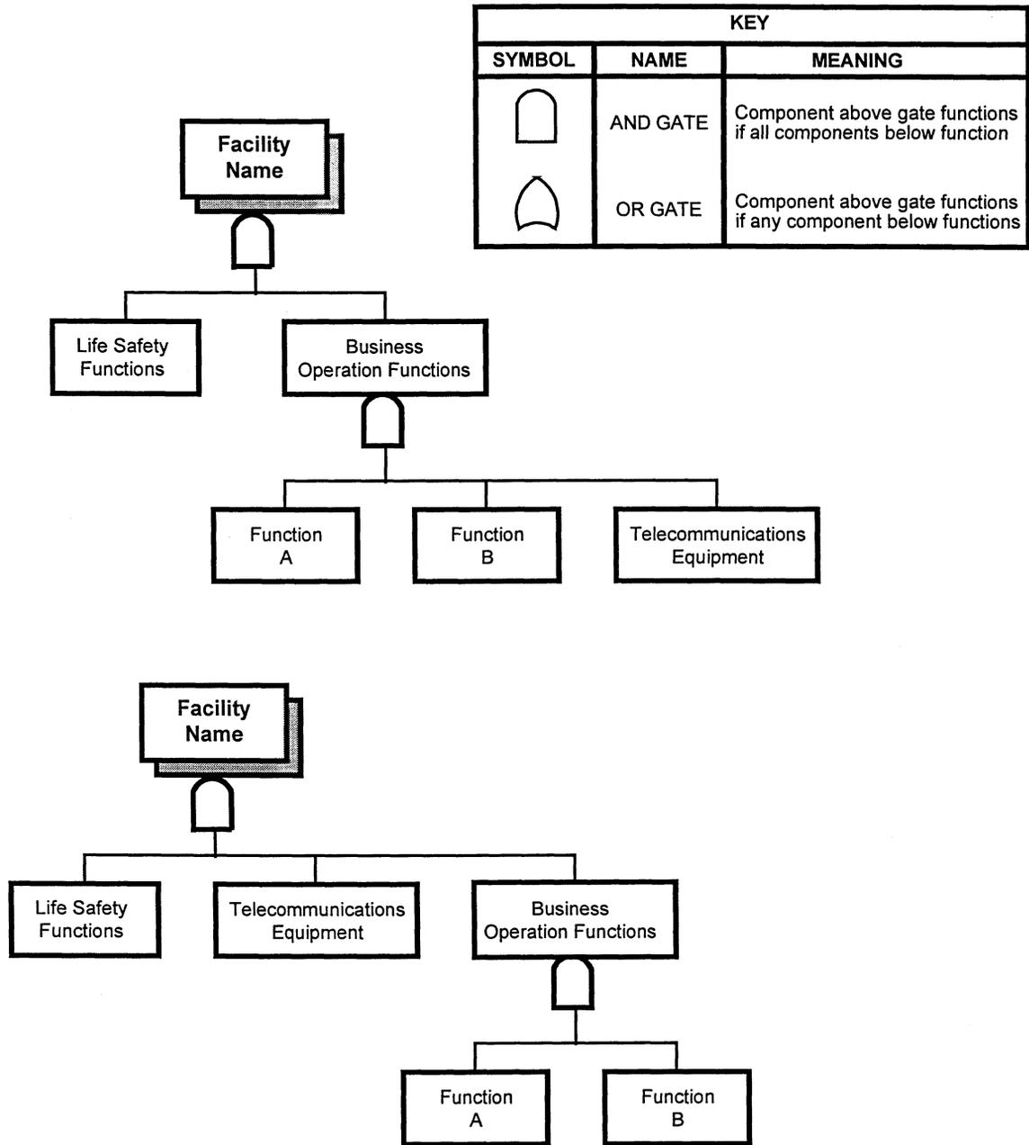
Figure 3-2: Equivalent Logic Model Configurations
