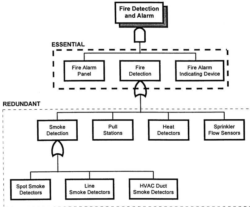
**Figure 2-4: Fire Detection and Alarm Logic Example**
