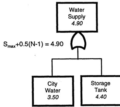
The water supply can be provided by either an on-site storage tank or a connection to the municipal water supply. The score for this redundant subsystem is dependent on the number of redundant components ( $N = 2$ ) and the highest component score ( $S_{\max} = 4.40$ ). The formula to calculate the water supply score is shown above.
