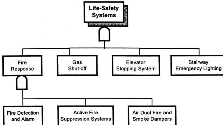
**Figure 2-3: Life-Safety Systems/Fire Response Level Logic**
