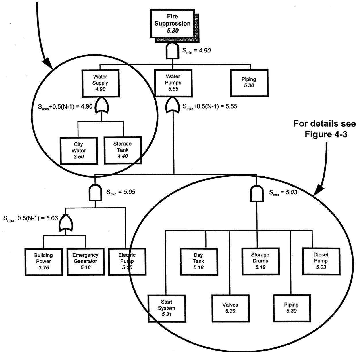
**Figure 4-1: Illustration of system scoring**
