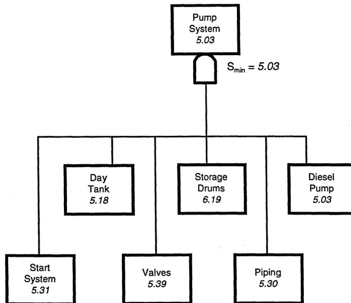
The pump system will not function unless all its components function. The score for this dependant system is controlled by the lowest component score. In this case the diesel pump ( $S = 5.03$ ) is the controlling component.
