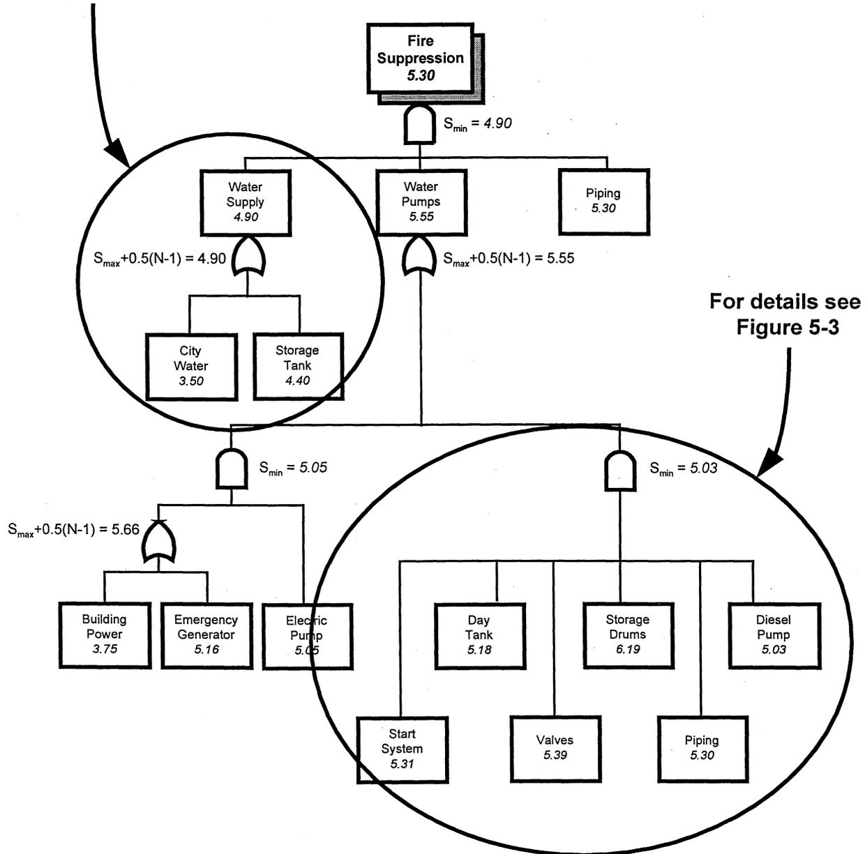
Figure 5-1: Illustration of system scoring
