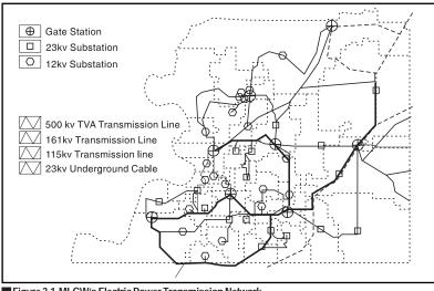
the network consisting of 500 kv, 16l kv, 115 kv and 23 kv transmission lines and gate, 23 kv and 12 kv substations. The 500 kv line and gate stations are operated by TVA, and other transmission lines and substations by MLGW. Each substation is associated with a service area, and usually one service area is served by only one substation with two exceptions.
