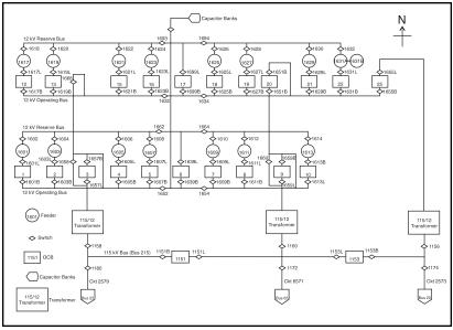
Figure 3.2 Schematic Diagram of MLGW Substation 21
