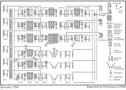
■ Figure 3.3 Damaged Equipment of Moss Landing 500kv Switchyard at the 1989 Loma Prieta Earthquake
