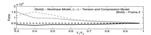
Figure 8.6: Frame Forces from Bounding Models for Frames Subjected to 1940 El Centro Earthquake (S00E Component),  $T_2/T_g = 1.0$ .
