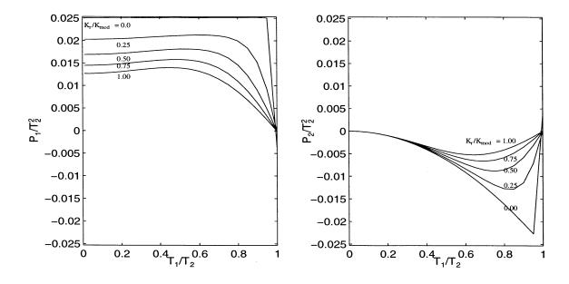
Figure 5.4: Normalized Modal Participation Factors as a Function of Frame Period Ratio and Restrainer Stiffness Ratio.
