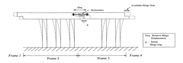
Figure 1.2: Interaction of Frames Subjected to Earthquake Loads.
