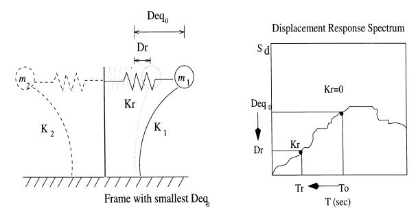
Figure 2.9: Interpretation of Caltrans Equivalent Static Procedure for Hinge Restrainers (Caltrans, 1990).
