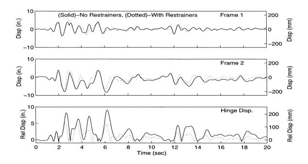
Figure 5.11: Response History for Two Frames Subjected to 1940 El Centro Earthquake (S00E Component) Using Restrainers Determined in Example 5.1.
