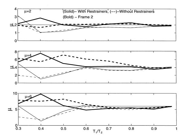
Figure 8.7: Frame Ductility Demands Using Tension and Compression Bounding Models for Frames Subjected to 1940 El Centro Earthquake (S00E Component),  $T_2/T_g=1.0$ .
