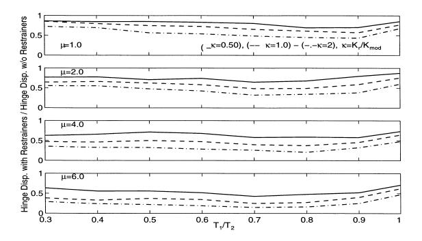
Figure 4.6: Effect of Restrainer Stiffness Ratio on Hinge Displacement Ratio for  $T_2/T_g=0.5$ : Mean for 26 Earthquake Records.
