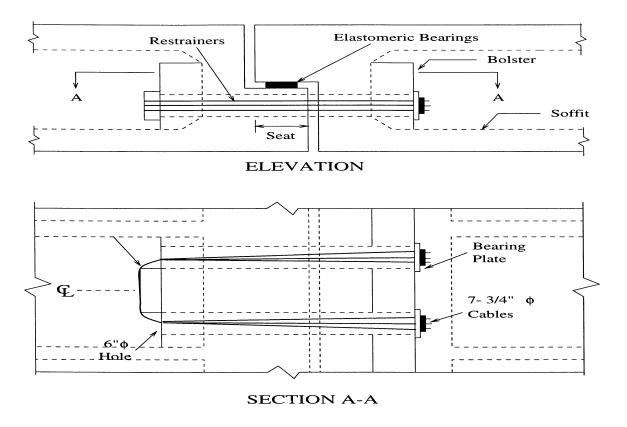
Figure 2.3: Older Hinge Restrainer Retrofit Scheme: Type C1 Restrainer Unit.
