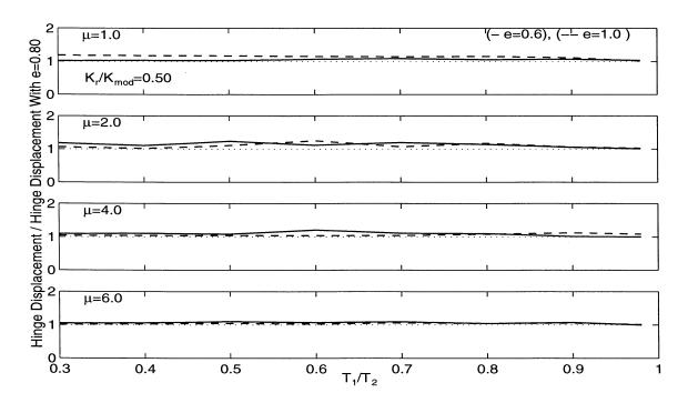
Figure 4.17: Effect of Coefficient of Restitution on Hinge Displacement,  $T_2/T_g=1.0$ , Mean Plus One Standard Deviation for 26 Earthquakes.
