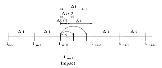
Figure 3.4: Variable Time Stepping Strategy for Numerical Solution of Pounding of Frames.
