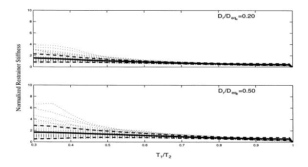
Figure 6.2: Mean  $\pm$  One Standard Deviation of the Normalized Restrainer Stiffness for  $\tilde{T}=0.50.$
