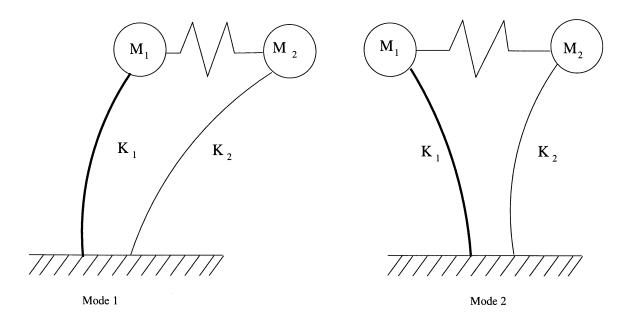
Figure 5.2: Mode Shape For 2-DOF System Representing Bridge Frames with Restrainers
