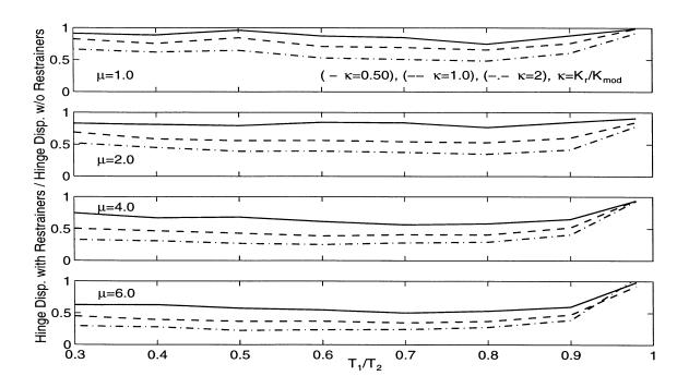
Figure 4.5: Effect of Restrainer Stiffness Ratio on Hinge Displacement Ratio for  $T_2/T_g=1.0$ : Mean Plus One Standard Deviation for 26 Earthquake Records.
