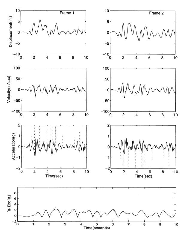
Figure 3.6: Comparison of Numerical Procedure with DRAIN3-DX for Inelastic Frame Response to 1940 El Centro Earthquake (S00E Component ), Scaled to 0.70g with  $\mu=4$  (..... DRAIN3-DX) (—— Numerical Procedure).
