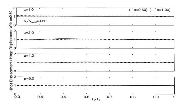
Figure 4.16: Effect of Coefficient of Restitution on Hinge Displacement,  $T_2/T_g=1.0$ , Mean for 26 Earthquakes.
