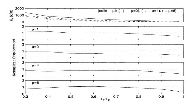
Figure 5.19: Evaluation of Restrainer Design Procedure: 1994 Northridge Earthquake (Sylmar Hospital Free-Field Record),  $D_r/D_{eq}$ =0.20,  $T_2/T_g$ =1.0.
