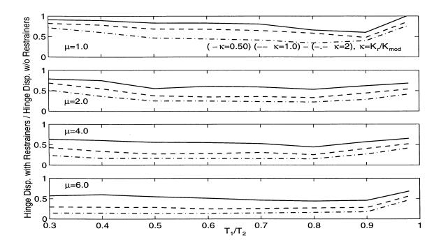
Figure 4.3: Effect of Restrainer Stiffness Ratio on Hinge Displacement Ratio for 1994 Northridge Earthquake (Sylmar Hospital Free-Field Record),  $T_2/T_g=1.0$ .
