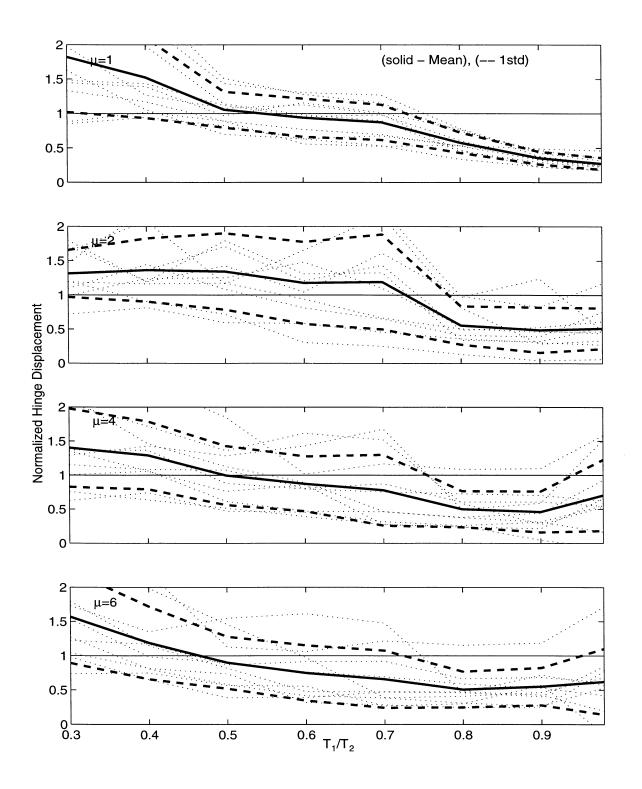
Figure 6.18: Mean  $\pm$  One Standard Deviation of the Normalized Hinge Displacement from Single-Step Design Procedure for  $D_r/D_{eq}$ =0.20,  $T_2/T_g$ =2.0.
