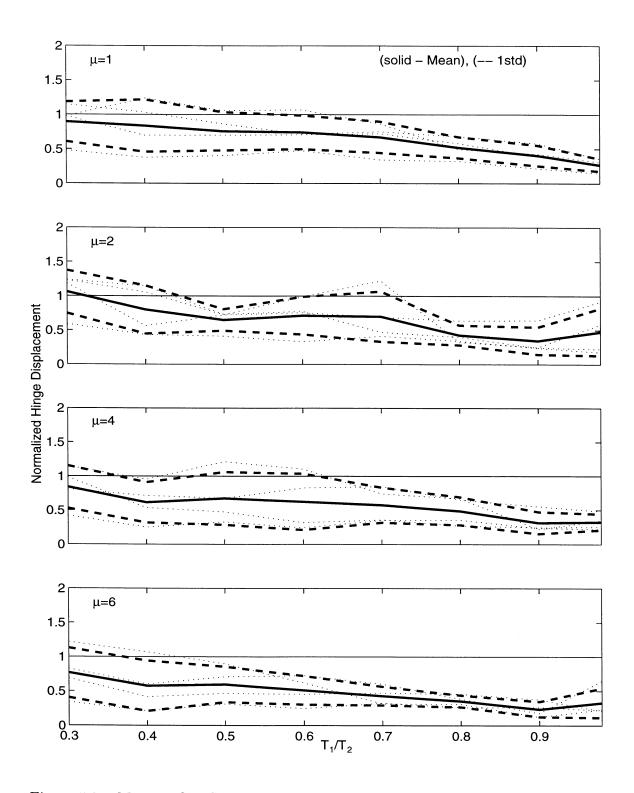
Figure 5.31: Mean  $\pm$  One Standard Deviation of Normalized Hinge Displacement for Restrainers from Design Procedure  $(D_r/D_{eq}=0.20,\,T_2/T_g=6.00)$ .
