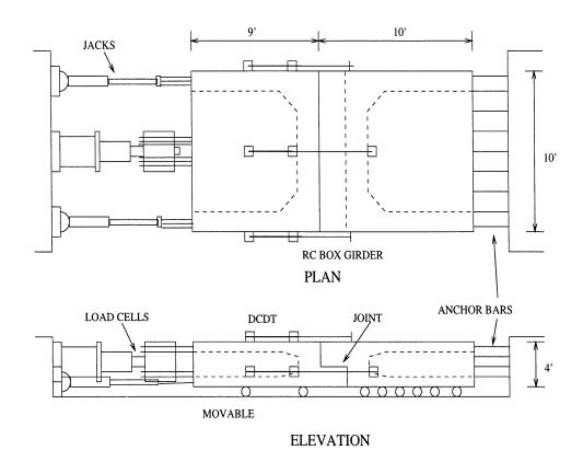
Figure 2.11: Test Specimen and Testing Arrangement for Experimental Studies on Hinge Restrainers (Selna, 1989).
