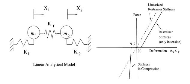
Figure 5.1: Simplified Linear Model for Longitudinal Earthquake Response of Two Adjacent Frames.
