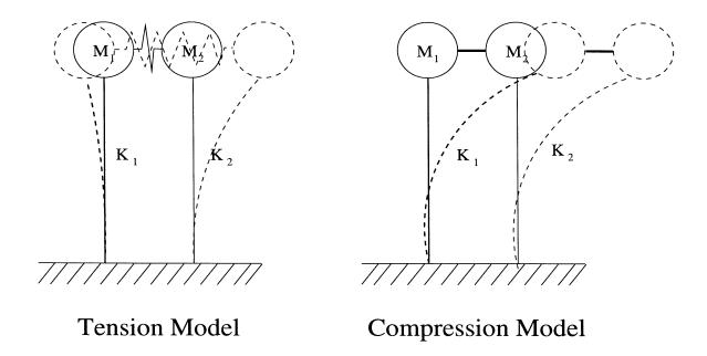
Figure 8.4: Schematic Representation of Tension and Compression Bounding Models
