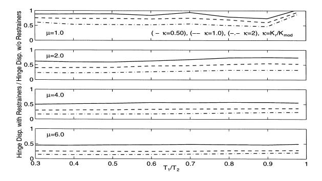
Figure 4.19: Effect of Restrainer Stiffness Ratio on Hinge Displacement for  $m_1/m_2 = 4.0$ , Mean for 26 Earthquake Records.
