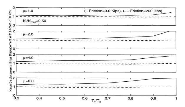
Figure 4.12: Effect of Friction on the Hinge Displacement,  $T_2/T_g=1.0$ , Mean for 26 Earthquakes.
