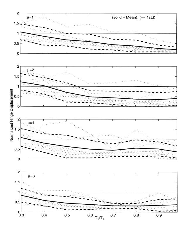
Figure 6.20: Mean  $\pm$  One Standard Deviation of the Normalized Hinge Displacement from Single-Step Design Procedure for  $D_r/D_{eq}$ =0.50,  $T_2/T_g$ =4.0.
