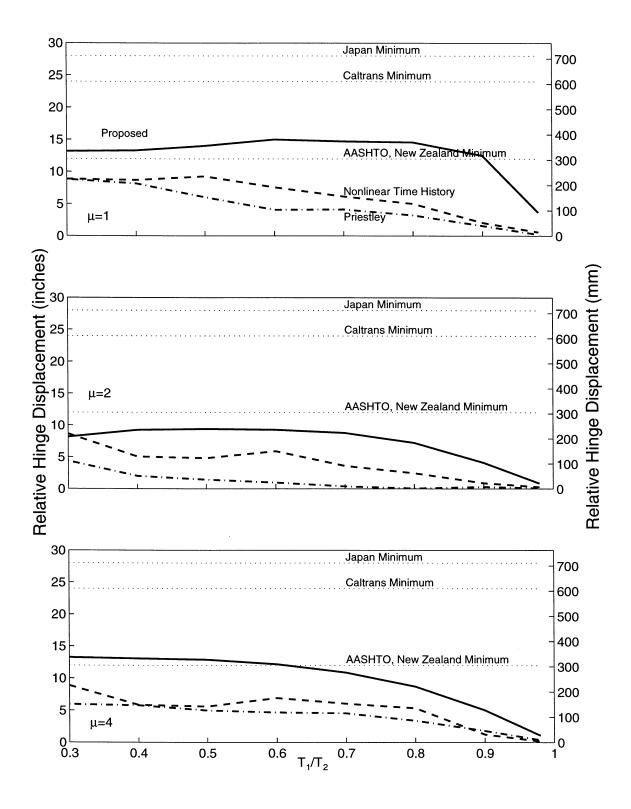
Figure 7.12: Comparison of Hinge Seat Widths with Nonlinear Time History Analysis for 1940 El Centro Earthquake (S00E Component),  $T_2/T_g=1.0$ .
