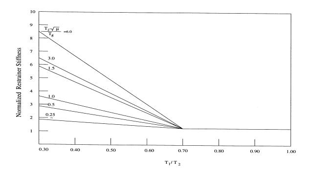
Figure 6.8: Bilinear Curve-Fit for Normalized Restrainer Stiffness for  $D_r/D_{eq_o}=0.50$ .
