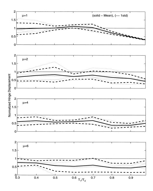
Figure 6.14: Mean  $\pm$  One Standard Deviation of the Normalized Hinge Displacement from Single-Step Design Procedure for  $D_r/D_{eq}$ =0.20,  $T_2/T_g$ =0.5.
