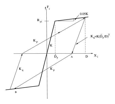
Figure 3.2: Q-Hyst Model Force-Deformation Relationship for Frame.
