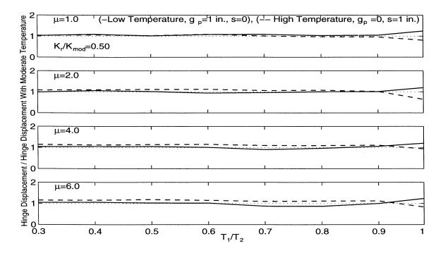
Figure 4.10: Effect of Hinge Gap and Restrainer Slack on Hinge Displacement Ratio for  $T_2/T_g=1.0$ : Mean for 26 Earthquake Records.
