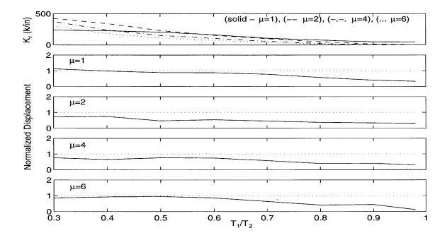
Figure 5.20: Evaluation of Restrainer Design Procedure: 1994 Northridge Earthquake (Sylmar Hospital Free-Field Record),  $D_r/D_{eq}$ =0.50,  $T_2/T_g$ =1.0.
