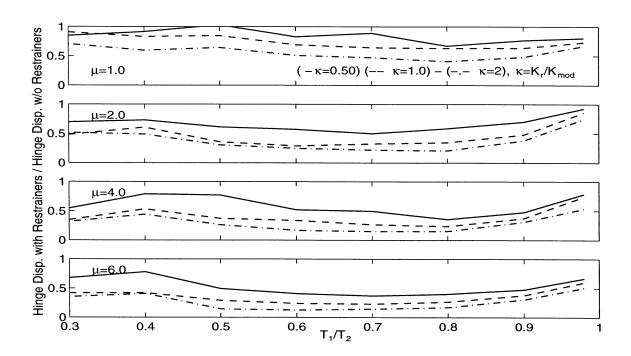
Figure 4.2: Effect of Restrainer Stiffness Ratio on Hinge Displacement Ratio for 1940 El Centro Earthquake (S00E Component),  $T_2/T_g = 1.0$ .
