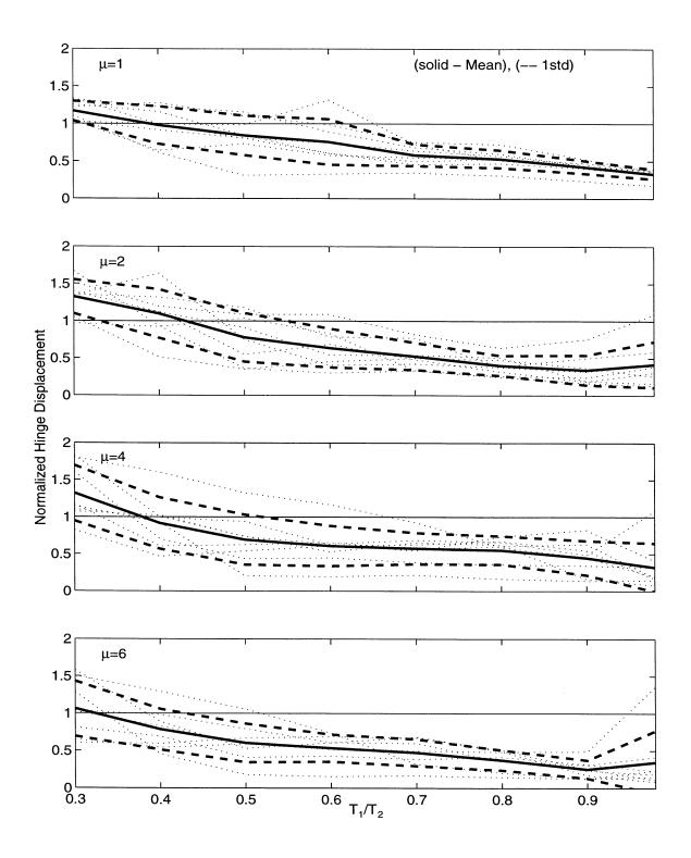
Figure 5.29: Mean  $\pm$  One Standard Deviation of Normalized Hinge Displacement for Restrainers from Design Procedure  $(D_r/D_{eq}=0.20,\,T_2/T_g=4.00)$ .
