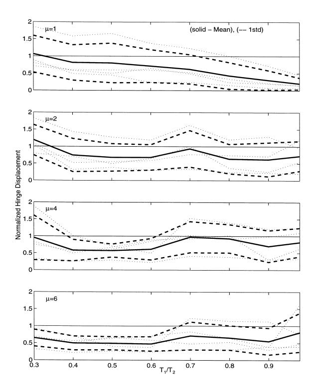
Figure 6.21: Mean  $\pm$  One Standard Deviation of the Normalized Hinge Displacement from Single-Step Design Procedure for  $D_r/D_{eq}$ =0.50,  $T_2/T_g$ =6.0.
