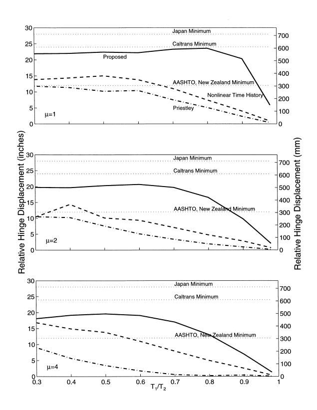
Figure 7.13: Comparison of Proposed Hinge Seat Widths with Nonlinear Time History Analysis for 1994 Northridge Earthquake (Sylmar Hospital Free-Field Record),  $T_2/T_g=1.0$ .
