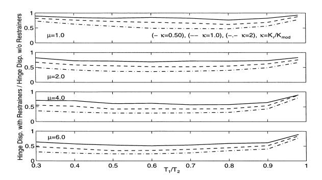
Figure 4.7: Effect of Restrainer Stiffness Ratio on Hinge Displacement Ratio for  $T_2/T_g=2.0$ : Mean for 26 Earthquake Records.
