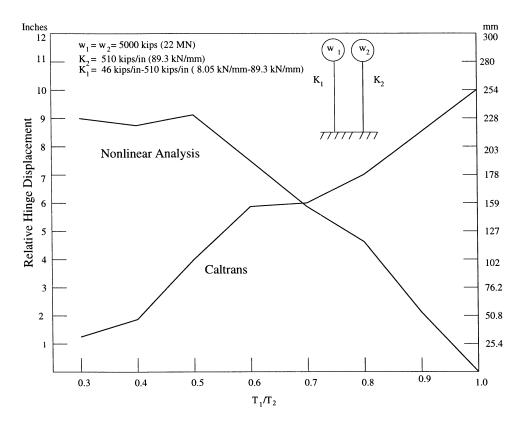
Figure 2.10: Relative Hinge Displacement Based on Nonlinear Analysis and the Caltrans Procedure.
