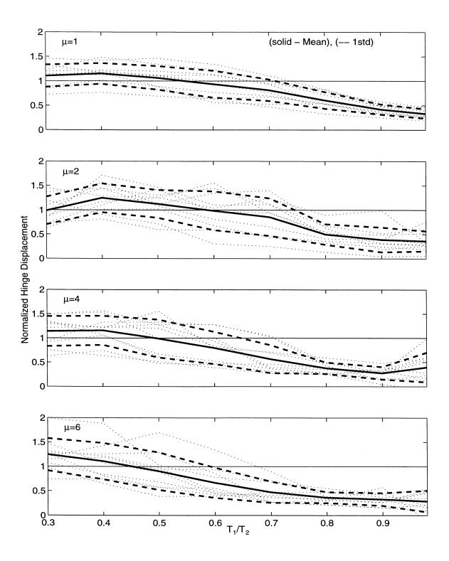
Figure 5.27: Mean  $\pm$  One Standard Deviation of Normalized Hinge Displacement for Restrainers from Design Procedure  $(D_r/D_{eq}=0.20,\,T_2/T_g=2.00)$ .
