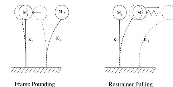
Figure 8.1: Schematic Representation of Frame Pounding and Restrainer Pulling in Adjacent Frames With Different Frame Properties.
