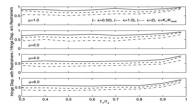
Figure 4.8: Effect of Restrainer Stiffness Ratio on Hinge Displacement Ratio for  $T_2/T_g=4.0$ : Mean for 26 Earthquake Records.
