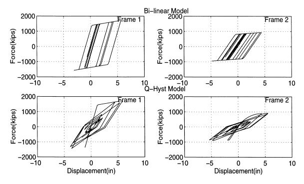
Figure 3.8: Force-Displacement Relationships for Frame Response to the 1940 El Centro Earthquake, Scaled to 0.70g, for Bi-Linear and Q-Hyst Hysteretic Models.
