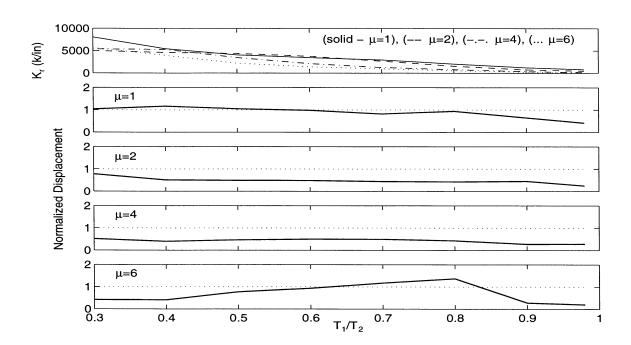
Figure 5.21: Evaluation of Restrainer Design Procedure: 1940 El Centro Earthquake (S00E Component),  $D_r/D_{eq}=0.20$ ,  $T_2/T_g=0.50$ .
