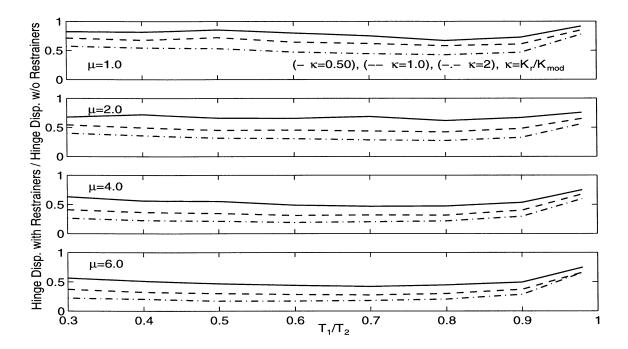
Figure 4.4: Effect of Restrainer Stiffness Ratio on Normalized Hinge Displacement for  $T_2/T_g=1.0$ : Mean for 26 Earthquake Records.
