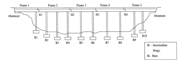
Figure 1.1: Typical Multiple-Frame Bridge.
