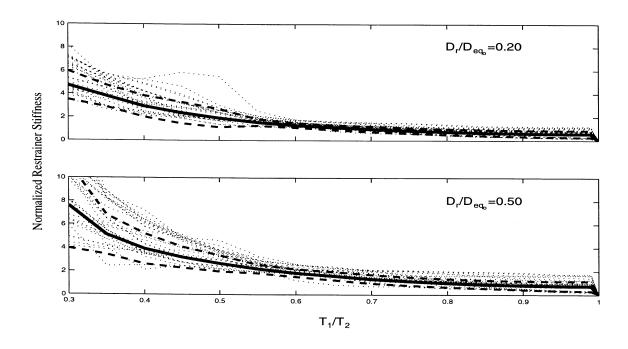
Figure 6.6: Mean  $\pm$  One Standard Deviation of the Normalized Restrainer Stiffness for  $\tilde{T}=6.00.$
