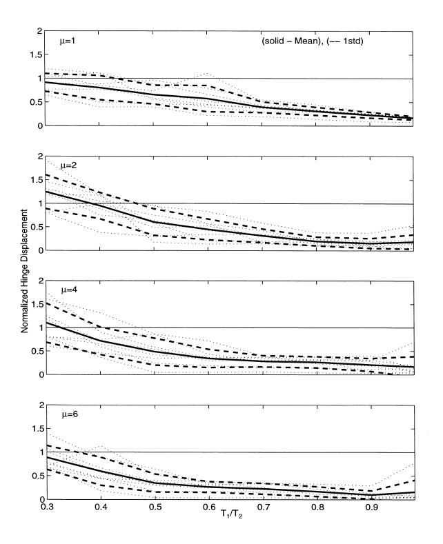
Figure 5.30: Mean  $\pm$  One Standard Deviation of Normalized Hinge Displacement for Restrainers from Design Procedure  $(D_r/D_{eq}=0.50,\,T_2/T_g=4.00)$ .
