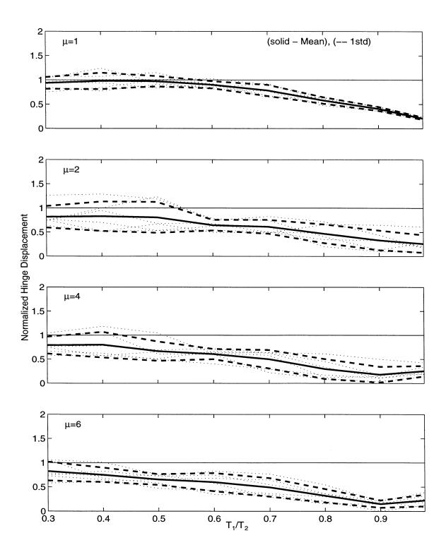
Figure 5.24: Mean  $\pm$  One Standard Deviation of Normalized Hinge Displacement for Restrainers from Design Procedure  $(D_r/D_{eq}=0.50,\,T_2/T_g=0.50)$ .
