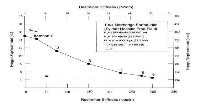
Figure 5.14: Hinge Displacement for Each Iteration of 1994 Northridge Earthquake (Sylmar Hospital Free-Field Record) Design Example.
