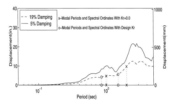
Figure 5.9: Displacement Response Spectrum for 1940 El Centro Earthquake (S00E Component), Showing Spectral Ordinates for First and Last Steps of Example 5.1.
