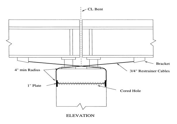
Figure 2.7: Typical Restrainer Configuration for Steel Bridges
