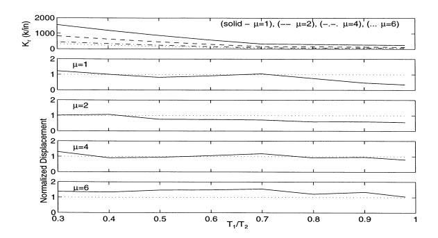
Figure 6.12: Single-Step Restrainer Design Procedure: 1994 Northridge Earthquake (Sylmar Hospital Free-Field Record)  $D_r/D_{eq}$ =0.20,  $T_2/T_g$ =1.0.
