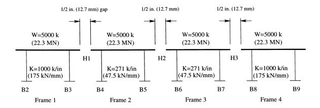
Figure 7.10: Four-Frame Bridge Used for Example Case.
