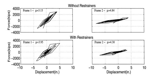
Figure 5.12: Force-Displacement Relationship for Two Frames Subjected to 1940 El Centro Earthquake (S00E Component) Using Restrainers Determined in Example 5.1.
