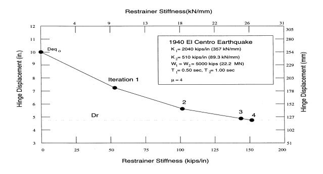
Figure 5.10: Hinge Displacement For Each Iteration of Example 5.1 for 1940 El Centro Earthquake (S00E Component).
