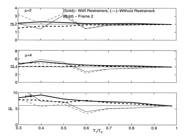
Figure 8.9: Frame Ductility Demands Using Tension and Compression Bounding Models for Frames Subjected to Northridge Earthquake (S00E Component),  $T_2/T_g = 1.0$ .
