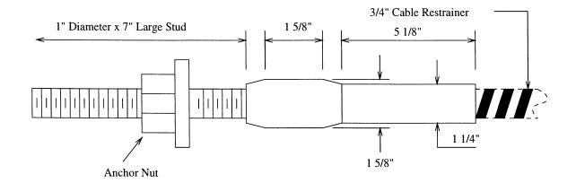
Figure 2.1: Typical Cable Restrainer and Swagged Fitting.
