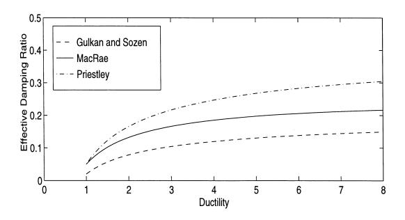
Figure 5.7: Effective Damping Values as a Function of Ductility.
