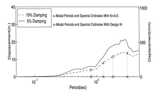
Figure 5.13: Displacement Response Spectrum for 1994 Northridge Earthquake (Sylmar Hospital Free-Field Record) Showing Spectral Ordinates for First and Last Step of Symlar Design Example.
