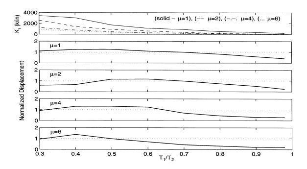
Figure 5.17: Restrainer Design Procedure: 1940 El Centro Earthquake (S00E Component),  $D_r/D_{eq}$ =0.20,  $T_2/T_g$ =1.0.
