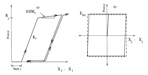
Figure 3.3: Force-Displacement Relationship for (a) Hinge Restrainers (b) Coulomb Friction.
