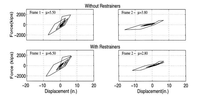
Figure 5.16: Force-Displacement Relationship for Two Frames Subjected to 1994 Northridge Earthquake (Sylmar Hospital Free-Field Record) Using Restrainers Determined from Design Procedure.
