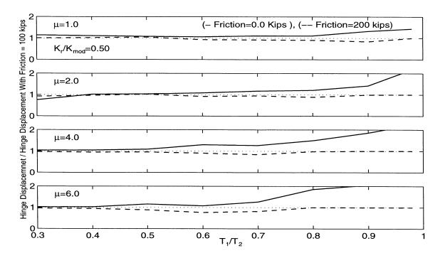
Figure 4.11: Effect of Friction on the Hinge Displacement,  $T_2/T_g = 1.0$  for 1940 El Centro Earthquake (S00E Component).
