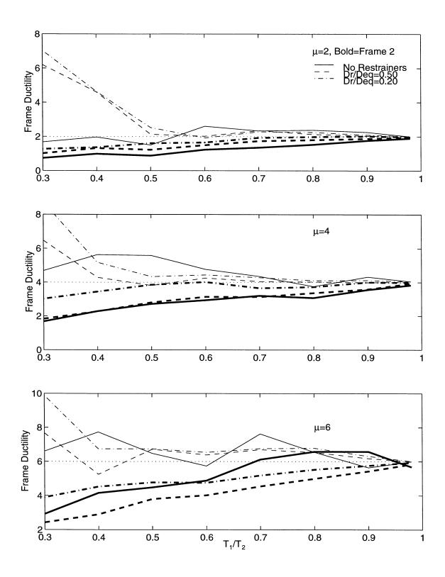
Figure 8.2: Frame Ductilities for Bridge Subjected to 1940 El Centro earthquake (S00E component),  $T_2/T_g=1.0.$
