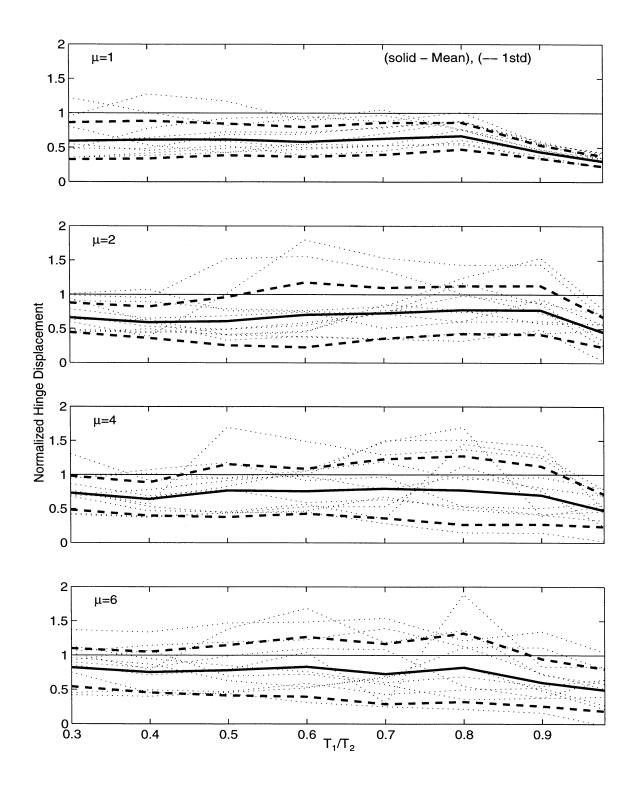
Figure 6.16: Mean  $\pm$  One Standard Deviation of the Normalized Hinge Displacement from Single-Step Design Procedure for  $D_r/D_{eq}$ =0.20,  $T_2/T_g$ =1.0.
