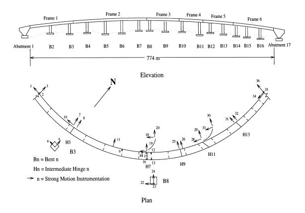
Figure 7.11: General Plan and Strong Motion Instrumentation of the Northwest Connector at the Interstate 10/215 Interchange in Colton, California.
