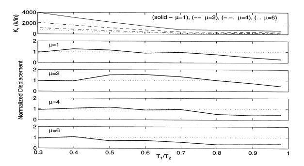
Figure 6.10: Single-Step Restrainer Design Procedure: 1940 El Centro Earthquake (S00E Component)  $D_r/D_{eq}$ =0.20,  $T_2/T_g$ =1.0.
