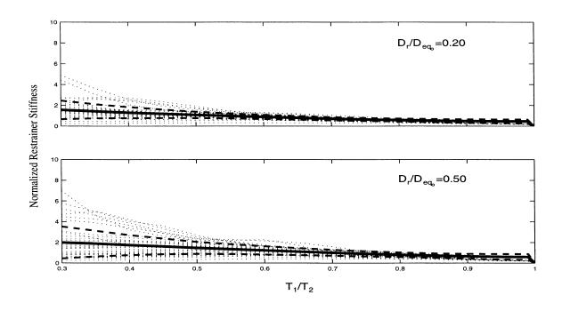
Figure 6.3: Mean  $\pm$  One Standard Deviation of the Normalized Restrainer Stiffness for  $\tilde{T}=1.00.$
