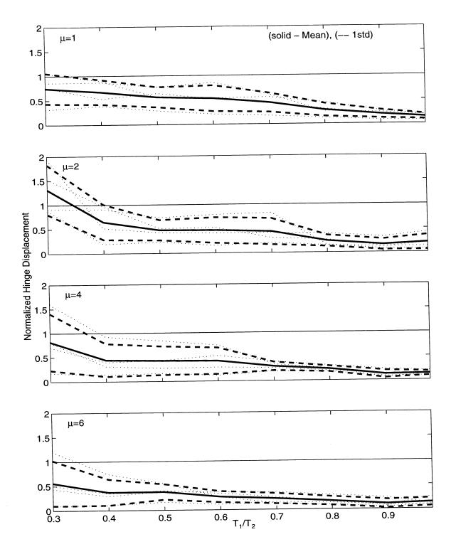
Figure 5.32: Mean  $\pm$  One Standard Deviation of Normalized Hinge Displacement for Restrainers from Design Procedure  $(D_r/D_{eq}=0.50,\,T_2/T_g=6.00)$ .
