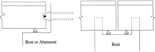
(a) Device to connect a girder and substructure (b) Device to provide a protrudor into a girder or substructure
