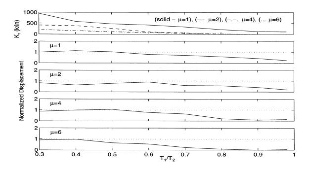
Figure 5.18: Restrainer Design Procedure: 1940 El Centro Earthquake (S00E Component),  $D_r/D_{eq}$ =0.50,  $T_2/T_g$ =1.0.
