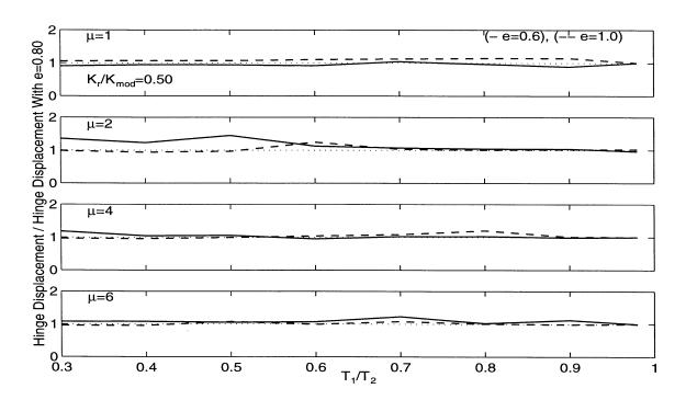
Figure 4.14: Effect of Coefficient of Restitution on the Hinge Displacement,  $T_2/T_g = 1.0$ , 1940 El Centro Earthquake (S00E Component).
