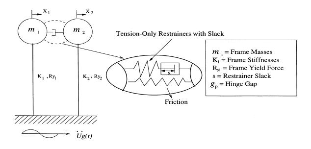
Figure 3.1: Two Degree-of-Freedom Nonlinear Model for Longitudinal Earthquake Response of Two Frames.
