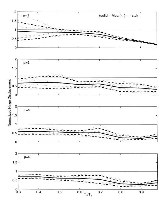
Figure 6.15: Mean  $\pm$  One Standard Deviation of the Normalized Hinge Displacement from Single-Step Design Procedure for  $D_r/D_{eq}$ =0.50,  $T_2/T_g$ =0.5.
