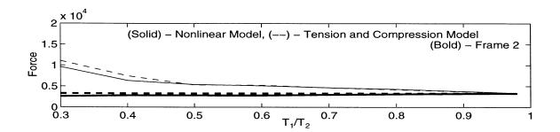
Figure 8.8: Frame Forces from Bounding Models for Frames Subjected to 1994 Northridge Earthquake (Sylmar Hospital Free-Field),  $T_2/T_g = 1.0$ .
