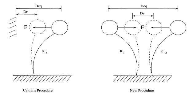
Figure 5.5: Interpretation of the Caltrans and New Procedure For Hinge Restrainers.
