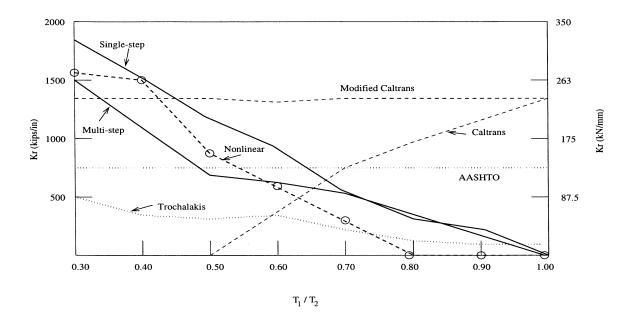
Figure 7.8: Comparison of Required Restrainer Stiffness for 1940 El Centro Earthquake (S00E Component),  $D_r = 4.7$  in. (119 mm),  $\mu = 1$ .
