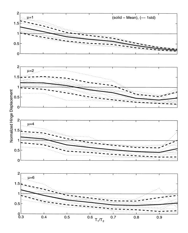
Figure 6.19: Mean  $\pm$  One Standard Deviation of Normalized Hinge Displacement from Single-Step Design Procedure for  $D_r/D_{eq}$ =0.50,  $T_2/T_g$ =2.0.
