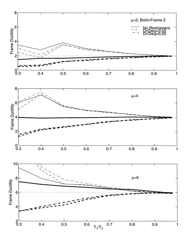
Figure 8.3: Frame Ductilities for Bridge Subjected to 1994 Northridge Earthquake (Sylmar Hospital Free-Field Record),  $T_2/T_g=1.0$ .
