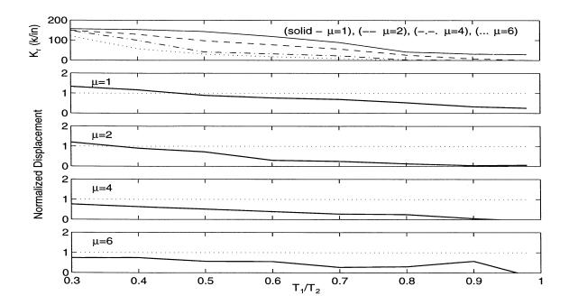
Figure 5.22: Evaluation of Restrainer Design Procedure: 1940 El Centro Earthquake (S00E Component),  $D_r/D_{eq}=0.20,\,T_2/T_g=2.00.$
