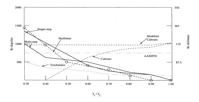
Figure 7.9: Comparison of Restrainer Stiffness for 1994 Northridge Earthquake (Sylmar Hospital Free-Field Record),  $D_r = 4.7$  in. (119 mm),  $\mu = 1$ .
