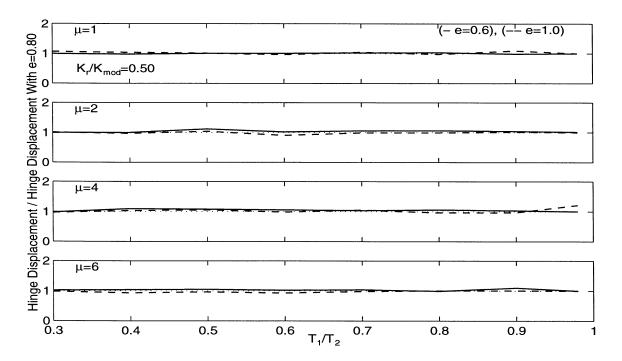
Figure 4.15: Effect of Coefficient of Restitution on Hinge Displacement,  $T_2/T_g = 1.0$ , 1994 Northridge Earthquake (Sylmar Hospital Free-Field Record).
