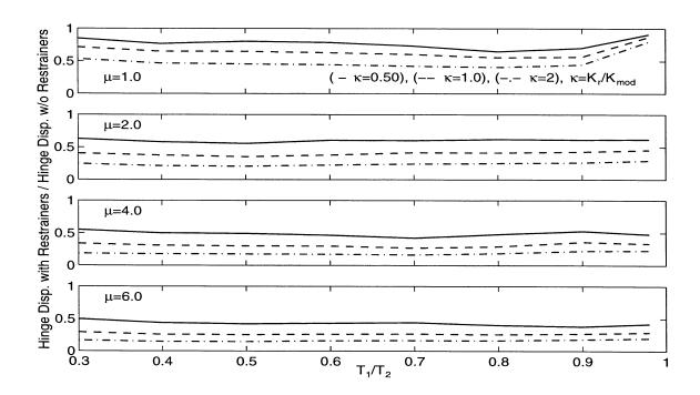
Figure 4.18: Effect of Restrainer Stiffness Ratio on Hinge Displacement for  $m_1/m_2 = 2.0$ , Mean for 26 Earthquake Records.
