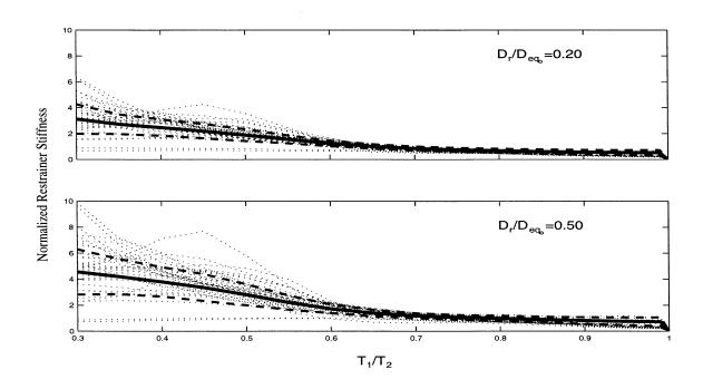
Figure 6.4: Mean  $\pm$  One Standard Deviation of the Normalized Restrainer Stiffness for  $\tilde{T}=1.50.$
