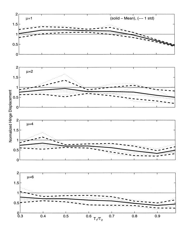
Figure 5.23: Mean  $\pm$  One Standard Deviation of Normalized Hinge Displacement for Restrainers from Design Procedure  $(D_r/D_{eq}=0.20,\,T_2/T_g=0.50)$ .
