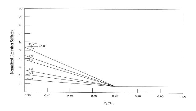
Figure 6.7: Bilinear Curve-Fit for Normalized Restrainer Stiffness for  $D_r/D_{eq_o}=0.20$ .
