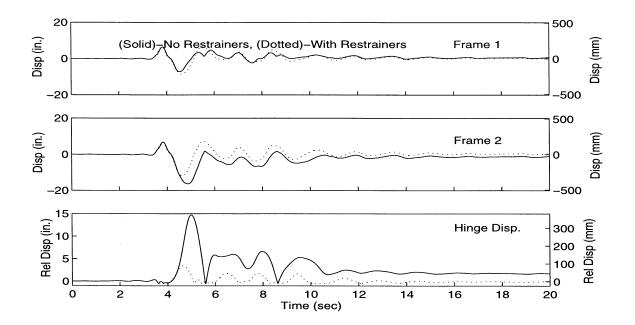
Figure 5.15: Response History for Two Frames Subjected to 1994 Northridge Earthquake (Sylmar Hospital Free-Field Record) Using Restrainers Determined from Design Procedure.
