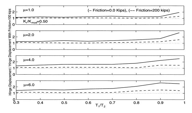
Figure 4.13: Effect of Friction on the Relative Hinge Displacement,  $T_2/T_g=1.0$ , Mean Plus One Standard Deviation for 26 Earthquakes.
