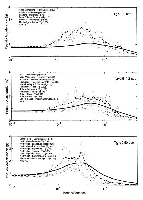
Figure 4.1: Mean Plus One Standard Deviation (- - - ) of the Pseudo-Acceleration Spectra (5% Damping) for 26 Ground Motions Compared With Caltrans ARS Spectra (---).
