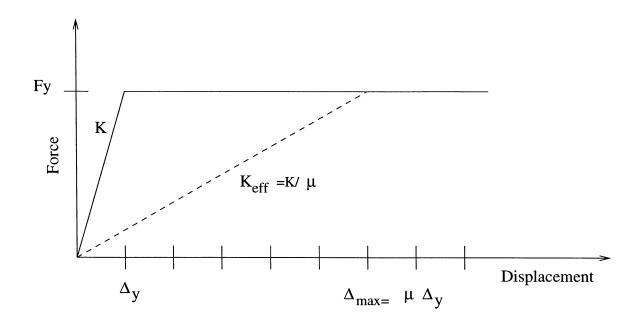
Figure 5.6: Effective Stiffness Values as a Function of Ductility.
