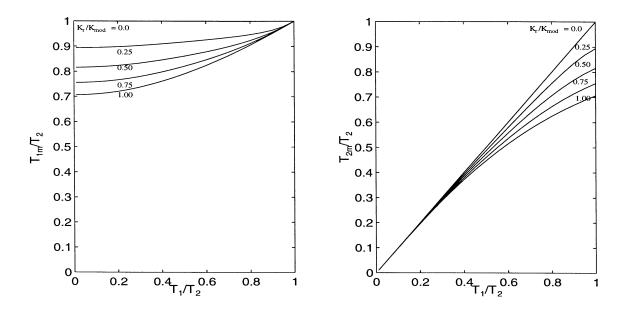
Figure 5.3: Normalized Modal Periods as a Function of Frame Period Ratio and Restrainer Stiffness Ratio.
