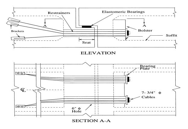
Figure 2.4: Modern Hinge Restrainer Retrofit Scheme: Type 1 Restrainer Unit.
