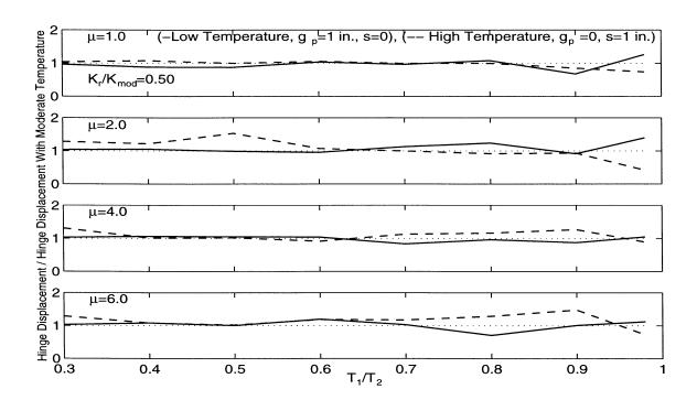
Figure 4.9: Effect of Hinge Gap and Restrainer Slack on Hinge Displacement Ratio for 1940 El Centro Earthquake (S00E Component):  $T_2/T_g = 1.0$ .
