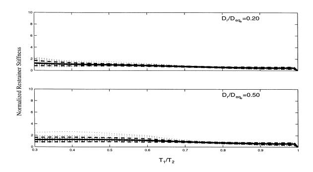
Figure 6.1: Mean  $\pm$  One Standard Deviation of the Normalized Restrainer Stiffness for  $\tilde{T}=0.25.$
