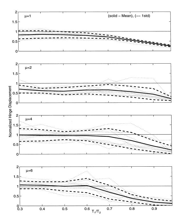
Figure 5.26: Mean  $\pm$  One Standard Deviation of Normalized Hinge Displacement for Restrainers from Design Procedure  $(D_r/D_{eq}=0.50,\,T_2/T_g=1.00)$ .
