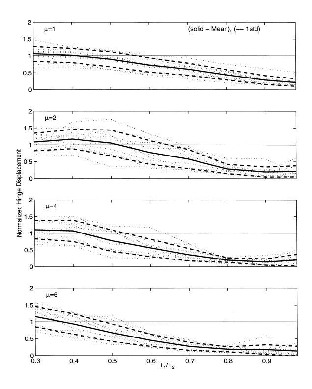
Figure 5.28: Mean  $\pm$  One Standard Deviation of Normalized Hinge Displacement for Restrainers from Design Procedure  $(D_r/D_{eq}=0.50,\,T_2/T_g=2.00)$ .
