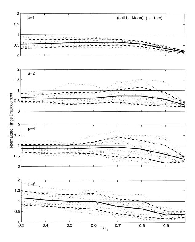
Figure 6.17: Mean  $\pm$  One Standard Deviation of the Normalized Hinge Displacement from Single-Step Design Procedure for  $D_r/D_{eq}$ =0.50,  $T_2/T_g$ =1.0.
