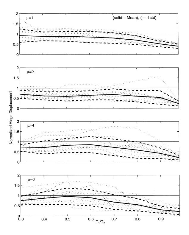
Figure 5.25: Mean  $\pm$  One Standard Deviation of Normalized Hinge Displacement for Restrainers from Design Procedure  $(D_r/D_{eq}=0.20,\,T_2/T_g=1.00)$ .
