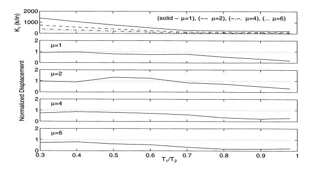
Figure 6.11: Single-Step Restrainer Design Procedure: El Centro Earthquake (S00E Component)  $D_r/D_{eq}$ =0.50,  $T_2/T_g$ =1.0.
