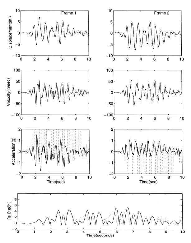
Figure 3.5: Comparison of Numerical Procedure with DRAIN3-DX for Elastic Frame Response to 1940 El Centro Earthquake (S00E Component), scaled to 0.70g (..... DRAIN3-DX), (—— Numerical Procedure).
