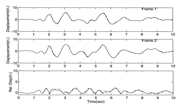
Figure 3.9: Frame Response to 1940 El Centro Earthquake, Scaled to 0.70g, for Different Values of the Coefficient of Restitution (——- e = 1.0), (- - - - e = 0.80), (……. e = 0.60).
