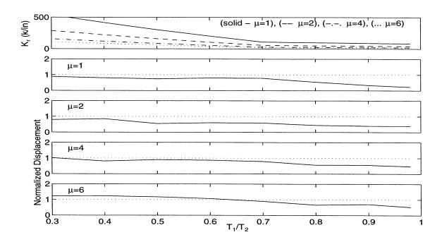
Figure 6.13: Single-Step Restrainer Design Procedure: 1994 Northridge Earthquake (Sylmar Hospital Free-Field Record)  $D_r/D_{eq}=0.50, T_2/T_q=1.0$ .
