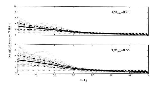
Figure 6.5: Mean  $\pm$  One Standard Deviation of the Normalized Restrainer Stiffness for  $\tilde{T}=3.00$ .
